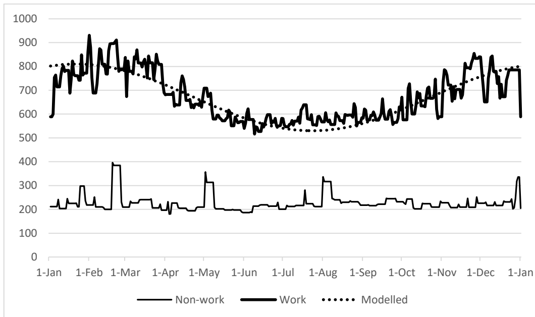
Figure 10. Actual energy consumption through largest site meter
