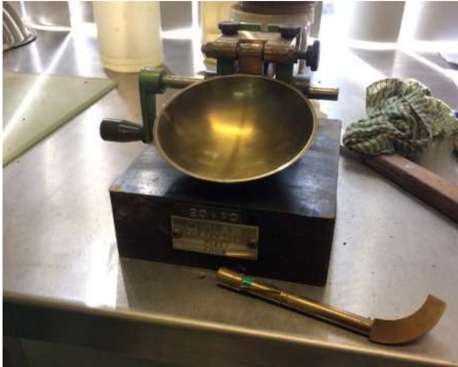
Figure 2.5: drop pan device with grooving tool in bottom right of picture
