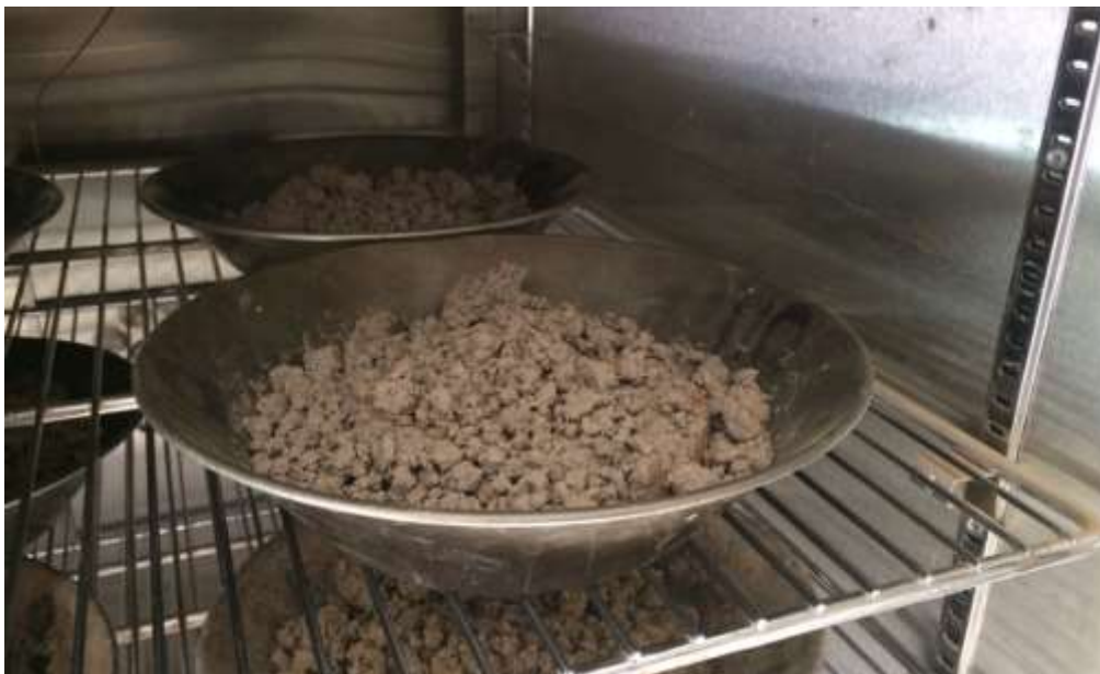
Figure 4.7: Moisture content sample being dried back in the soil oven.
