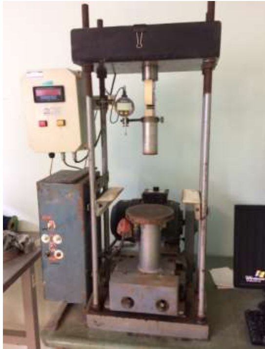
Figure 2.6: CBR testing apparatus
