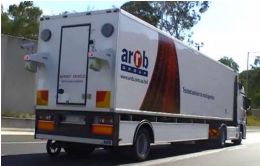
Figure 4.9: ARRB Groups TSD truck which was used to collect TSD data
