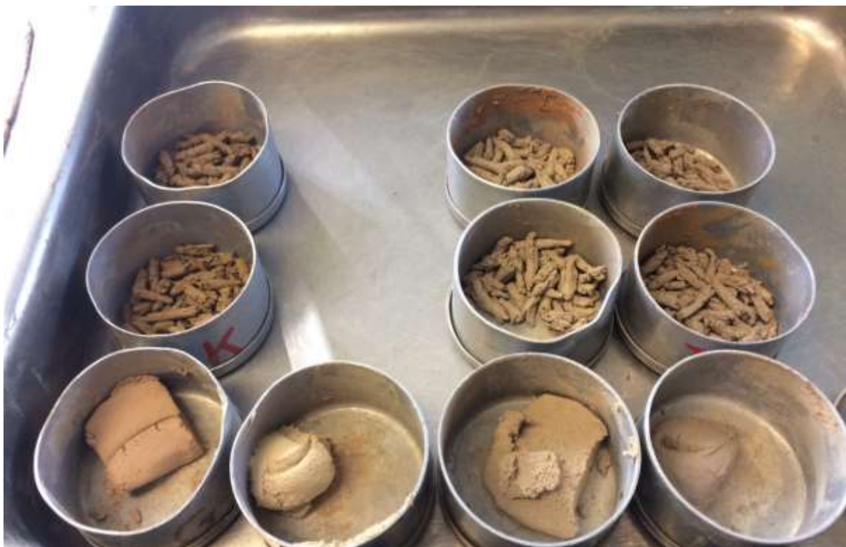
Figure 4.8: Moisture contents sample from Atterberg tests after being oven dried
