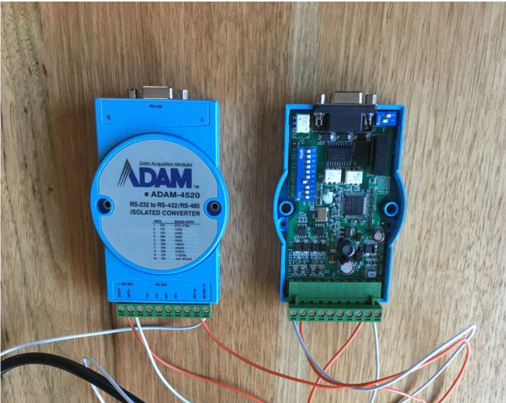
Figure 3.10: Adam-4520 RS-232 to RS-485 converter
