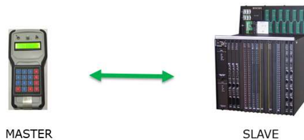
Figure 6.2: Arduino Modbus Simulator Master to Triconex Slave
