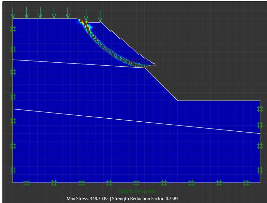
Figure 3.13: Results of slope stability analysis showing fifty percent deformation and the plastic multiplier (Optum Computational Engineering 2016).
