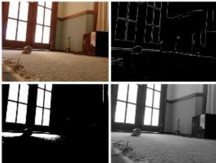
Figure 4-1: A visual comparison of the various image formats considered within Experiment 1 (from top-left clockwise these formats are Colour, Edge, Greyscale and Black and White respectively).
