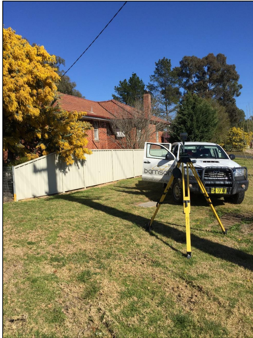
Figure 3-7: Photograph showing R10 rover set up
