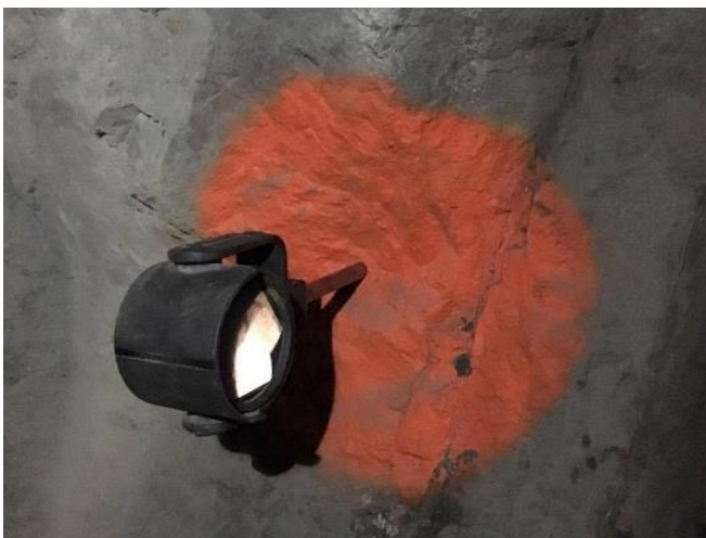
Figure 3-2 Wall Station Prism placed into Sleeve
