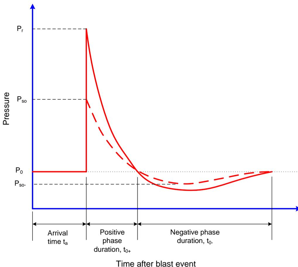
Figure 2-6. Pressure time history of free field blast and reflected blast
