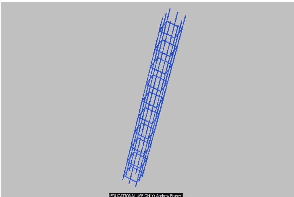
Figure 3-46. Reinforced Concrete Column Reinforcement Detailing
