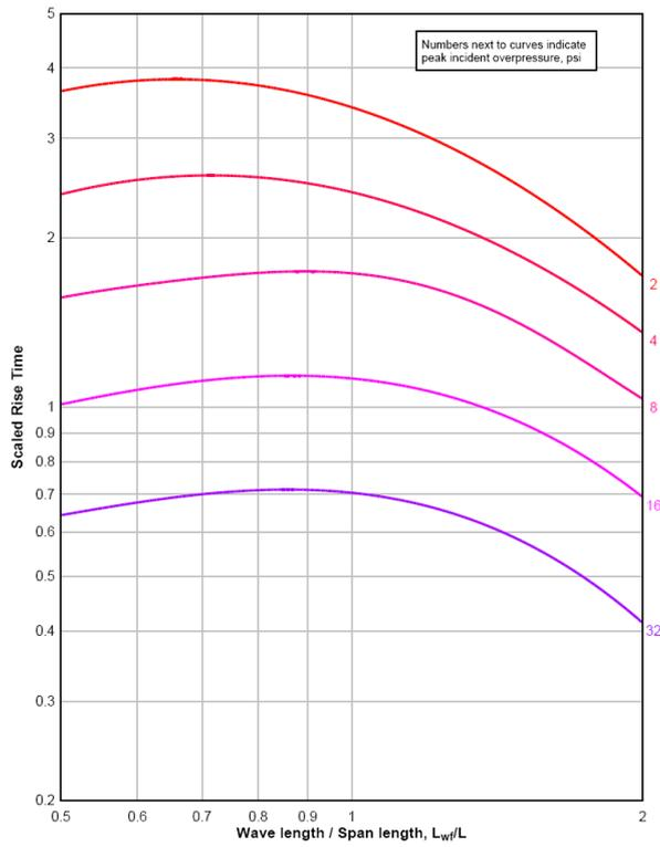
Figure 3-14. Scaled Rise Time of Equivalent Uniform Positive Roof Pressures
