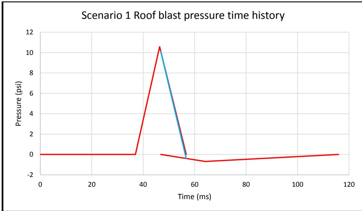
Figure 3-20. Scenario 1 Blast pressure time history for Roof
