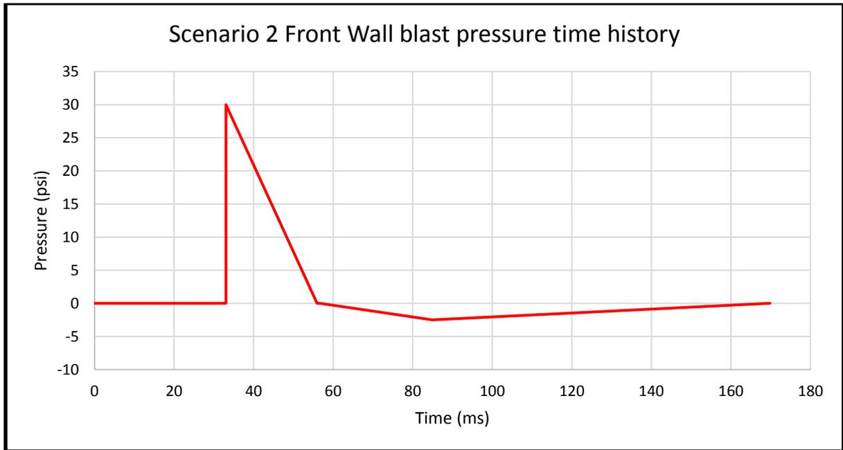
Figure 3-10. Scenario 2 Blast pressure time history at front wall
