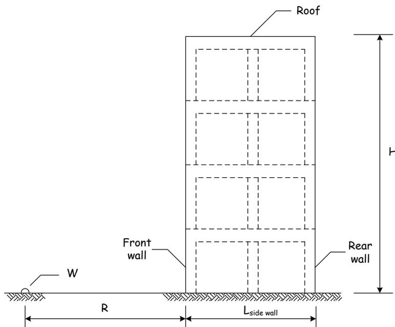
Figure 3-1. Model Structure Subjected to Blast Action (elevation)
