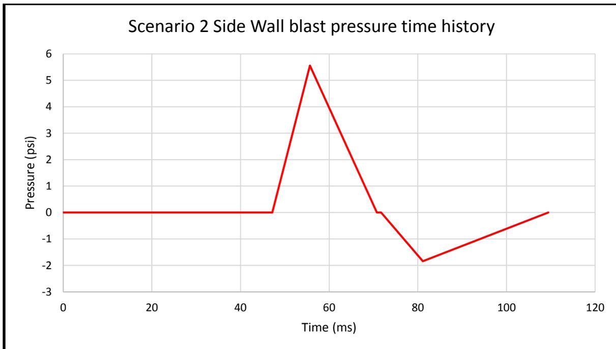
Figure 3-18. Scenario 2 Blast pressure time history at side wall
