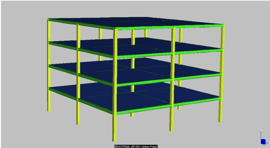
Figure 3-28. Reinforced Concrete Framed Building FE Structural Model
