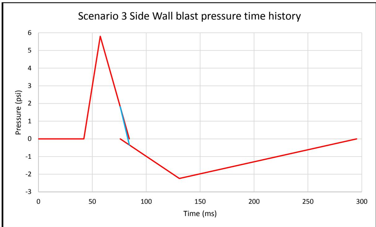
Figure 3-19. Scenario 3 Blast pressure time history at side wall
