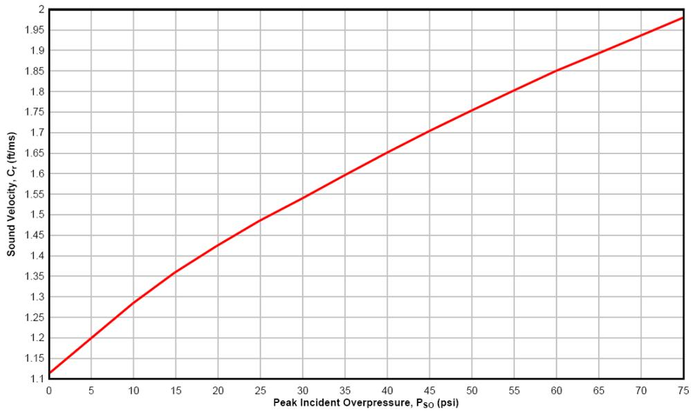
Figure 3-5. Velocity of Sound in Reflected Overpressure Region vs Peak Incident Overpressure
