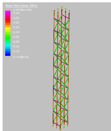
Time step 2ms (steel shear lacing reinforcement elements)
