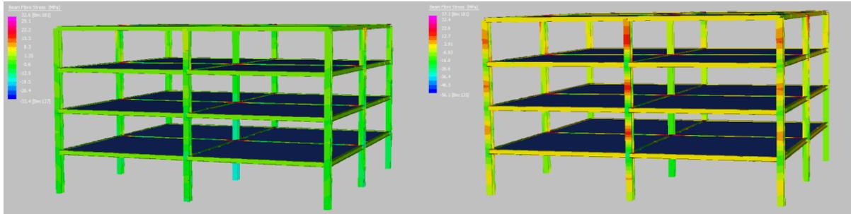
Time step 12ms (arrival of front wall blast pressure)
