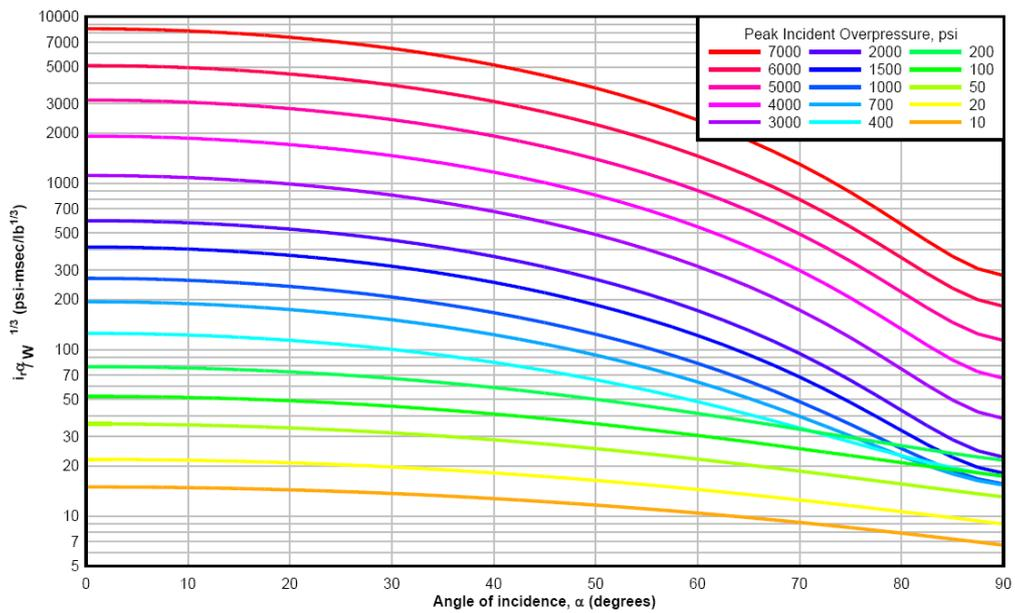
Figure 3-4. Reflected Scaled Impulse versus Angle of Incidence
