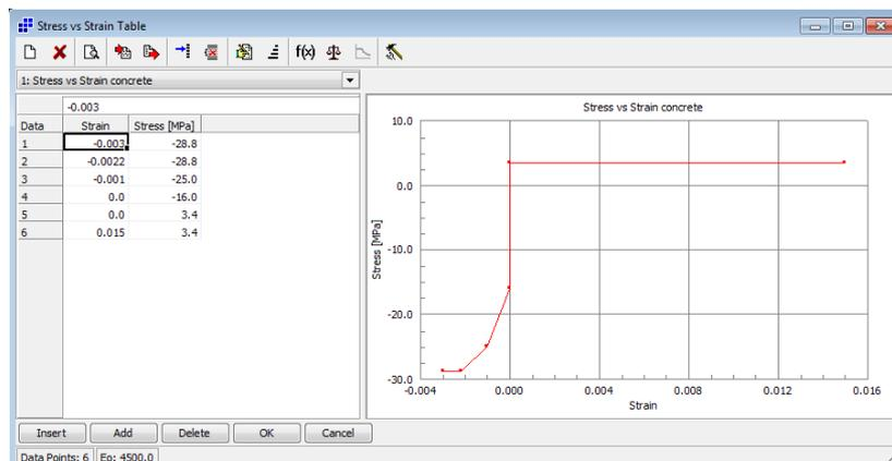
Figure 3-41. Concrete stress vs strain curve
