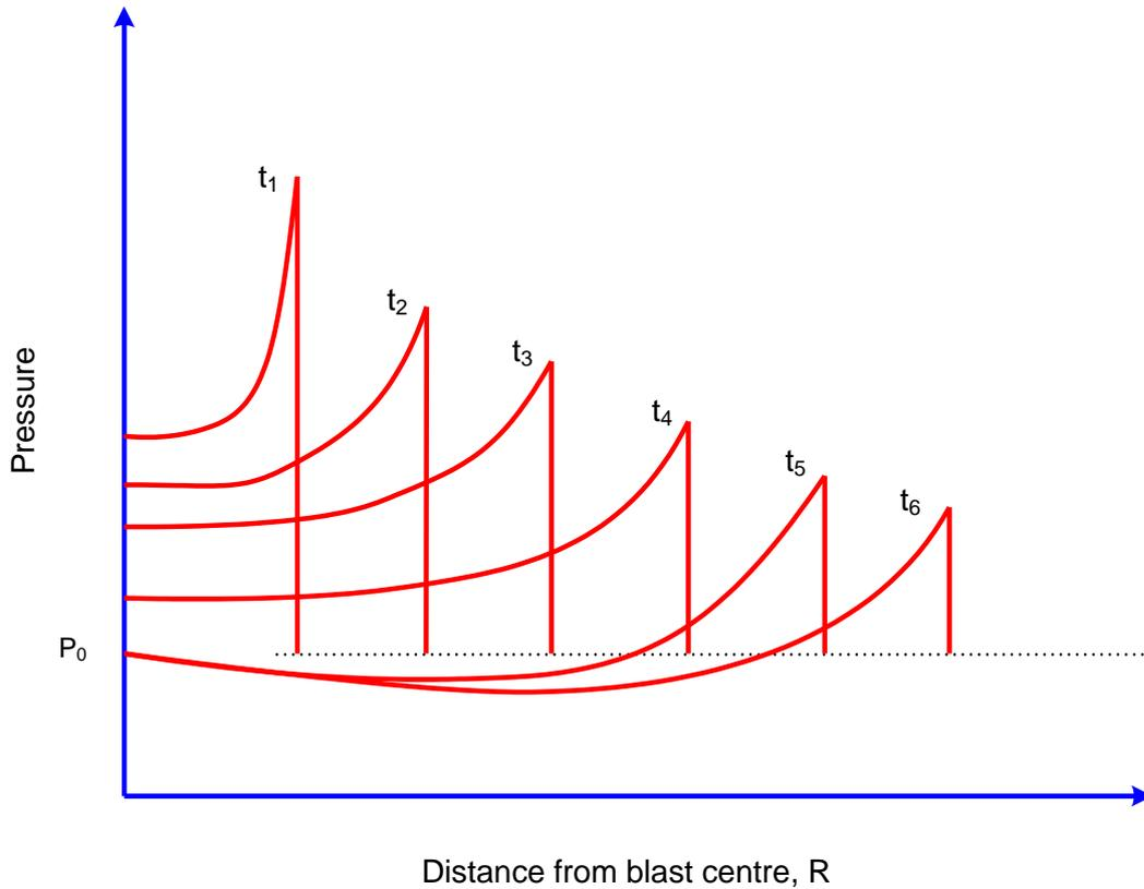
Figure 2-3. Incident overpressure ( $P_s$ ) variation with the distance ( $R$ ) from the charge centre (Source: Ngo et al. 2007)
