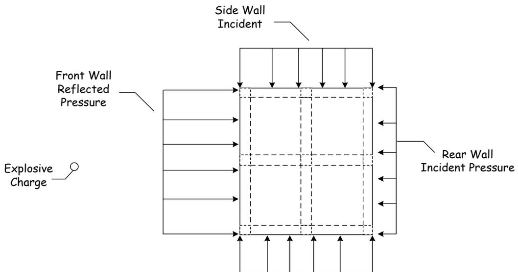
Figure 3-27. Plan Diagram of Typical Structural Model Peak Blast Loading Interaction
