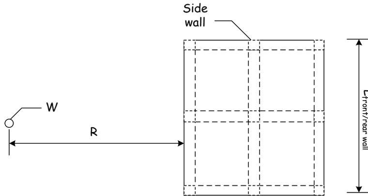
Figure 3-2. Model Structure Subjected to Blast Action (plan)
