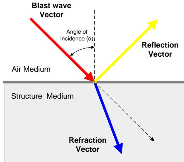
Figure 2-8. Refraction and reflection of blast waves interacting with two mediums
