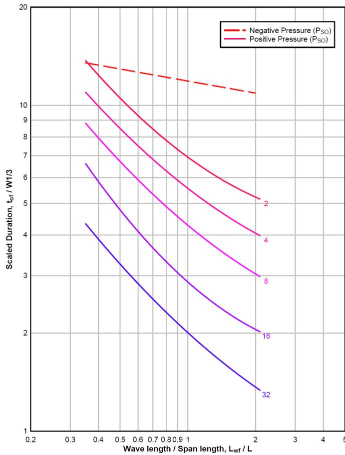
Figure 3-15. Scaled Duration of Equivalent Uniform Roof Pressures
