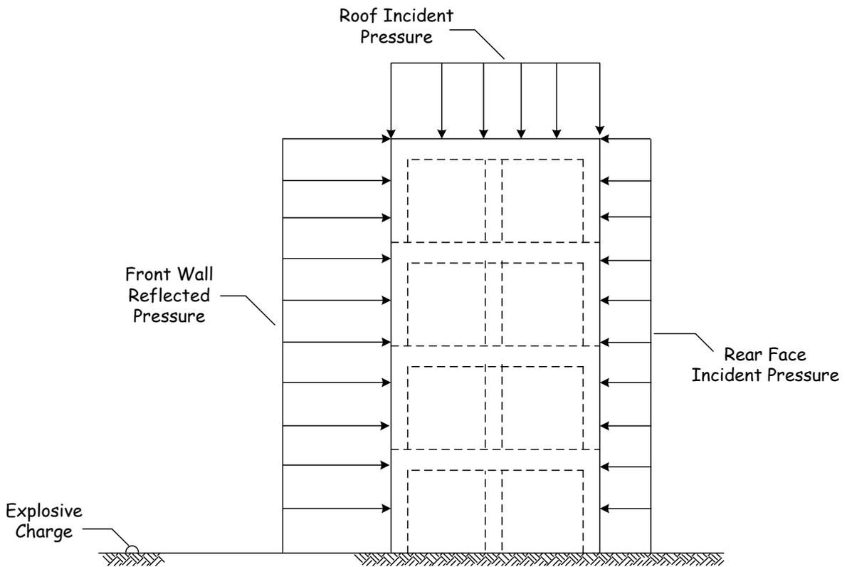
Figure 3-26. Elevation Diagram of Typical Structural Model Peak Blast Loading Interaction
