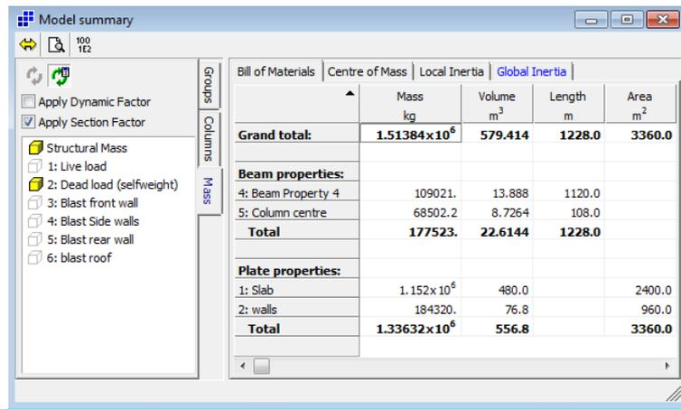
Figure 3-39. Structural mass applied as dead load
