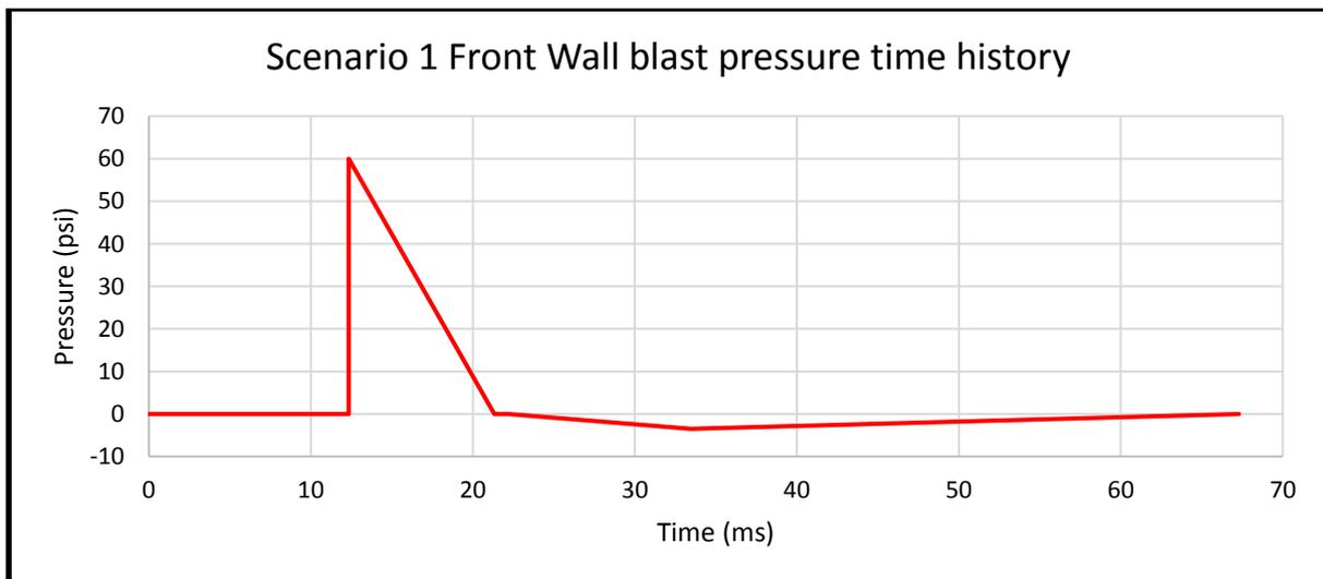
Figure 3-8. Scenario 1 Blast pressure time history at front wall
