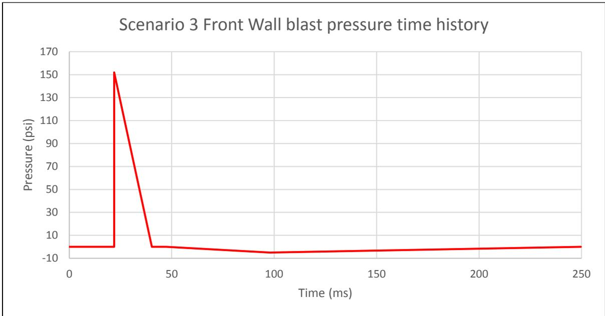
Figure 3-11. Scenario 3 Blast pressure time history at front wall
