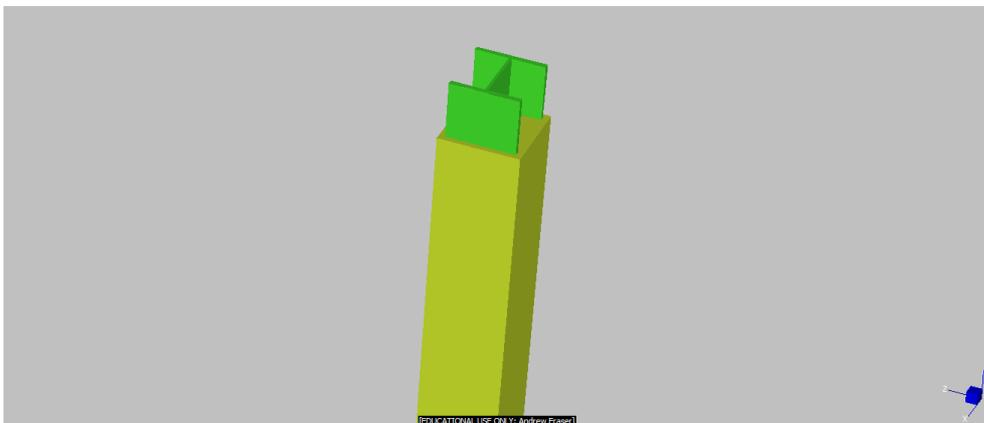
Figure 3-51. Universal Steel Column Encased in Concrete
