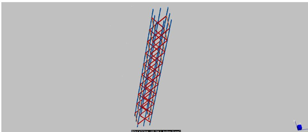
Figure 3-48. Reinforcement Lacing Detailing
