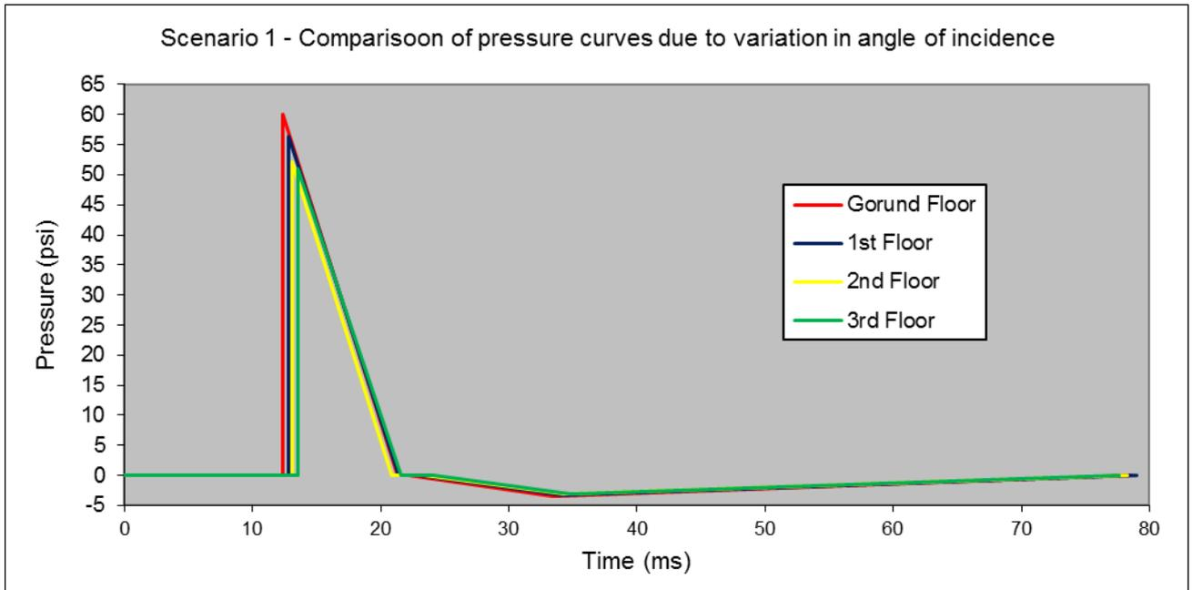
Figure 3-9. Scenario 1 Comparison of Pressure Time Histories Due to the Variation in Incidence Angle
