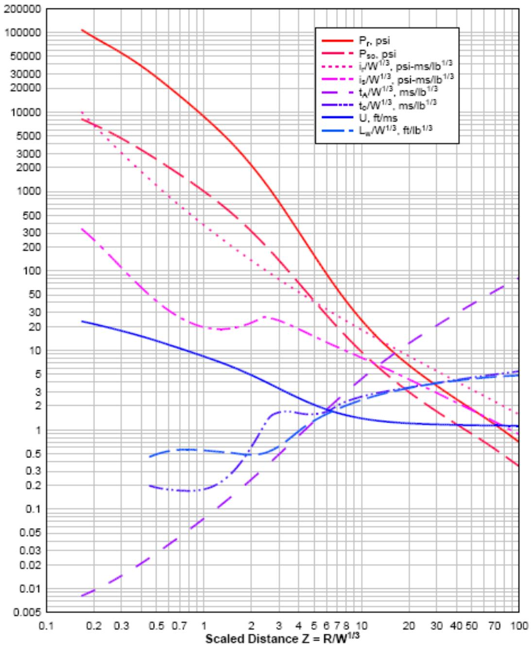
Figure 2-11. Blast Parameters for TNT Surface Bursts (Department of Defense, 2014)
