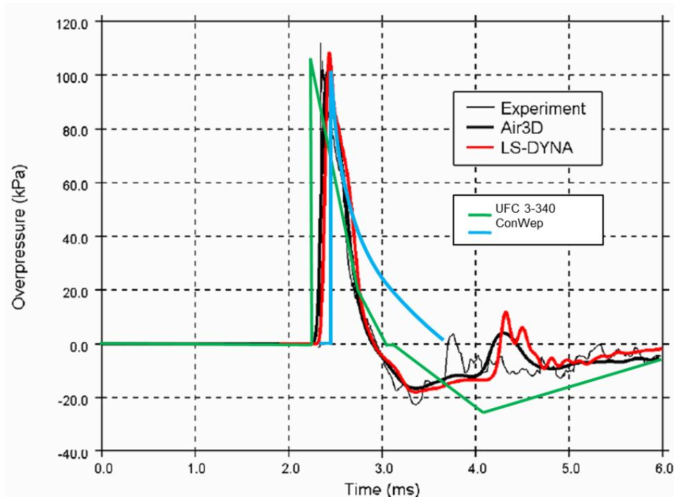
Figure 2-12. Comparison of Blast Pressure Time History Prediction Methods
