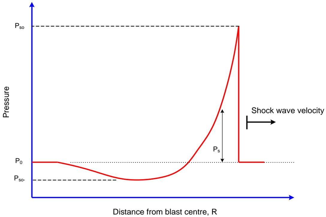
Figure 2-2. Variation of incident overpressure at a distance from blast centre at a given time (Cormine, Mays, & Smith, 2009)
