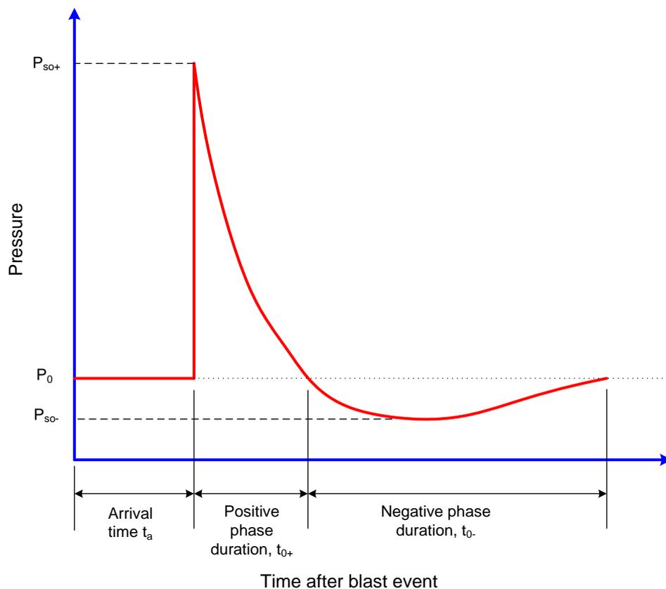
Figure 2-4. Shock wave pressure time history from blast Detonation (adapted from Dusenberry, 2010 Pg 164)
