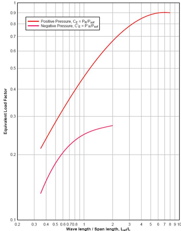
Figure 3-13. Peak Equivalent Uniform Roof Pressures
