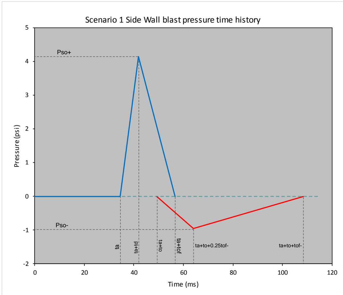
Figure 3-16. Scenario 1 Blast Pressure Time History at Side Wall
