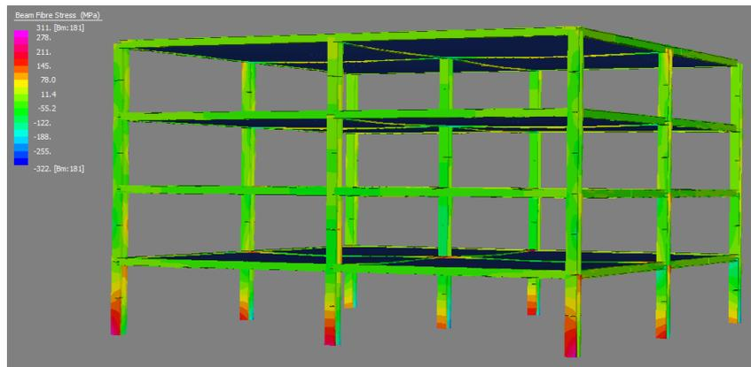
Time step 40ms end of front wall positive phase duration
