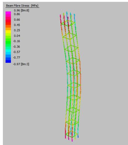
Time step 5ms (steel reinforcement elements)
