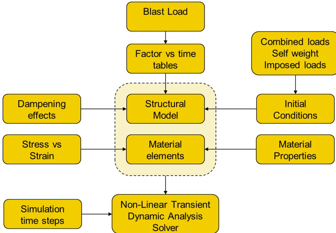
Figure 3-35. Strand7 FEA Non Linear Transient Dynamic Analysis Approach
