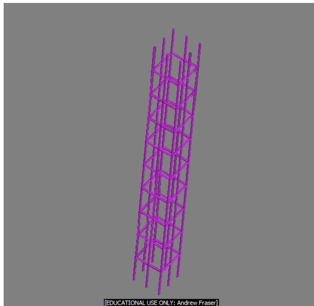
Figure 3-30. RC Column Reinforcement Detailing
