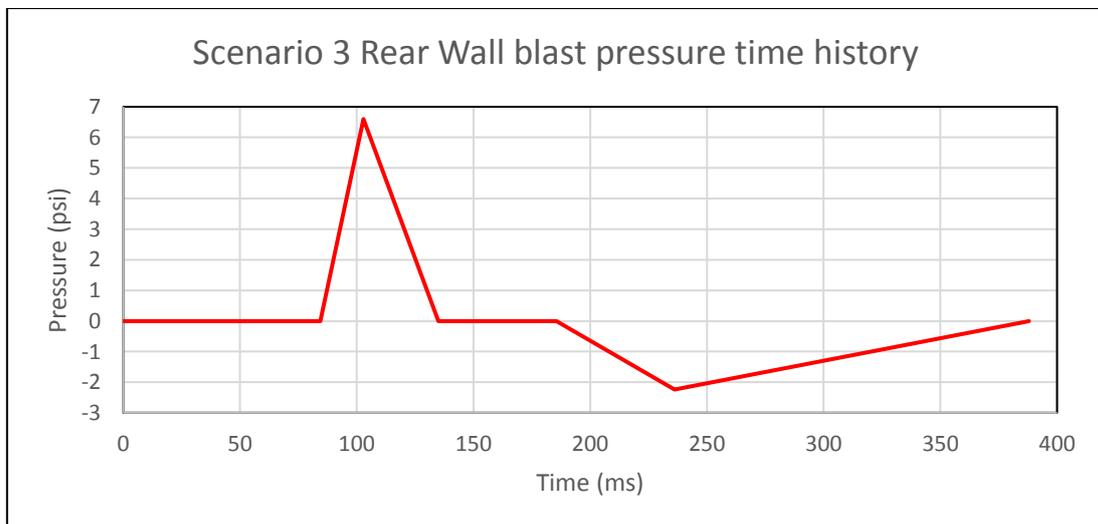
Figure 3-25. Scenario 3 Blast pressure time history of Rear Wall
