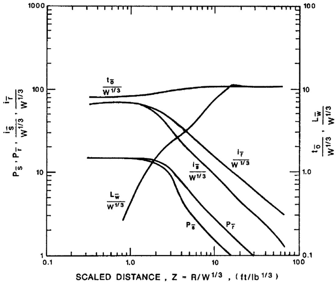
Figure 3-12. Negative Phase Shock Wave Parameters for a Spherical TNT Explosion in Free Air at Sea Level
