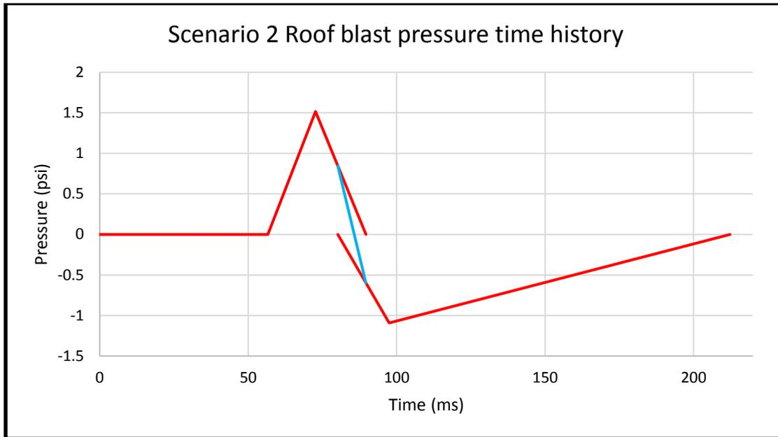
Figure 3-21. Scenario 2 Blast pressure time history for Roof
