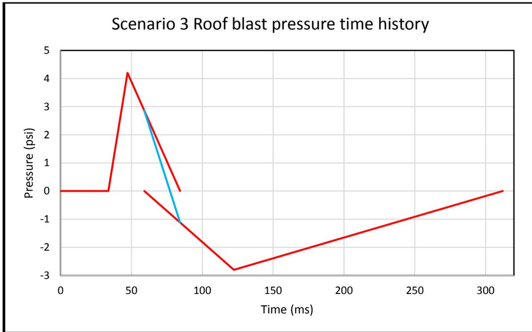
Figure 3-22. Scenario 3 Blast pressure time history for Roof
