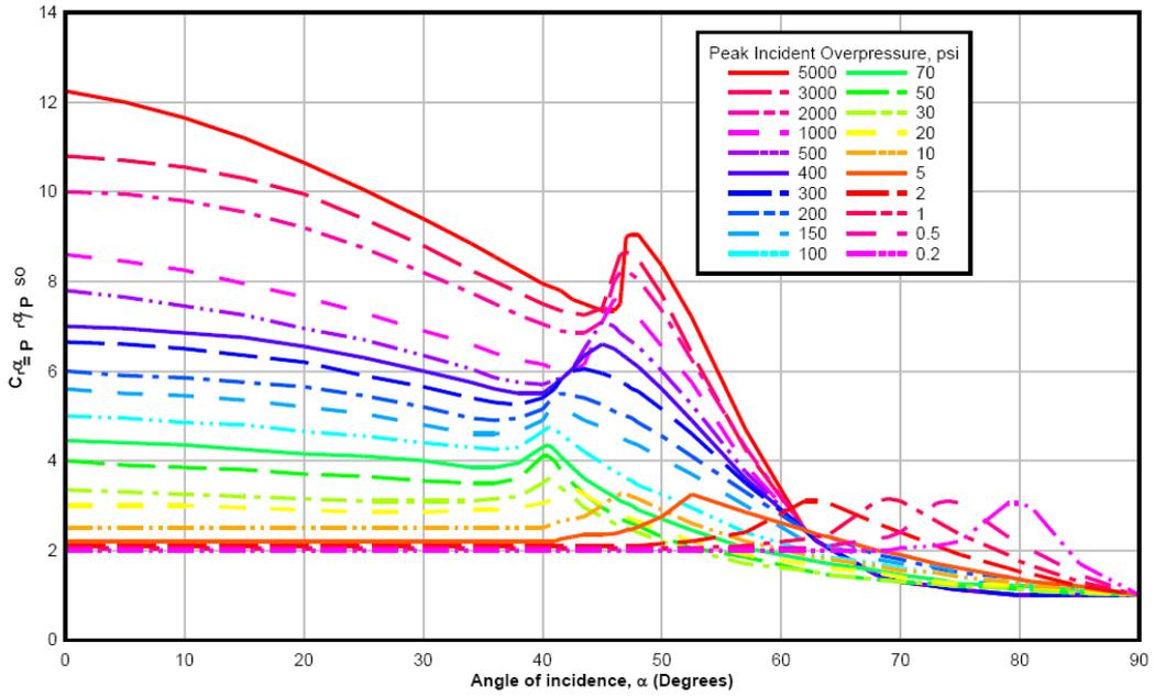
Figure 3-3. Reflected Pressure Coefficient versus Angle of Incidence
