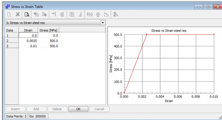
Figure 3-42. Steel stress vs strain curve
