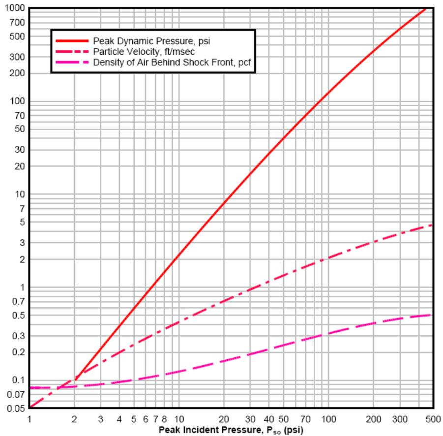
Figure 3-6. Peak Incident Pressure vs Peak Dynamic Pressure, Density of Air Behind the Shock Front, and Particle Velocity
