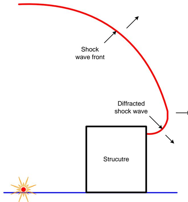
Figure 2-7. Blast wave diffraction
