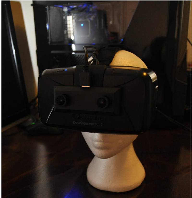
Figure 16: OVRVision Pro mounted on the DK2.0
