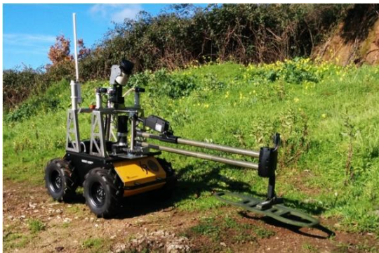
Figure 1: The FSR Husky demining robot
