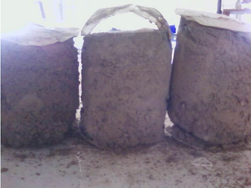
Figure 53: Columns of Treatment 2. From left to right: 2A, 2B, 2C. These columns have fertiliser but no biochar applied.
