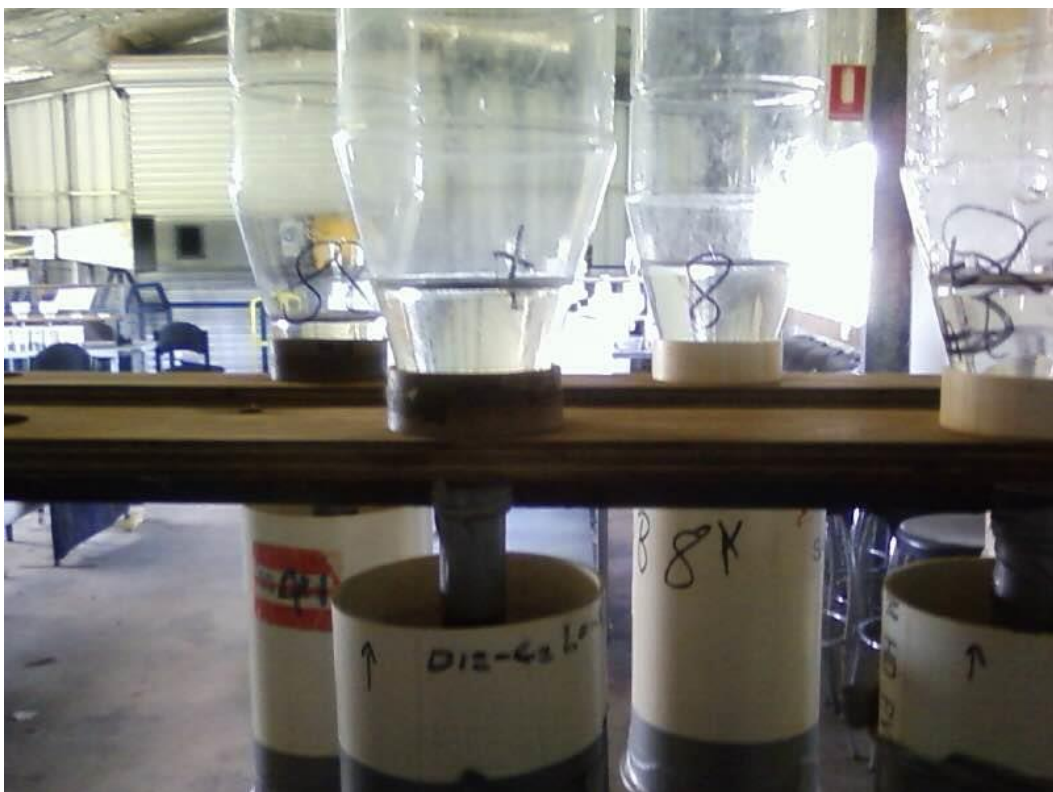
Figure 64: A close up of the working experiment. The lengths of poly pipe extend from the bottles to control the depth of ponded head.
