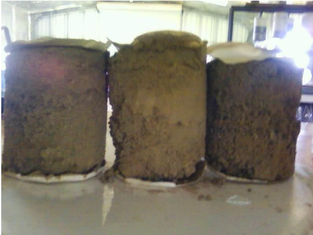
Figure 52: Columns of Treatment 1. From left to right: 1A, 1B, 1C. These columns have biochar but no fertiliser applied.
