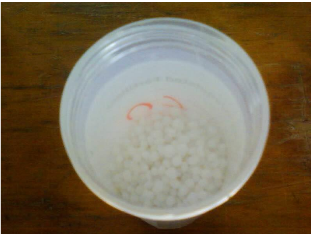
Figure 62: The granulised urea fertiliser. This was dissolved in the water applied during the first rainfall event.
