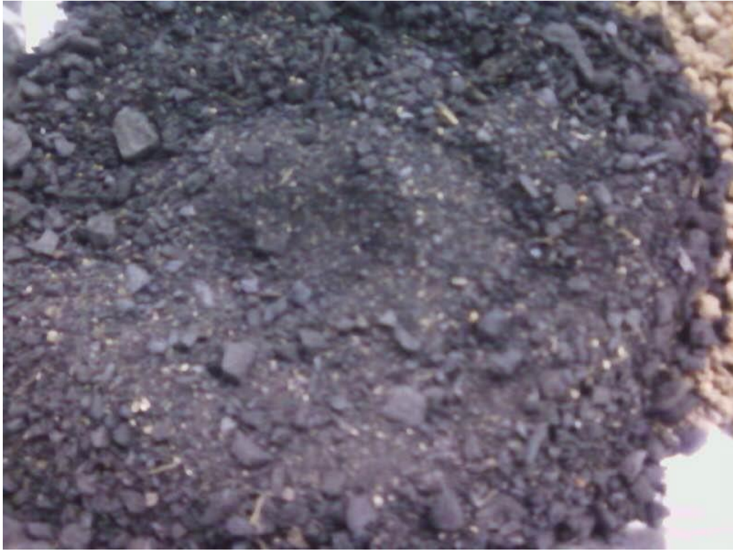
Figure 60: Up-close image of the biochar used. The lighter coloured pieces appear to be uncooked plant material.
