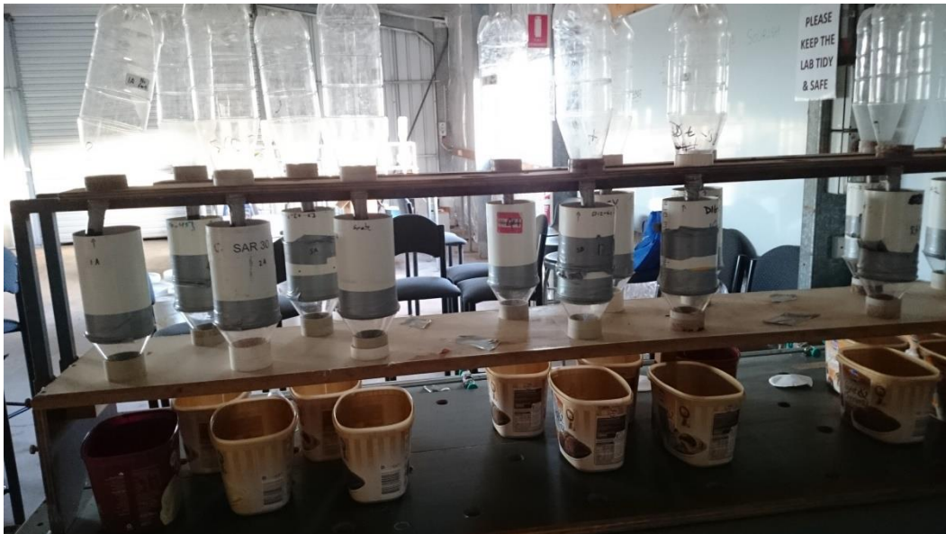
Figure 4: Column Testing Set-up, note the use of common household materials is extremely unlikely to compromise accuracy.
