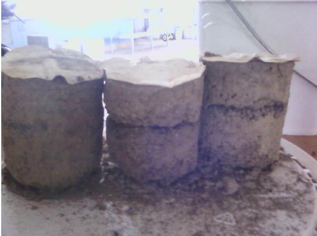
Figure 56: Columns of Treatment 5. From left to right: 5A, 5B, 5C. These columns have fertiliser and layered biochar applied.
