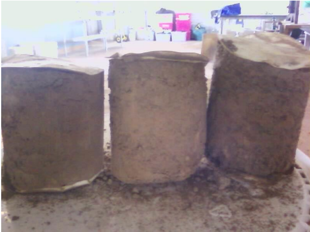
Figure 54: Columns of Treatment 3. From left to right: 3A, 3B, 3C. These columns have no fertiliser or biochar applied.
