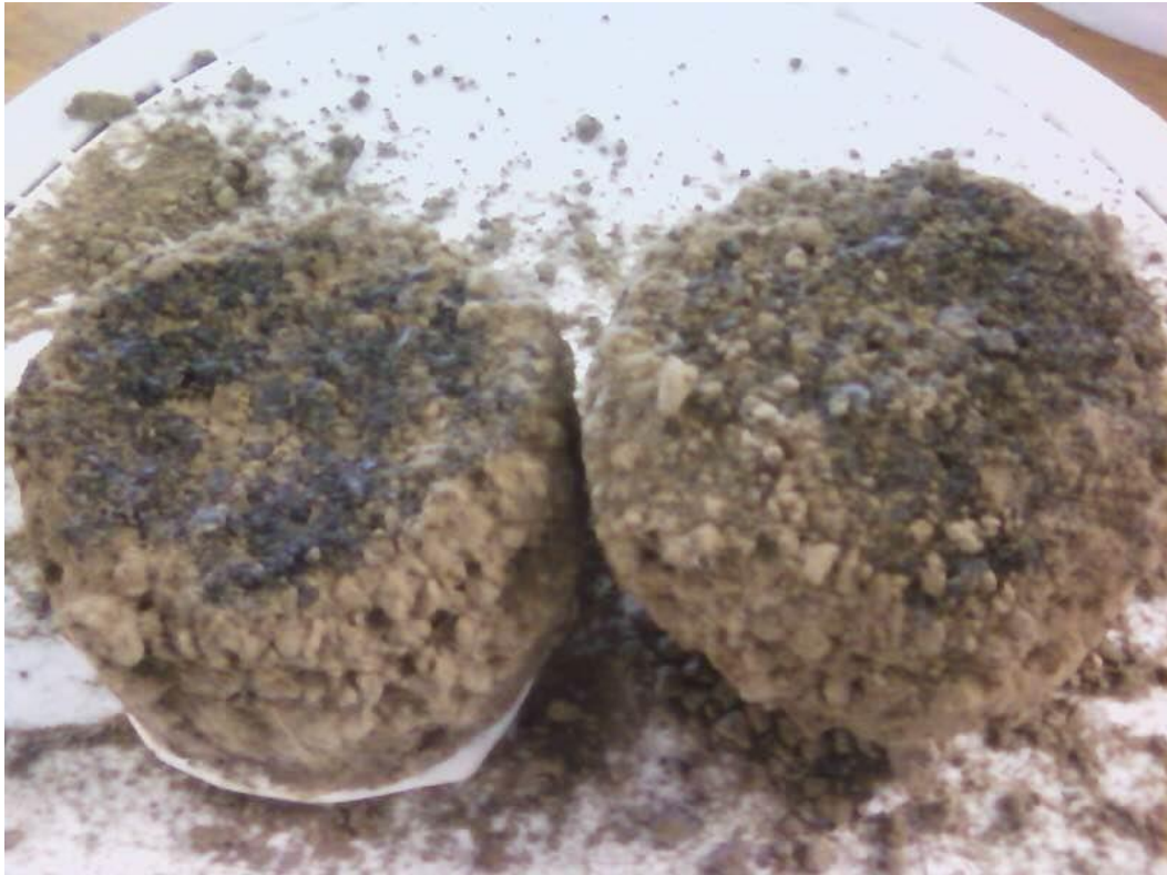
Figure 57: View of the two broken halves of 5B. As expected the biochar layer created a point of structural failure.
