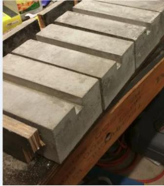
**Figure 3-5 Prisms Stripped ready for final notch detailing.**
