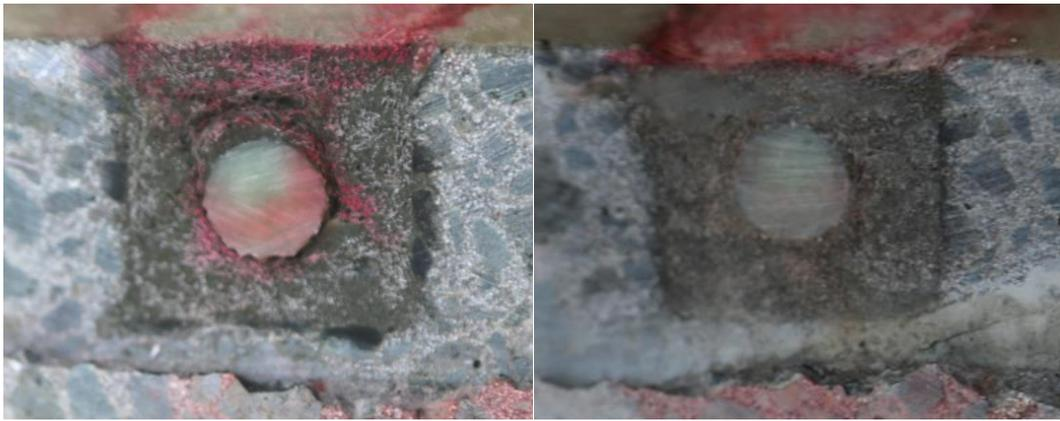
**Figure 4-11 Dye Penetration - ECC2-4 (Left) ECC2-2 (Right)**
