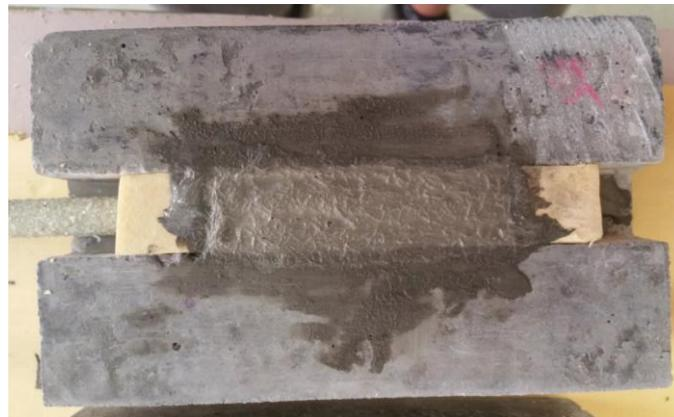
**Figure 3-8 Completed Specimen shortly after ECC pour.**
