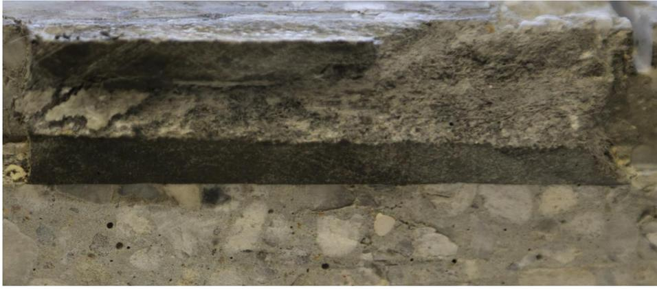
**Figure 4-5 Cross Section of ECC1 sample showing dense adhesive and no apparent air voids.**
