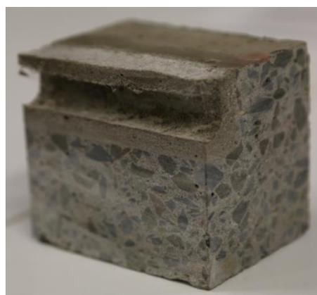
**Figure 4-20 Sample ECC3-1 Section View**
