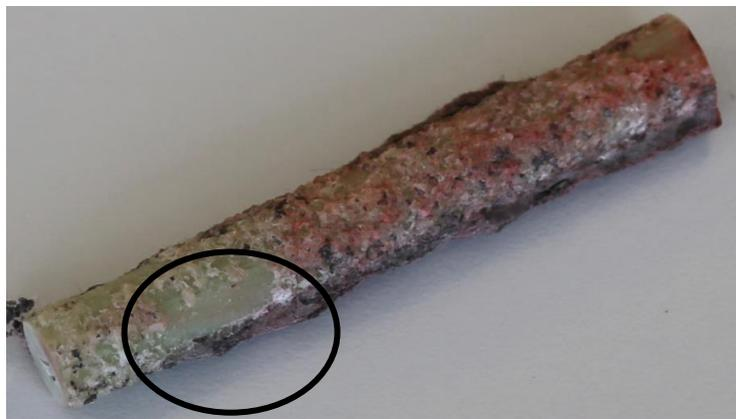
**Figure 4-4 ECC1 FRP bar showing sand coating de-bonding**
