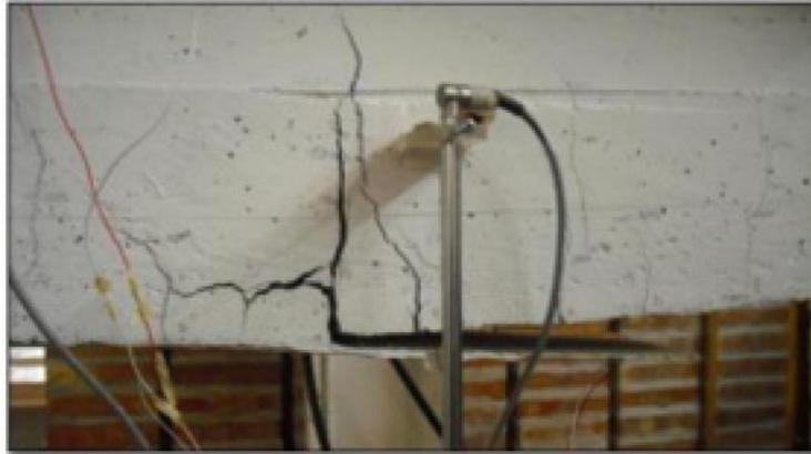
**Figure 2-3 De-bonding failure of FCRM, note the reinforcing strip protruding from the base of the beam (Ombres 2012)**
