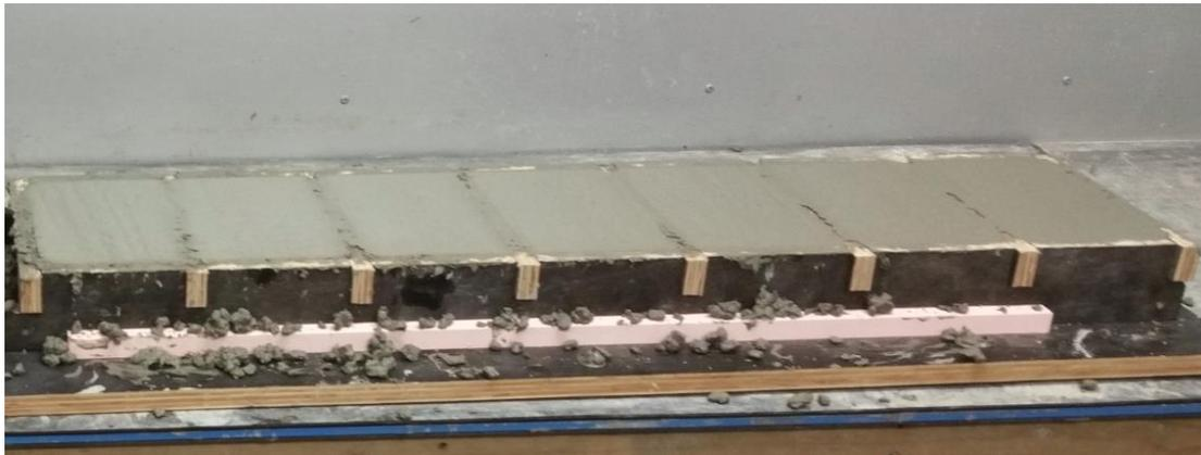
**Figure 3-4 Base Prisms Cast**
