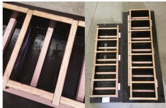
**Figure 3-2 Prism Molds - Ready for Casting**
