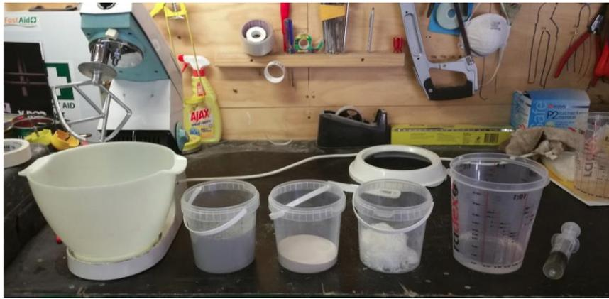
**Figure 3-7 All materials ready for mixing. Note: syringe was used to measure out super plasticiser.**
