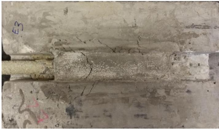
**Figure 4-3 Sample Set ECC1 Typical Failure Mode - Brittle**
