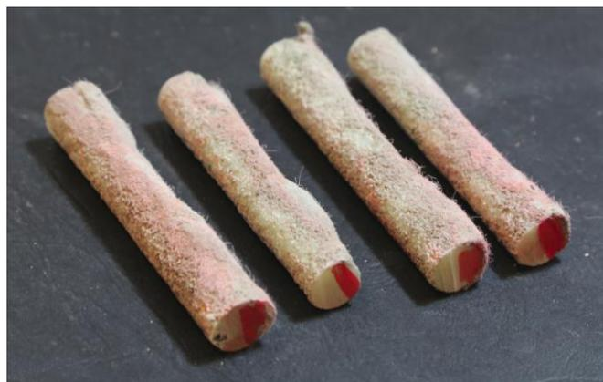
**Figure 4-12 ECC4 samples showing good of ECC on external facing side and poor bond on internal facing side.**
