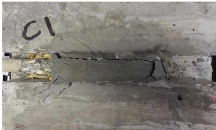
**Figure 4-1 Cover splitting in Sample C1-1**
