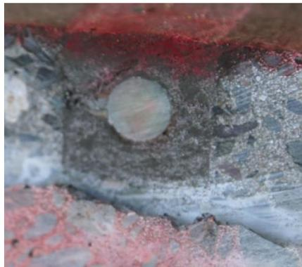
**Figure 4-19 Sample 3-1 Dye Penetration**
