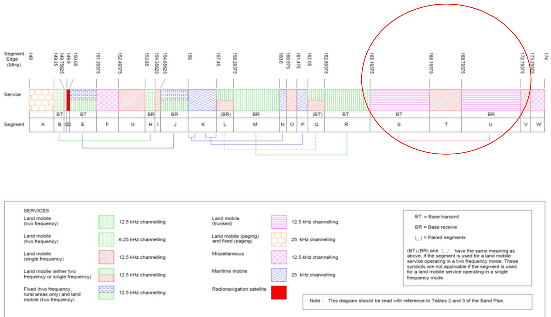
Figure 6: ACM VHF High Band Plan (Airwave Solutions P25 Rack Training, 2012)
