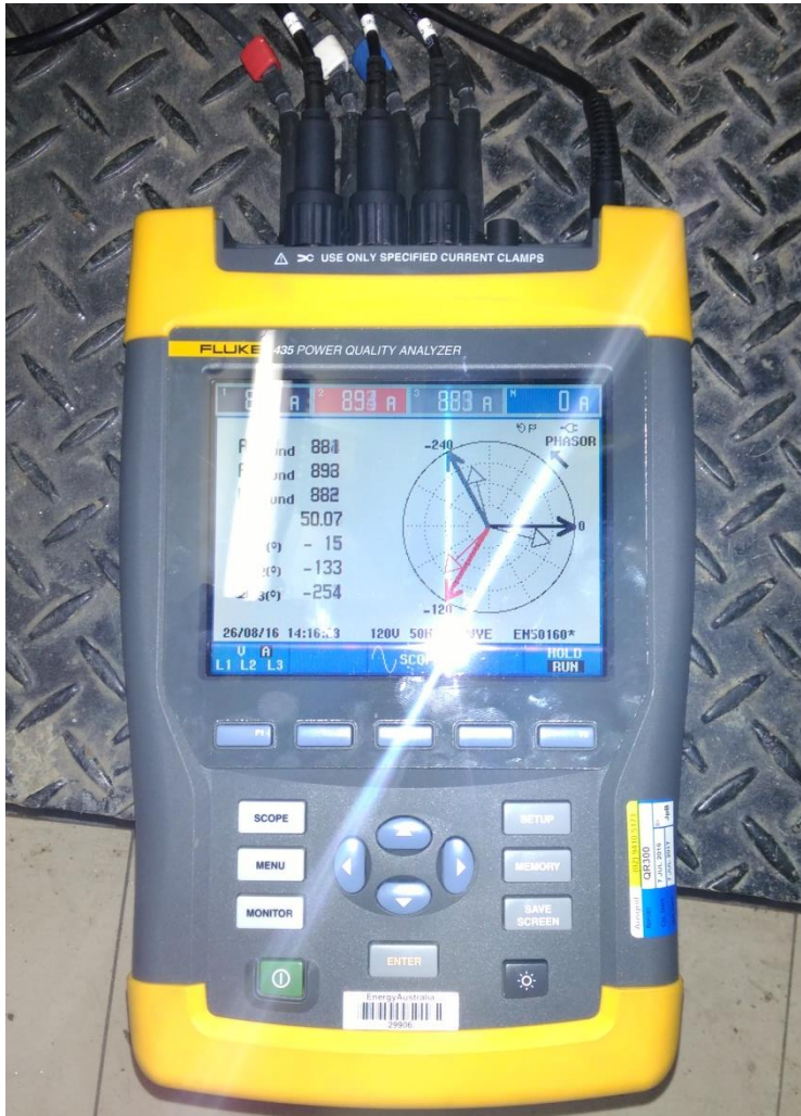
Figure 23: Fluke 435 Power Quality Analyser – zone bus phase currents
