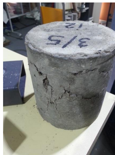
Figure 6.12: Concrete specimen failure (Proctor mould) after compressive test.
