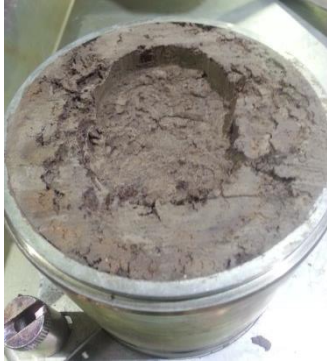
Figure 4.2: Imperfections in Vertosols soil compacted into Proctor mould
