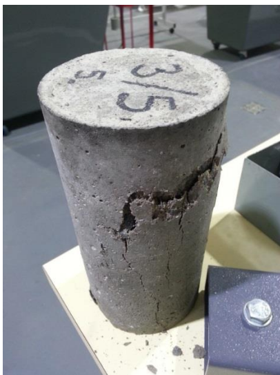
Figure 6.11: Concrete specimen failure (normal mould) after compressive test.
