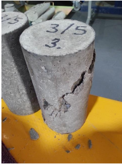
Figure 4.12: Failure of concrete specimen moulded in normal concrete moulds
