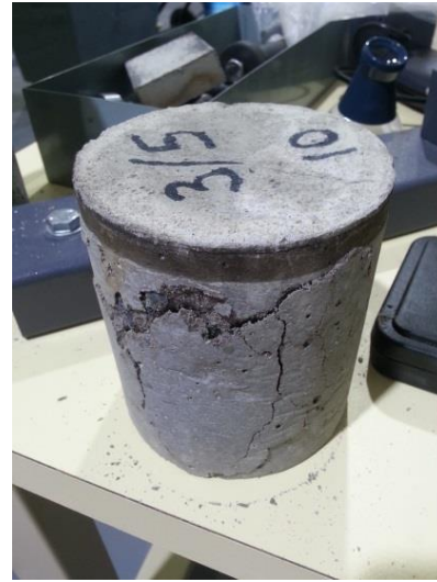
Figure 4.13: Failure of concrete specimen moulded in Proctor moulds
