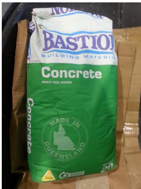
Figure 3.10: N25 Bastion Pre-Mix Concrete
