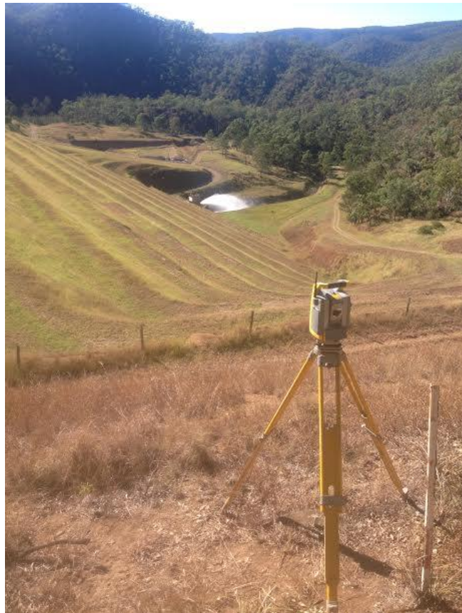
Figure 3: Trimble S6 Total Station Looking over Survey Site
