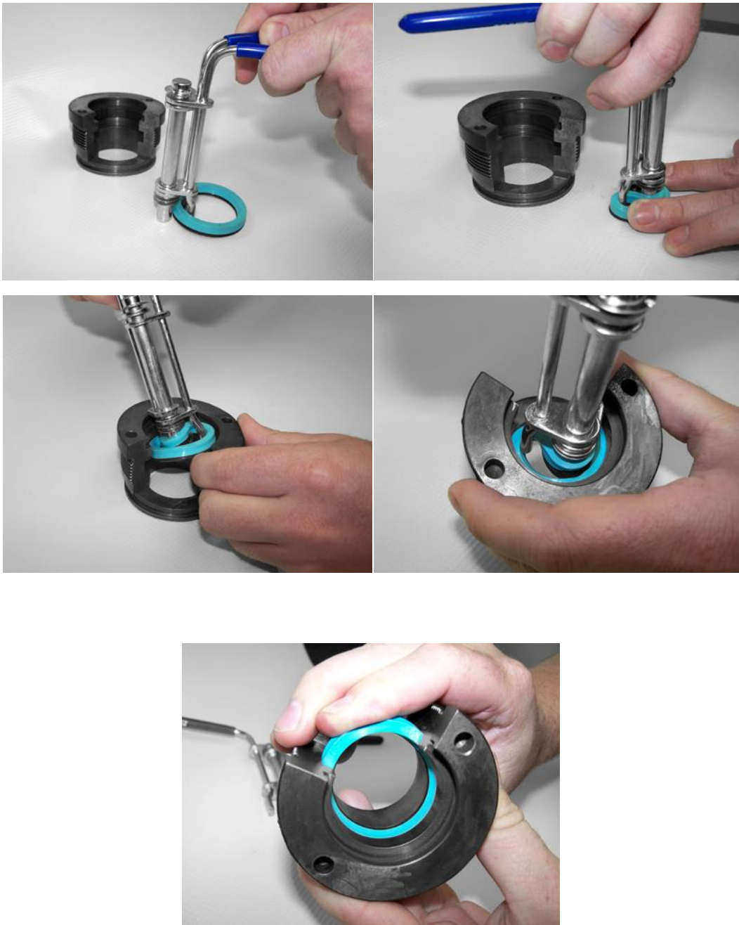
Figures 35-41 – Seal installation methods (SKF)
