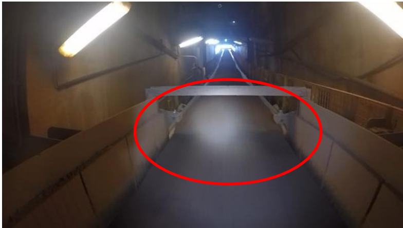
Figure B-9 Lack of load profile
