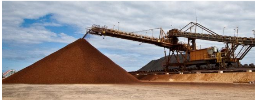
Figure 1-3 Stackers stacking iron ore in operation Source: www.fremantleports.com.au
