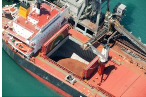
Figure 1-1 Shiploader dumping iron ore into the cargo hold of a bulk transport ship Source: www.fremantleports.com.au
