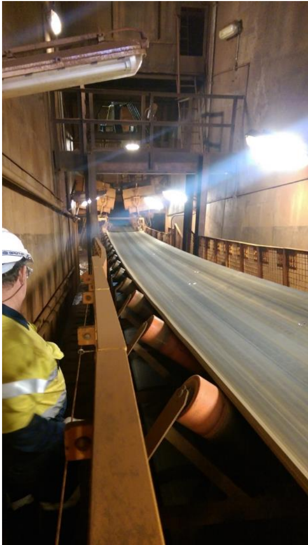
Figure B-2 Longitudinal wear lines.
