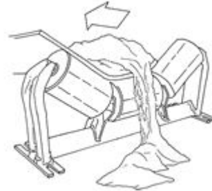
Figure 2-7b Material COG falling into trough of idler and associated spillage off edge of belt
