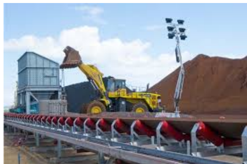
Figure 1-2 Front end loader transferring iron ore from the stockpile to the loadout conveyor. Source: www.fremantleports.com.au
