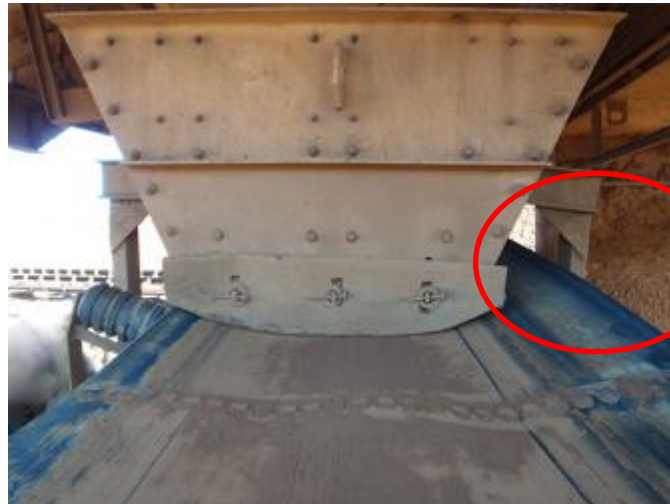
Figure 2-8 Belt edge damage from misalignment Source: www.esseng.com.au
