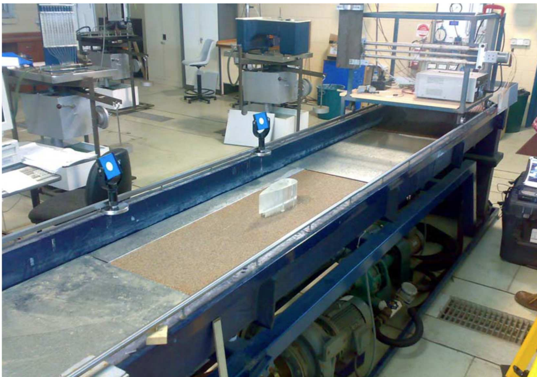
Figure 2.4 An example of a typical flume tank setup for a physical model experiment (Christensen 2009).
