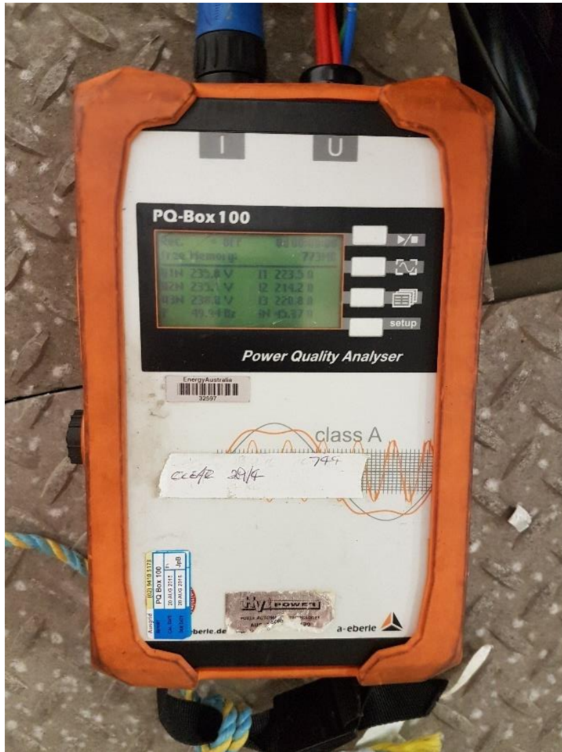
Figure 3.1 PQ-Box 100 network analyser used to survey selected sites
