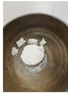
(b) Extent of shrinkage cracks
