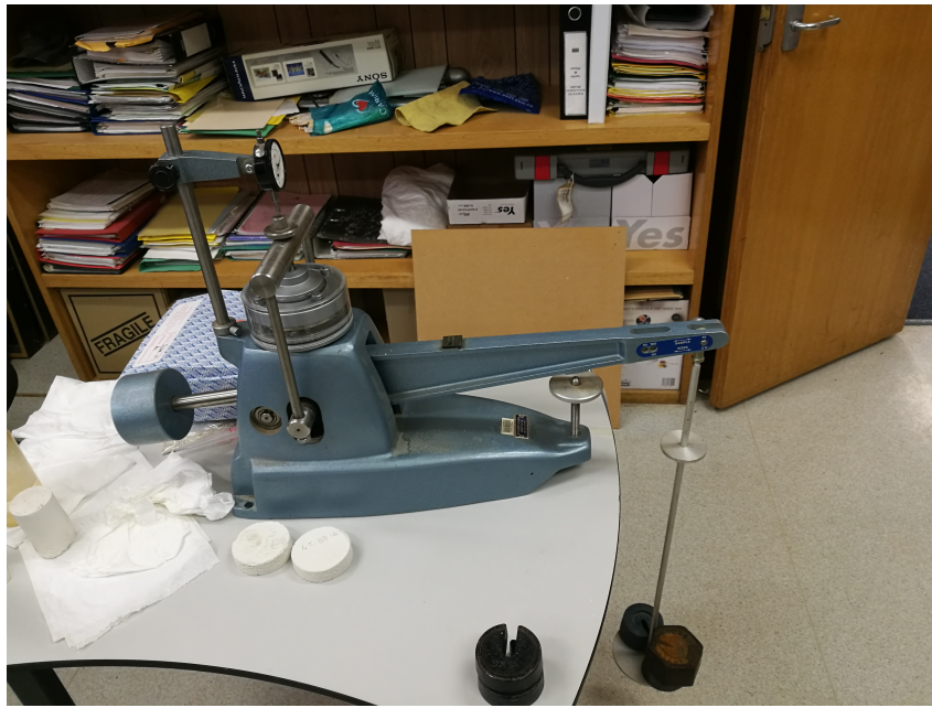
Figure 3.1: Manual oedometer used for tests
