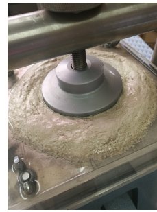
(b) Heaving of sample after initial swell
