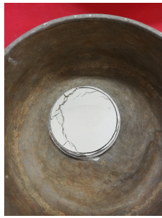
(a) Shrinkage of sample after oven dry
