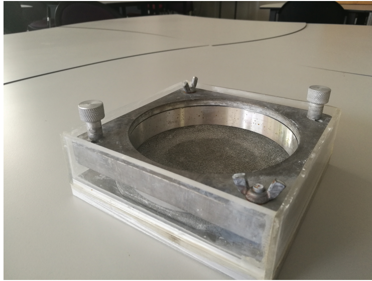
Figure 3.3: Completed cell for two-dimensional testing
