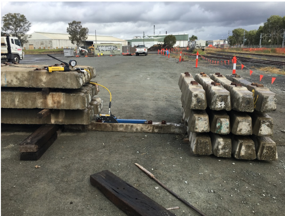
Figure 3-7: Proof Load Testing of SSPT Device
