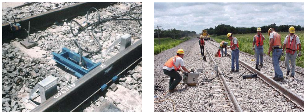
Figure 2-13: Single Sleeper Push Test Device (left) and Testing (right) (Kish 2011)
