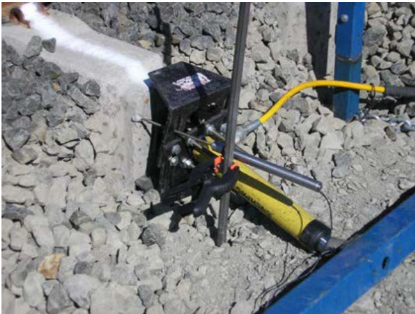
Figure 2-15: Hydraulic Cylinder Pushing End Area of Test Sleeper
