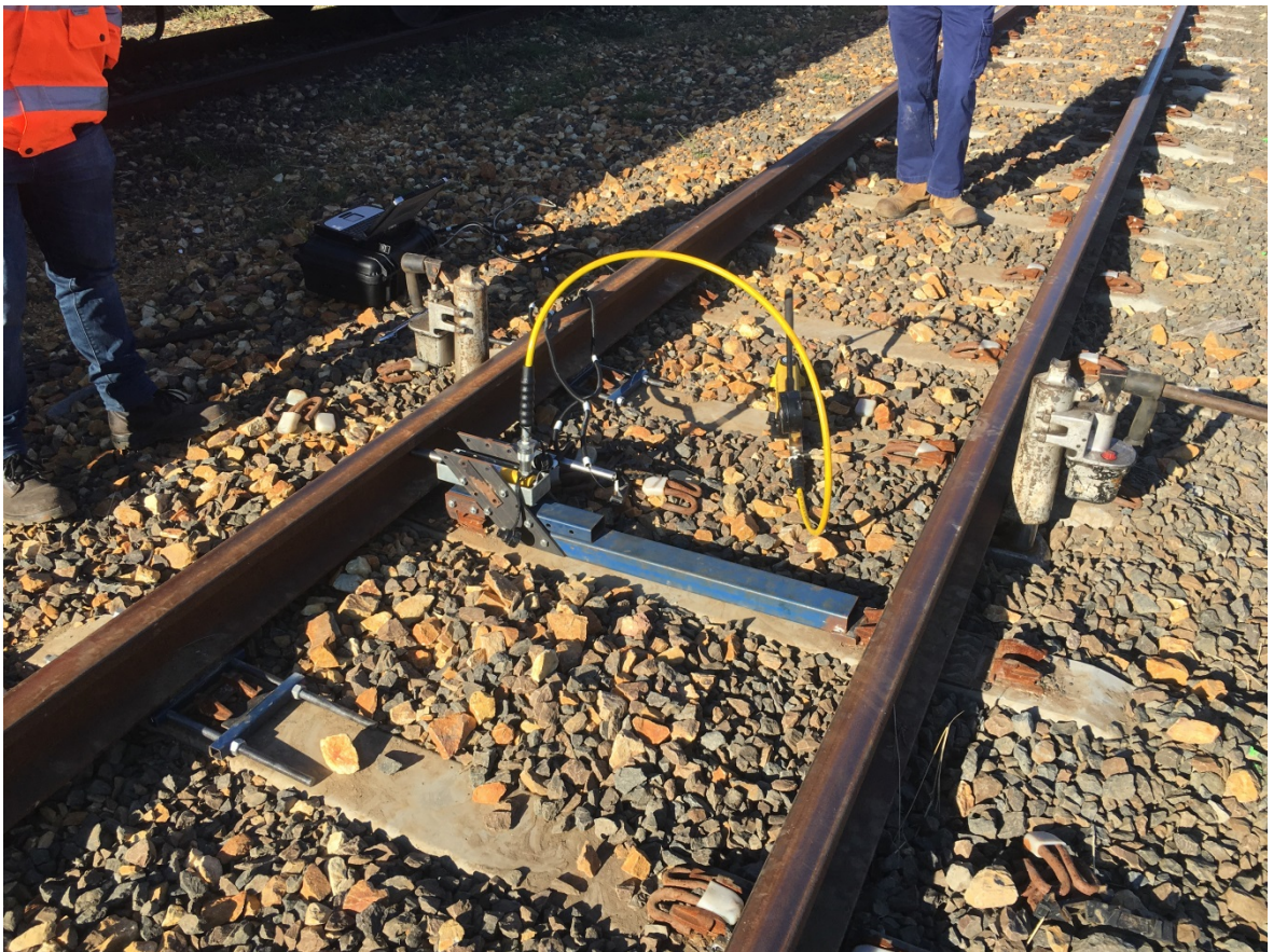
Figure 3-15: SSPT Equipment Attached to Test Sleeper
