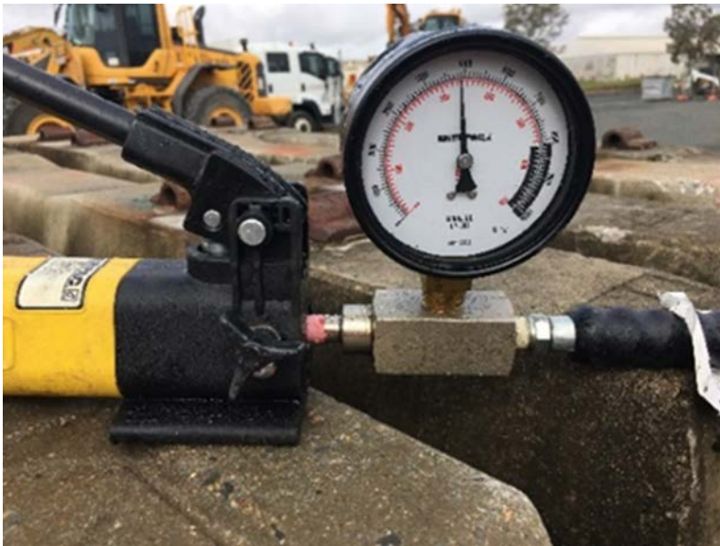
Figure 3-8: Pressure Gauge used to Measure Test Loads
