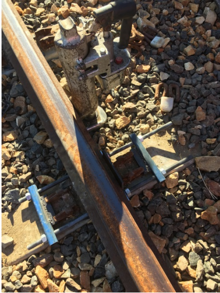
Figure 3-16: Rail Fixture attached to Reaction Rail
