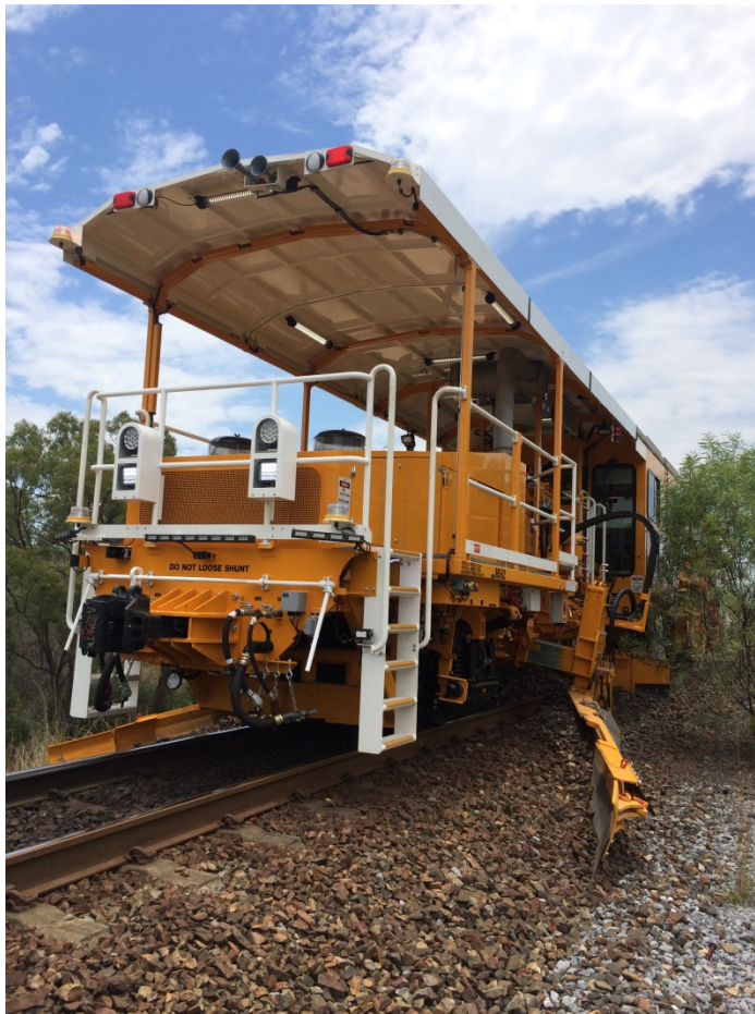
Figure 2-6: Ballast Regulator working its Shoulder Ploughs
