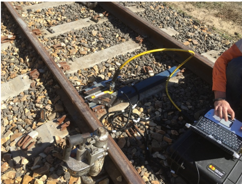
Figure 3-9: Data Acquisition Setup
