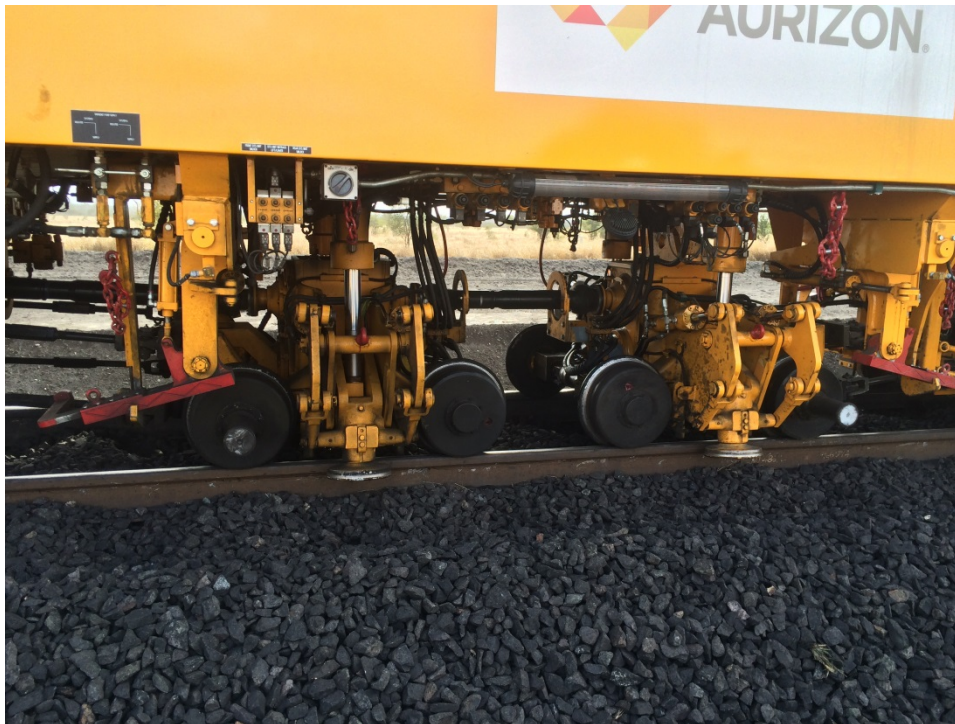
Figure 2-8: Stabilising units of a Dynamic Track Stabiliser
