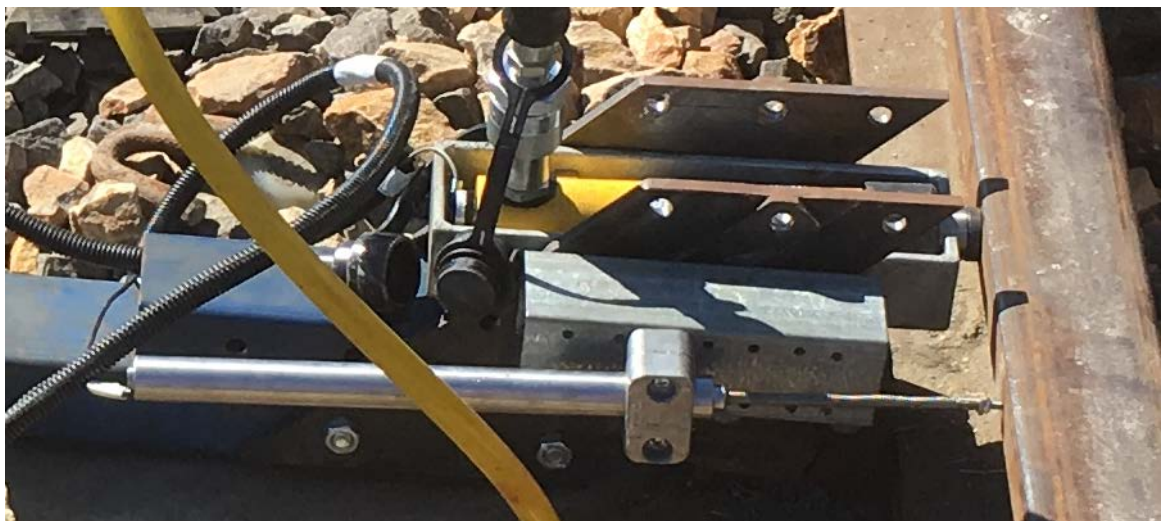
Figure 3-10: Load Cell and LVDT Setup
