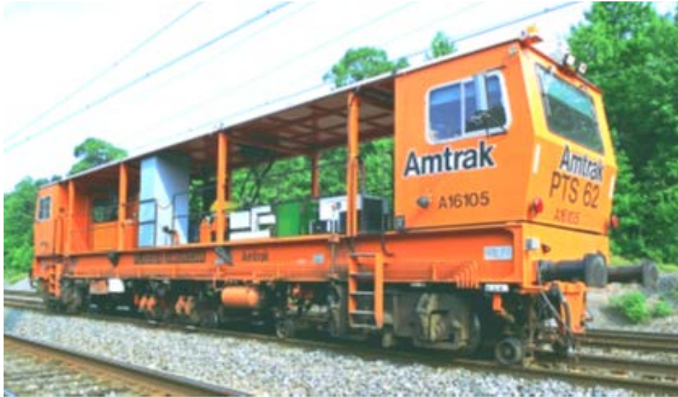
Figure 2-7: Dynamic Track Stabiliser (Kish 2011)
