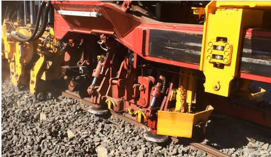
Figure 2-4: Clamp Frame of a Tamper Liner
