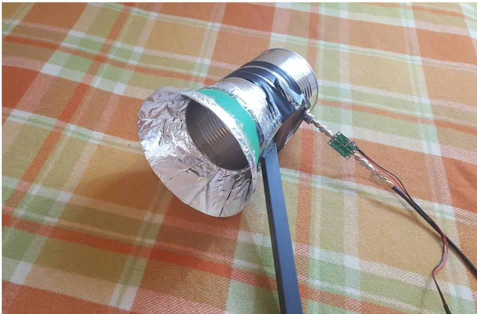
Figure 5.7: Cylindrical waveguide with expanded opening.
