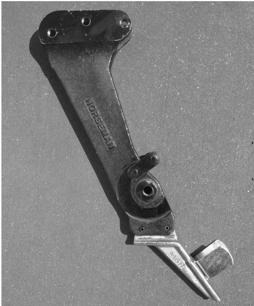
Figure 50 – Throat fitted with nonstandard seed tube guard
