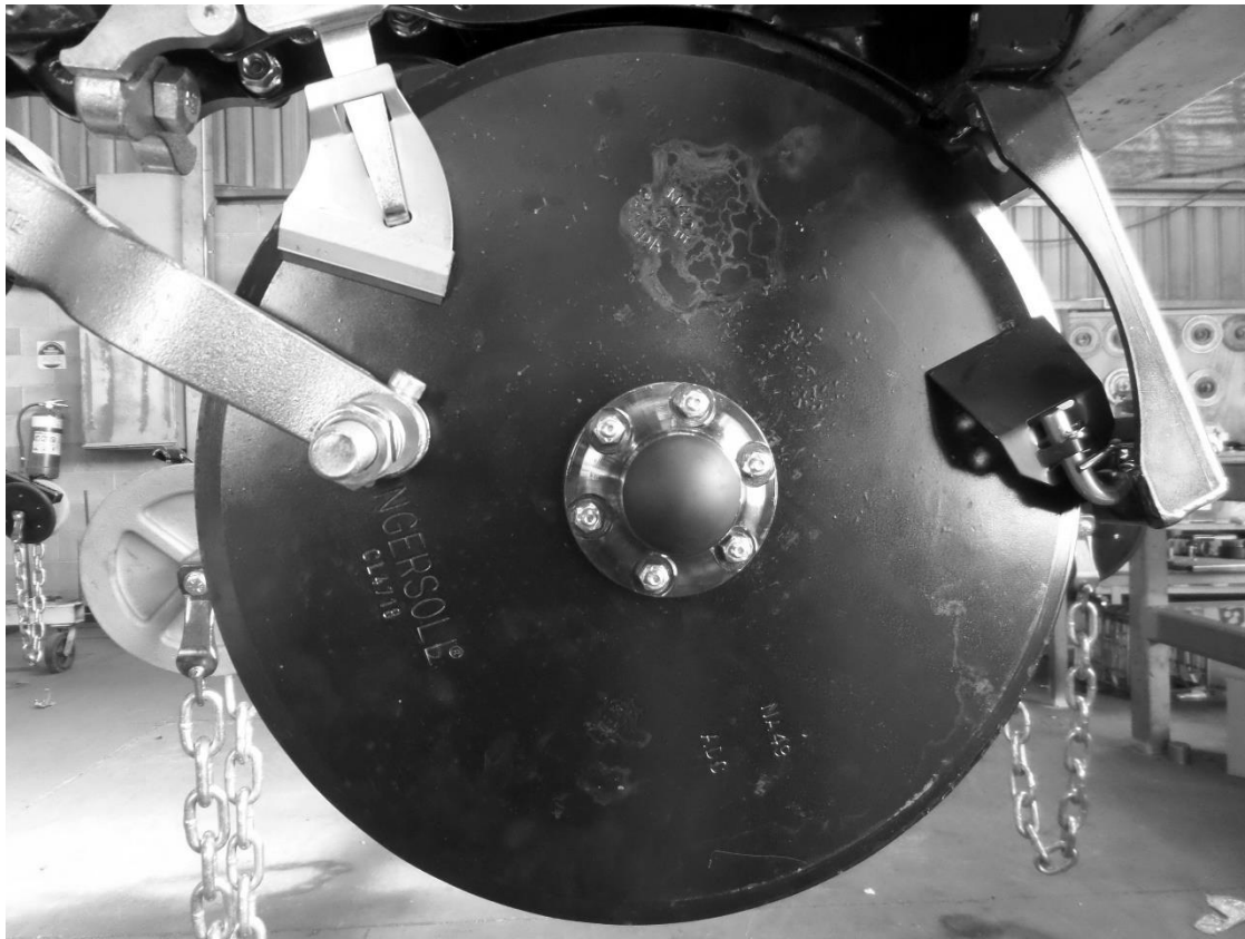
Figure 18 – Opening Disc. Gauge wheel removed for clarity
