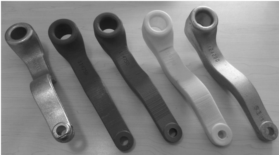
Figure 39 - Progress from old design (left) to new design (right)
