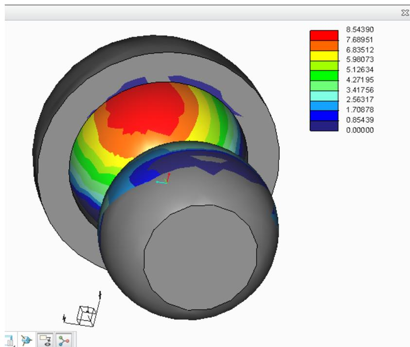
Figure B.8: contact pressure of diameter 28 mm at zero clearance.
