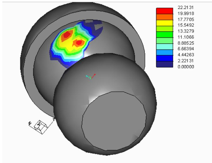
Figure B.3: contact pressure of diameter 50 mm at 24  $\mu$  clearance.
