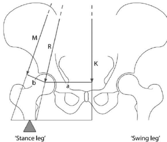
Figure 2.5: Free body diagram of the hip joint
