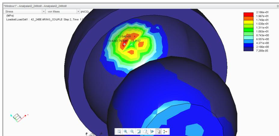
Figure 6.7: Contact with 30  $\mu\text{m}$  clearance.
