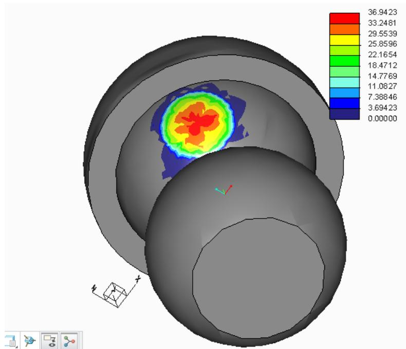
Figure B.7: contact pressure of diameter 36 mm at 30  $\mu$  clearance.
