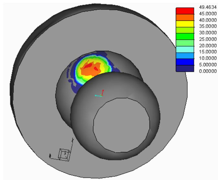
Figure B.9: contact pressure of diameter 28 mm at  $30 \mu$  clearance.
