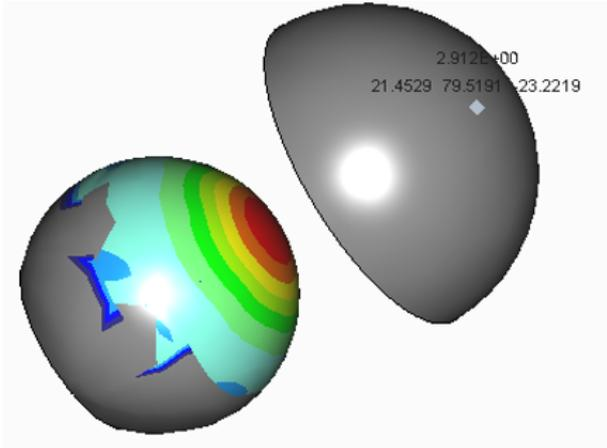
Figure 7.5: Contact stress distribution of the new design.
