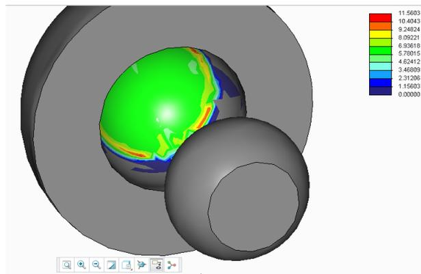
Looking at figures 6.8 and 6.9 it can quickly be seen that the elliptic model had lower contact pressures than the spherical model. The referred figures are for the 28 mm diameter head only but the full comparison is delt with in chapter 7.
