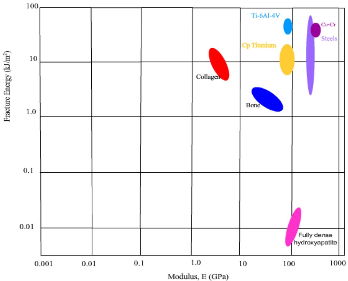
Figure 4.1: Comparison of fracture toughness. Source: Capes and McCloskey (2006)
