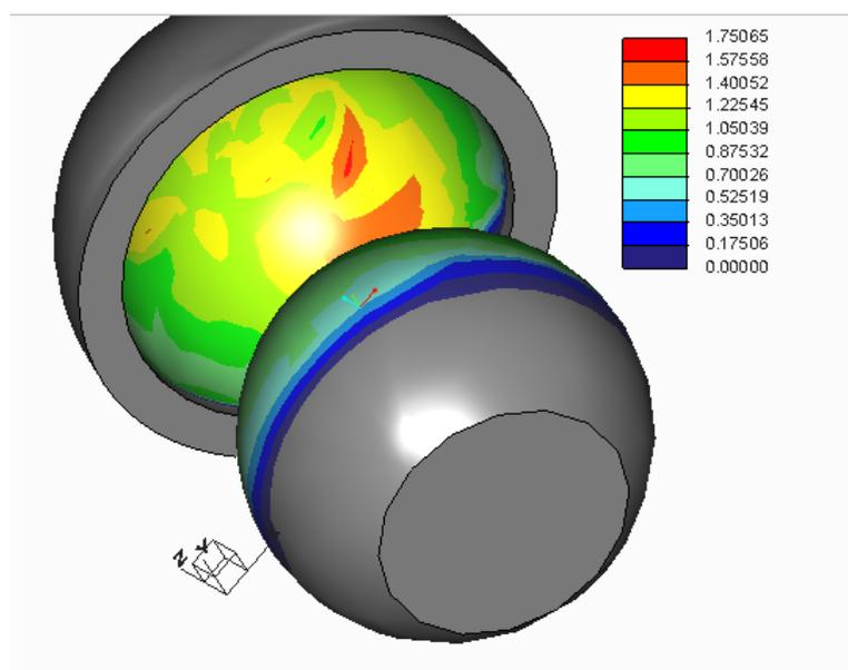
Figure B.2: contact pressure of diameter 50 mm at zero clearance.
