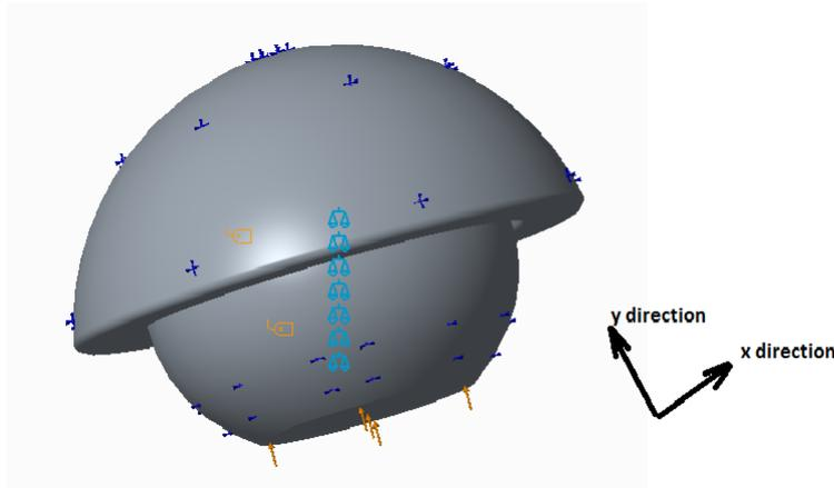
between the peek liner and the femoral head surfaces has got finite friction set at 0.15 of which the value is derived from online material data sheets attached in the appendix B.
