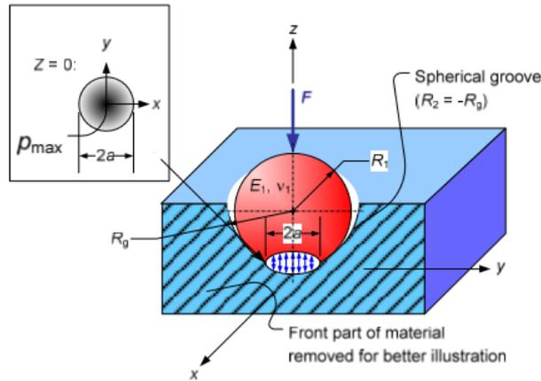
Since the femoral head is made of the hard material it indents the Peek there by deforming it more than itself creating contact area of radius  $a$ . Given that  $F$  is the normal applied force,
