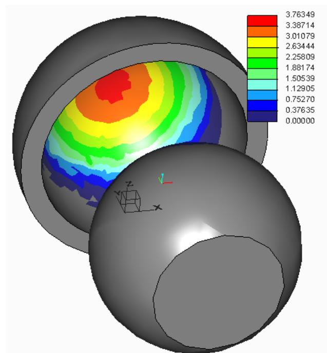
Figure B.4: contact pressure of diameter 50 mm at 30  $\mu$  clearance.
