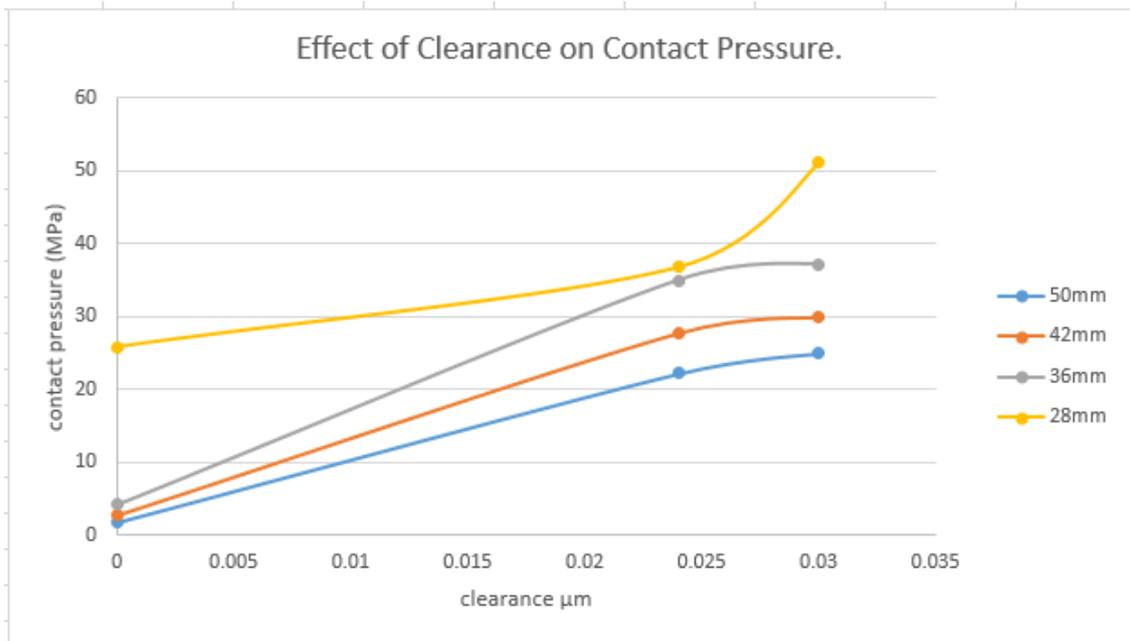
Figure 7.1: Contact stress by FEA method.
