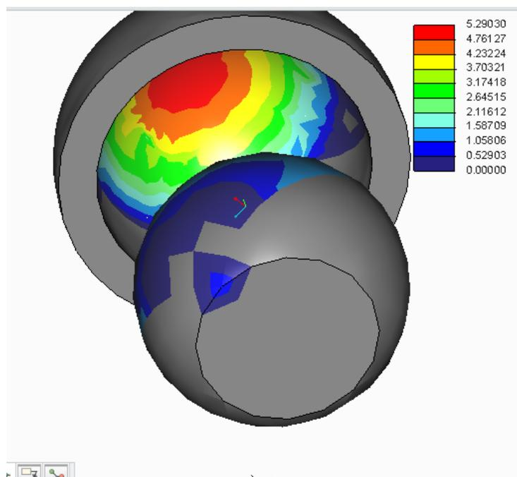
Figure B.6: contact pressure of diameter 36 mm at 24  $\mu$  clearance.
