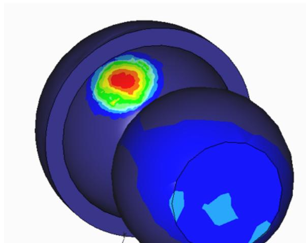
noted that the size of the contact area decreases as the diameter differences increase. This is discussed further in chapter 7, The figures 6.5 to 6.7 are an illustration of the variation of the contact stresses with clearances for a 42 mm diameter head only. For the bearing sizes 28 mm, 36 mm, 42 mm, and 50 mm each had three analyses for the zero, 24  $\mu\text{m}$ , and 30  $\mu\text{m}$  diametrical clearances.
