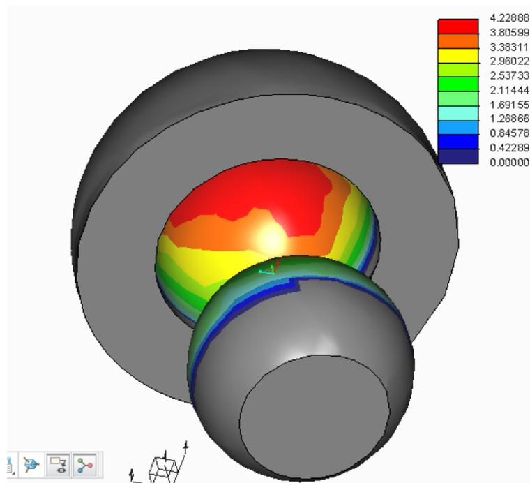
Figure B.5: contact pressure of diameter 36 mm at zero clearance.
