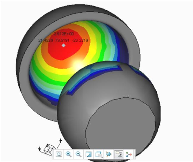
Figure 7.4: Contact stress distribution of the new design.
