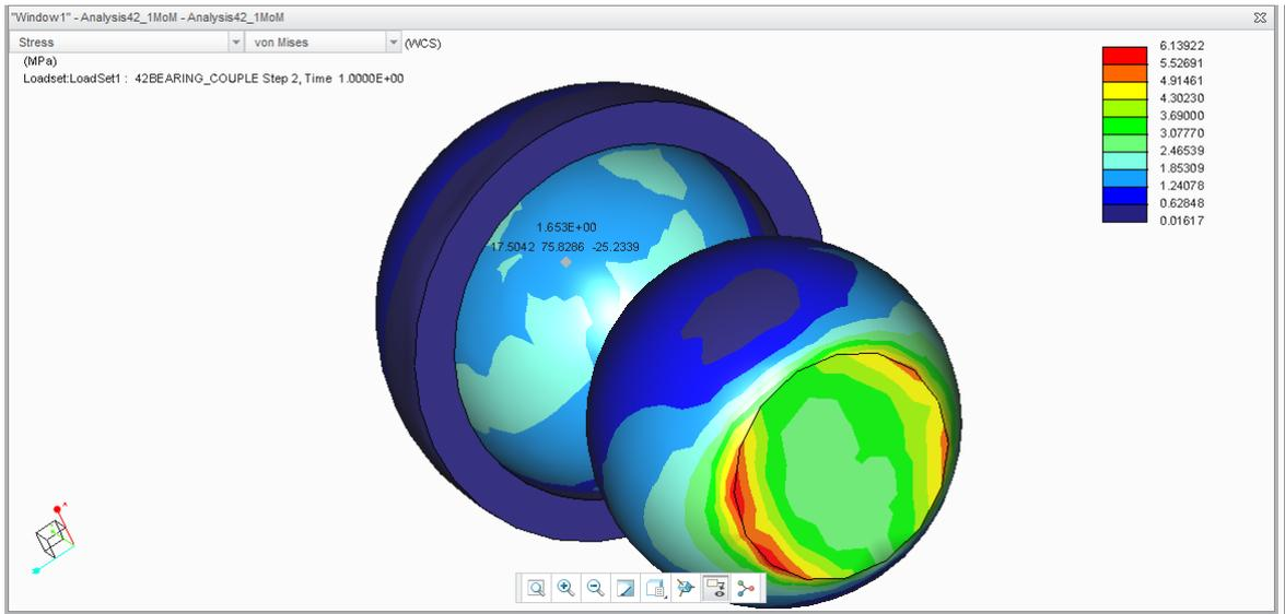
Figure 6.6: contact with 24  $\mu\text{m}$  clearance.
