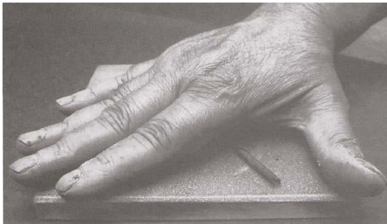
Figure 11. Rolling of soil mass on ground glass to determine plastic limit (Das, 2008)
