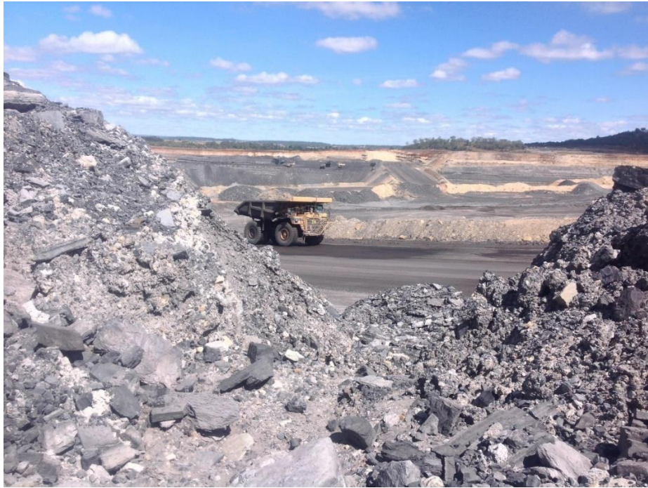
Figure 1 Example of Interburden at New Acland mine demonstrating varying shapes and sizes of coarse fragments. Interburden on the front left and front right are from two sources, but will eventually be placed in the same soil profile.
