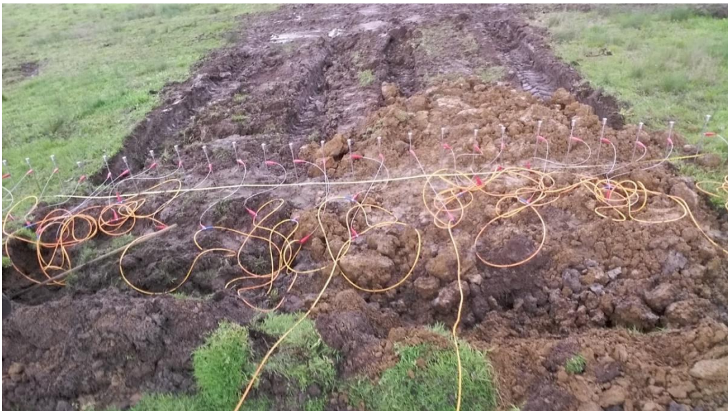
Figure 19 Variability trial buried with electrodes
