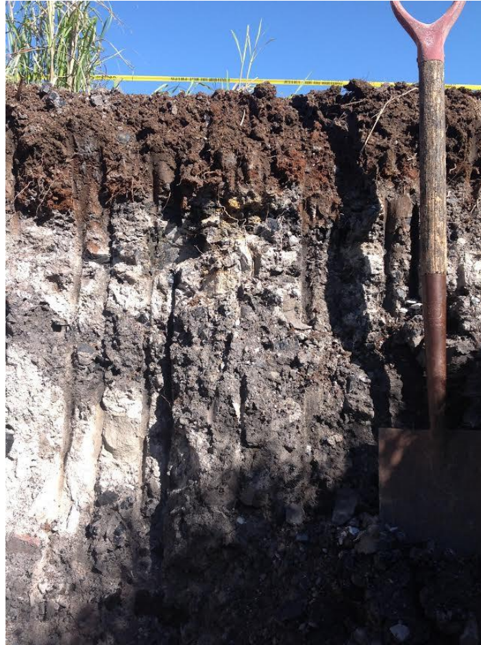
Figure 2 Soil profile of buried interburden with \approx 30\text{cm} of soil as overburden. Note the heterogeneity of interburden colour (source) and coarse fragments.
