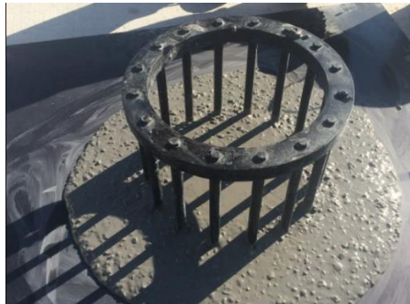
Figure 4.7: J-ring apparatus used for testing passing ability
