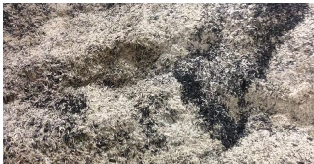
Figure 4.6: RHA material following firing process
