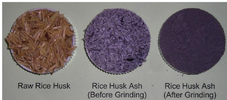
Figure 2.1 - Development of Rice Husk to Ash (Aprianti et al. 2014)
