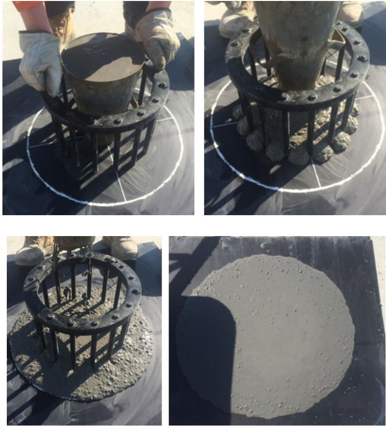
Figure 4.8: Testing procedure using J-ring apparatus
