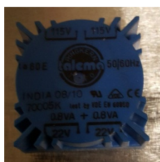
Figure 3.13 – Transformer with high magnetising inductance used in initial charging circuit (Stephens 2016)
