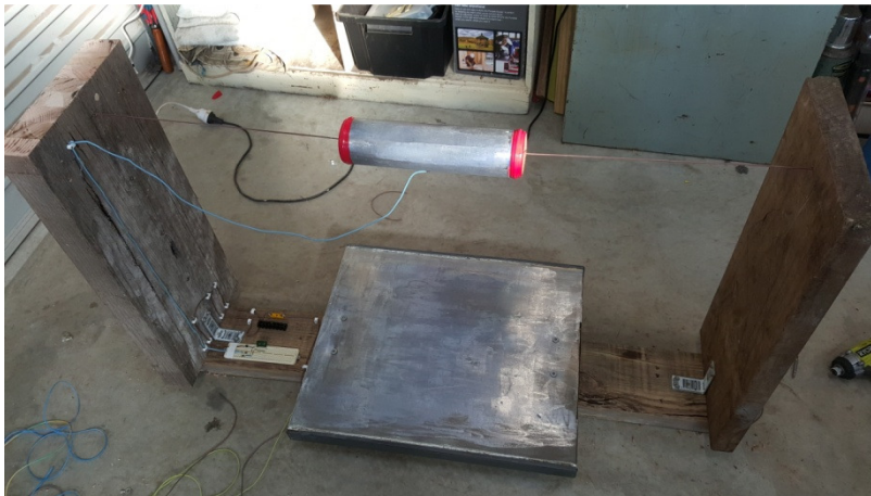
Figure 3.10 – Electric field energy harvesting experiment apparatus (Stephens 2016)
