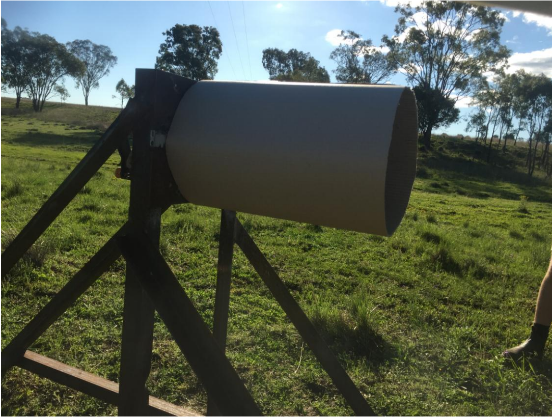
Figure 4.3.2 - Test frame with cardboard tube in position ready for a test shot.
