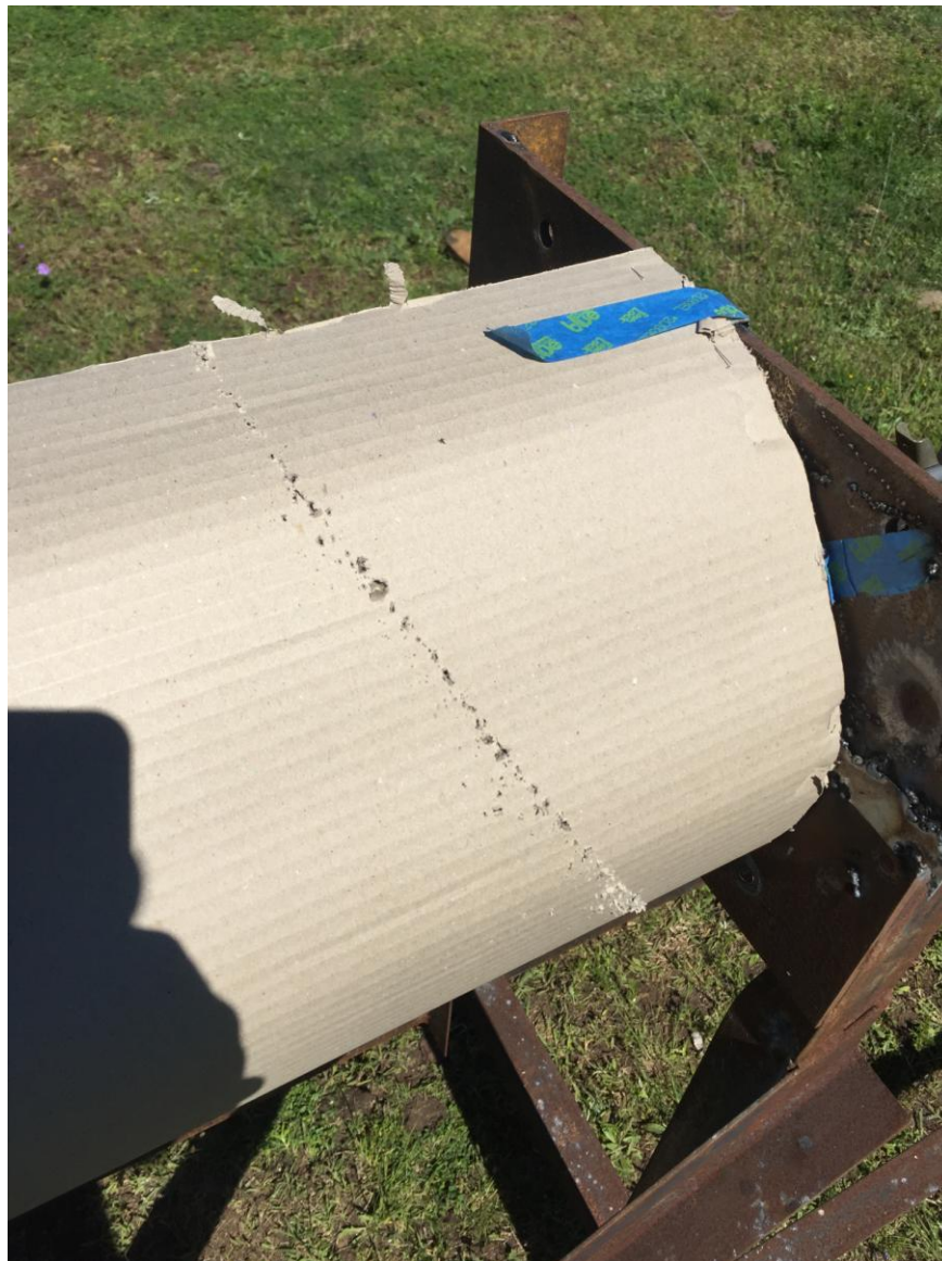
Figure 5.1.1 - Resulting damage of a 60° test shot, it should be noted that the distribution of fragments has begun to thin across the top of the circle, but it is still complete.
