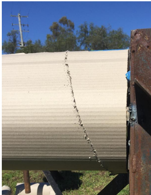
Figure 6.1.1 - The clear cut line of fragment damage to the testing cardboard indicating the projected plane on which the fragments travel.
