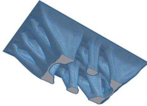
Figure 3.8 -The organic shape of an optimised structure. Image from (Clausen, Andreassen & Sigmund 2015)
