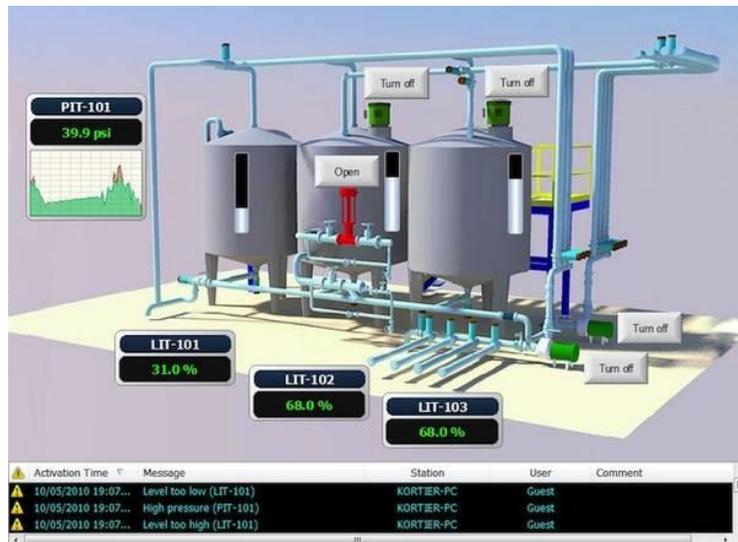
Figure 5: Example HMI screen of a plant process (Katzel 2012)
