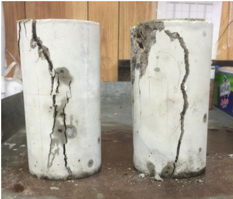
Figure 32: Batch 3 28 day crushed sample
