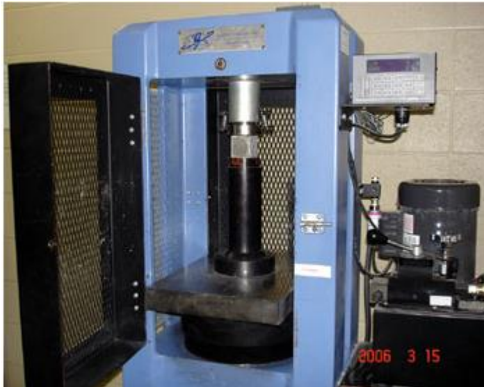
Figure 23: Compression Testing Machine (Research, 2016)
