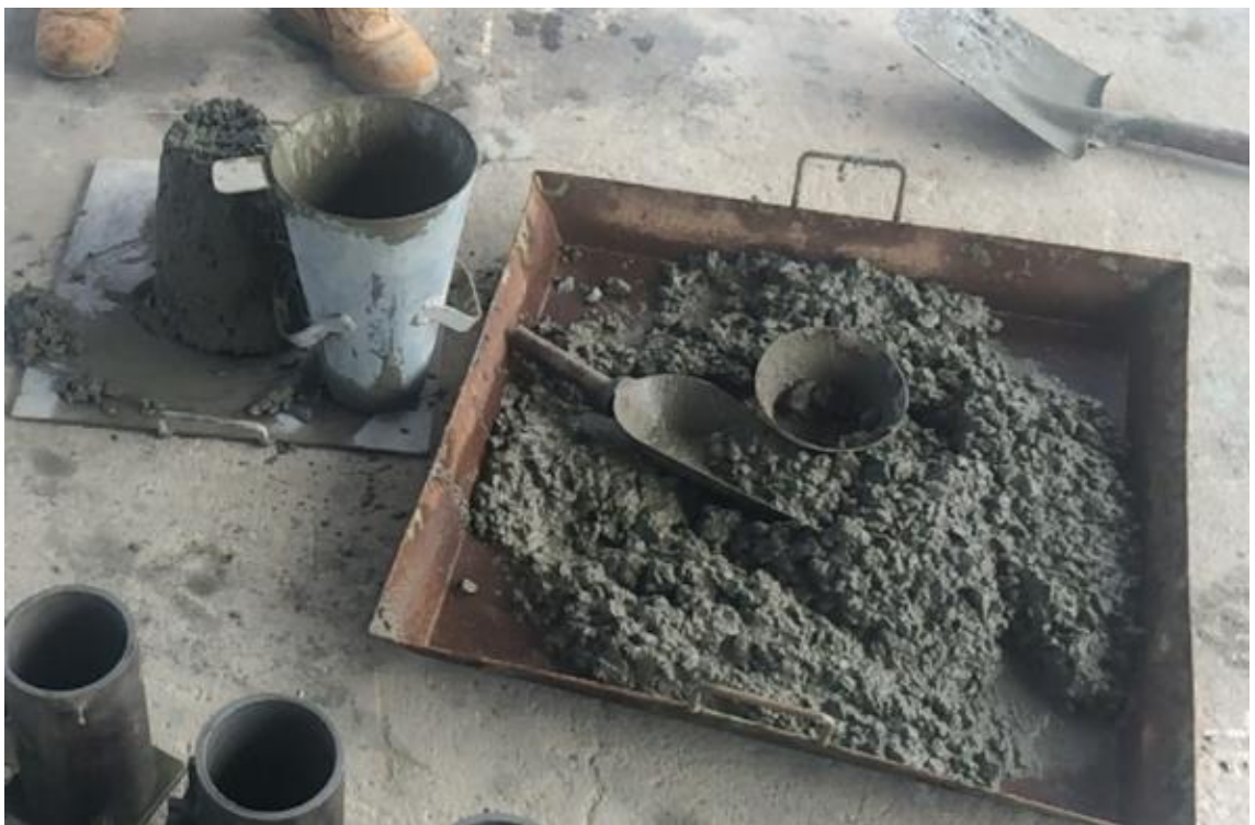
Figure 26: Slump Testing in accordance with AS1012.3.1
