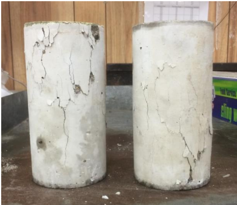
Figure 34: Batch 5 28 day crushed sample
