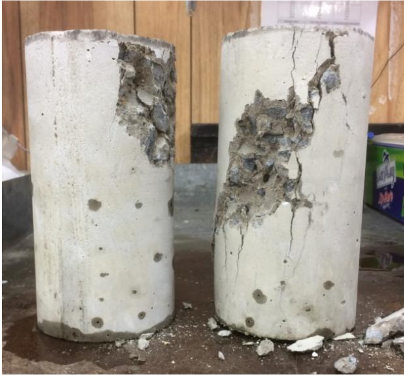
Figure 31: Batch 2 28 day crushed sample
