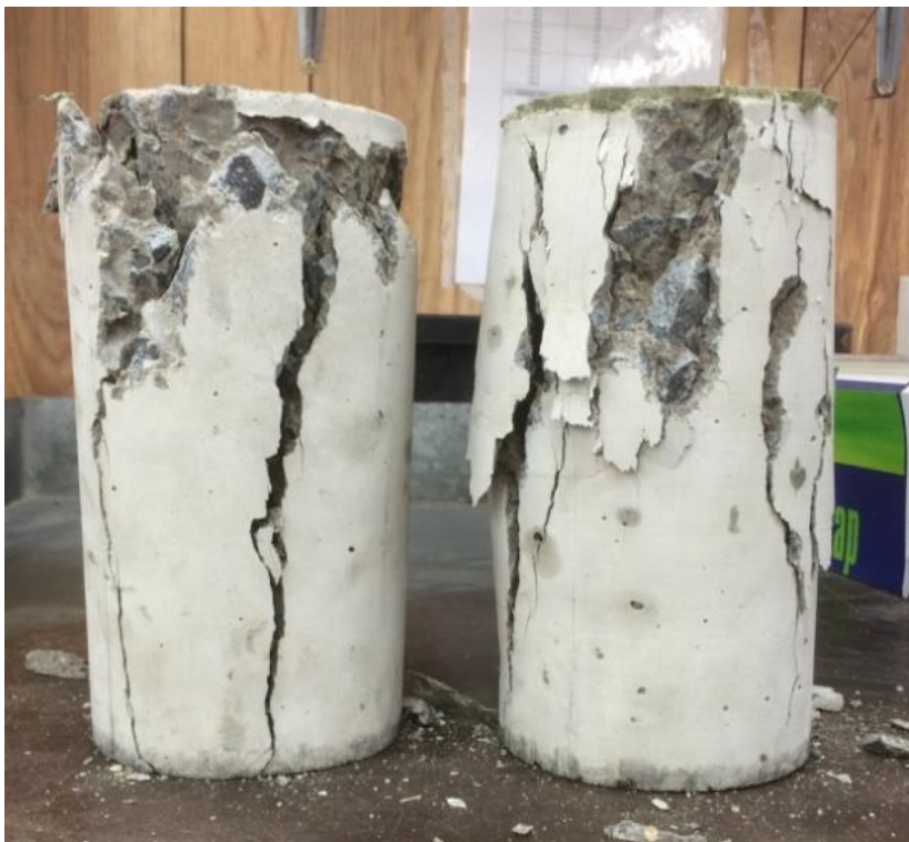
Figure 30: Batch 1 (adjusted) 28 day crushed sample
