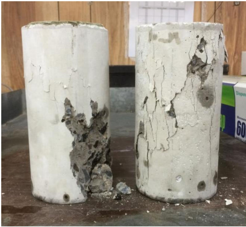
Figure 33: Batch 4 28 day crushed sample
