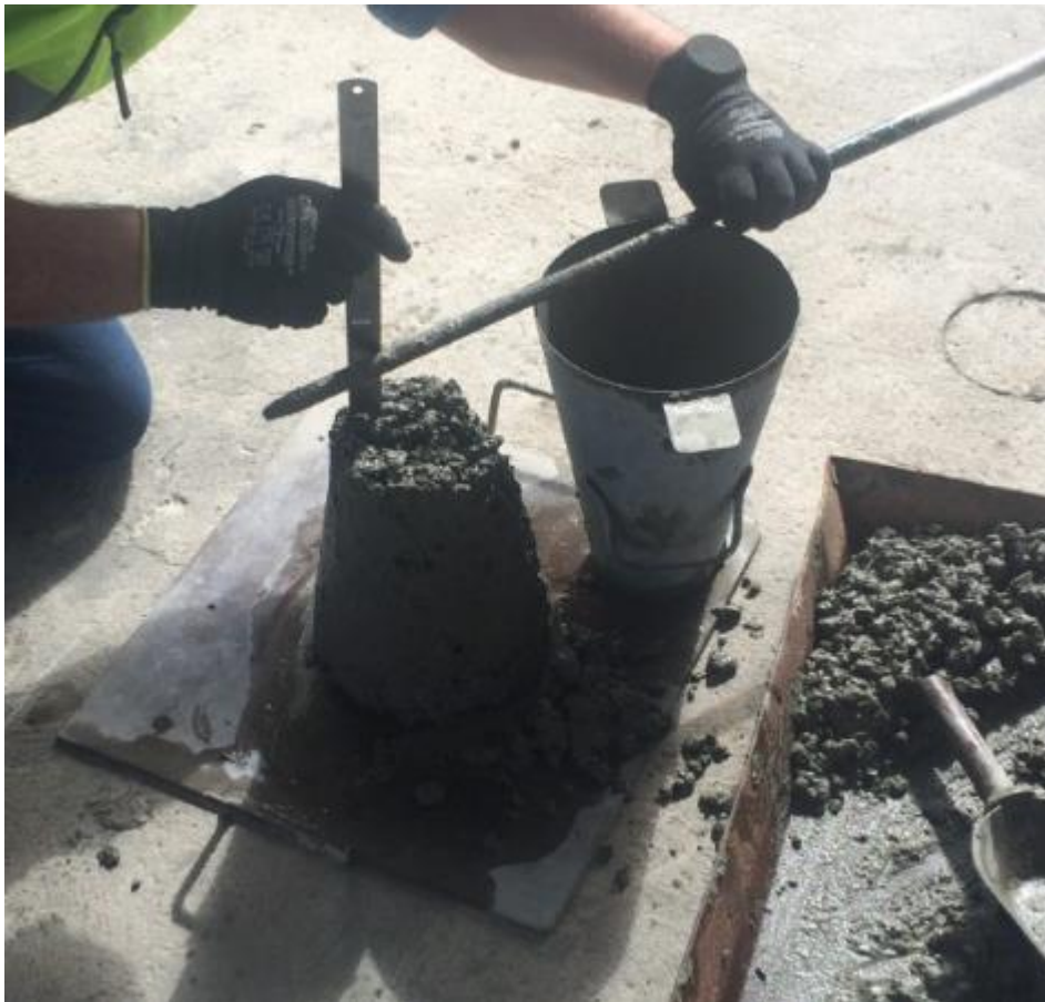
Figure 27: Slump testing of fresh concrete in accordance with AS1012.3.1
