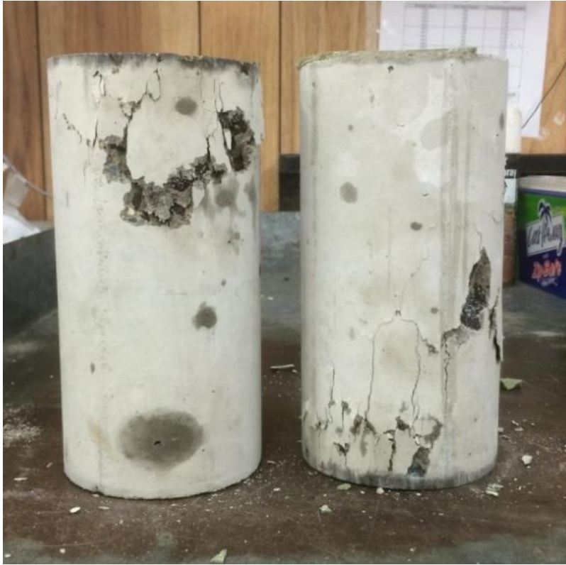
Figure 35: Batch 6 28 day crushed sample
