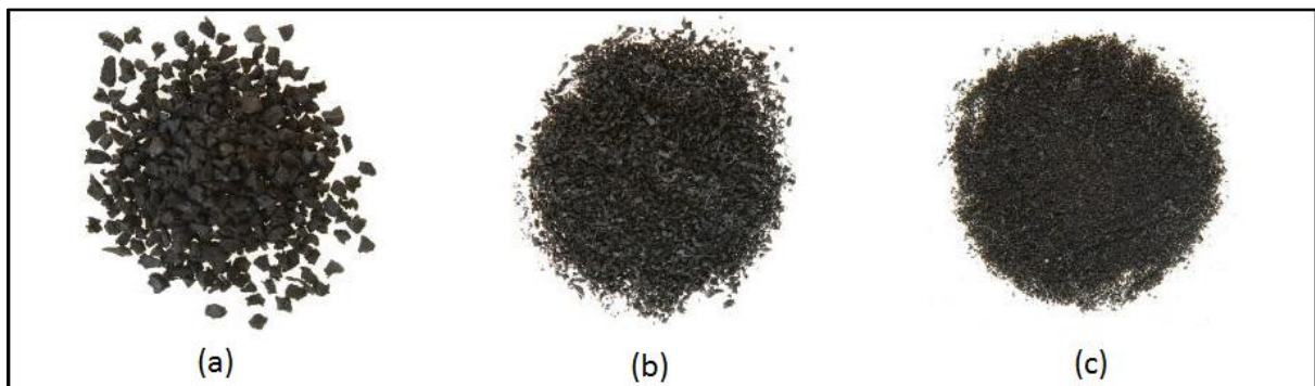
Figure 1: The three main types of recycled rubber used in CRC, (a) chip rubber, (b) crumb rubber and (c) ash rubber (ReRubber 2016).
