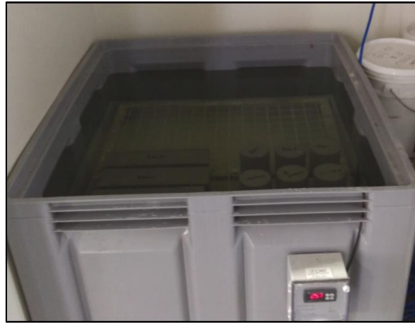
Figure 9: Specimens submerged in curing tank set to 24^{\circ}\pm 2^{\circ} .
