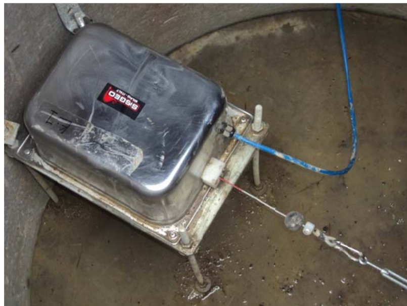
Figure 12 – SISGEO wire extensometer in typical below ground installation (Geotesta 2012)
