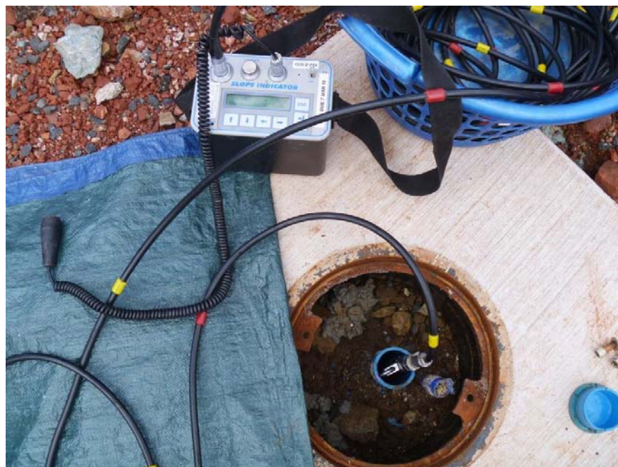
Figure 5 – Probe, cable and Datamate set up for reading inclinometer
