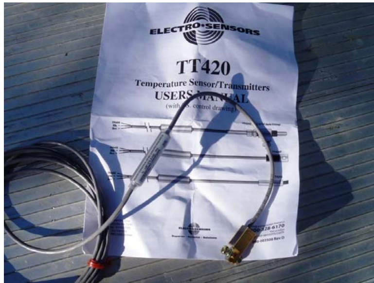
Figure 61 – 4 to 20 mA temperature sensor
