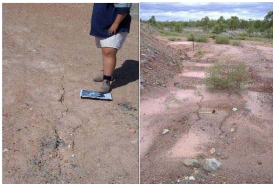
Figure 39 – Observed cracking in the vicinity of the West Wall Fault (Coffey Geotechnics 2011a)
