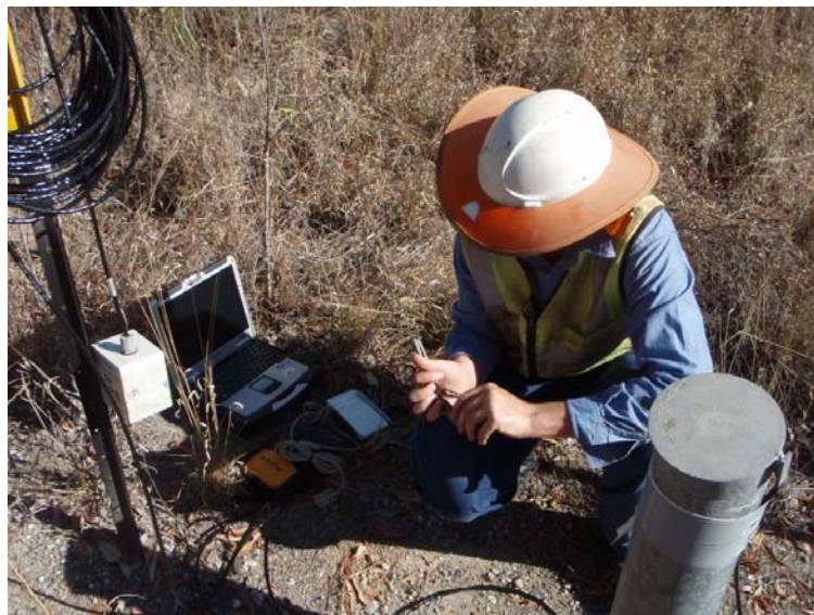
Figure 42 – Installation of VWP and logger in existing monitoring well
