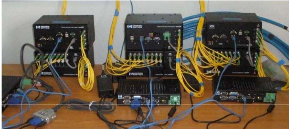
Figure 27 – Micron Optics interrogators, multiplexers and processors located in the site hut
