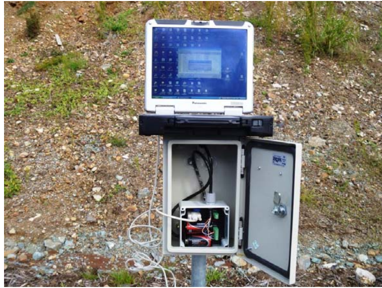
Figure 29 – VW Mini Logger connected to PC for data retrieval
