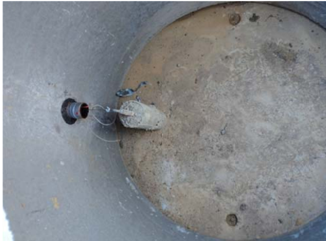
Figure 16 – Anchor end of the wire extensometer on the Morwell site (Geotesta 2012)
