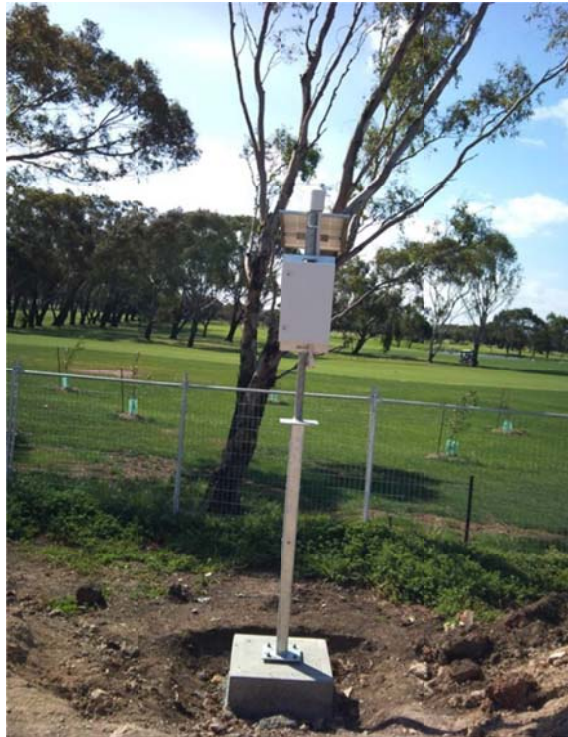
Figure 17 – Logger enclosure and solar panel on the Morwell site (Geotesta 2012)
