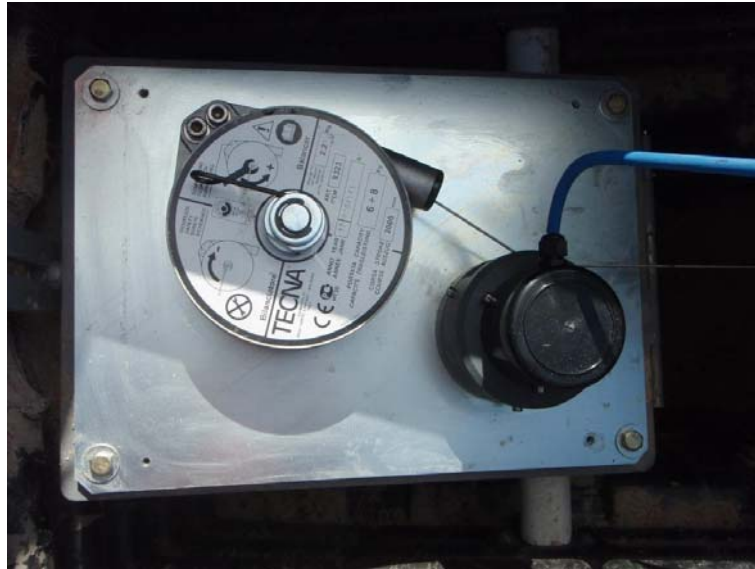
Figure 13 – Wire extensometer internal components
