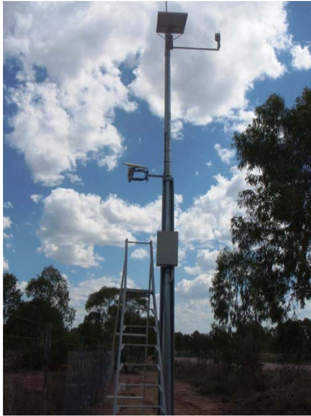
Figure 65 – Completed installation showing logger box (bottom), satellite antenna (mid), weather station and solar panel (top)
