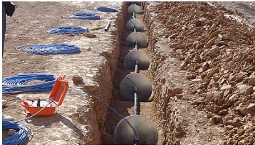
Figure 19 – Soil strainmeter installation (SISGEO 2010)
