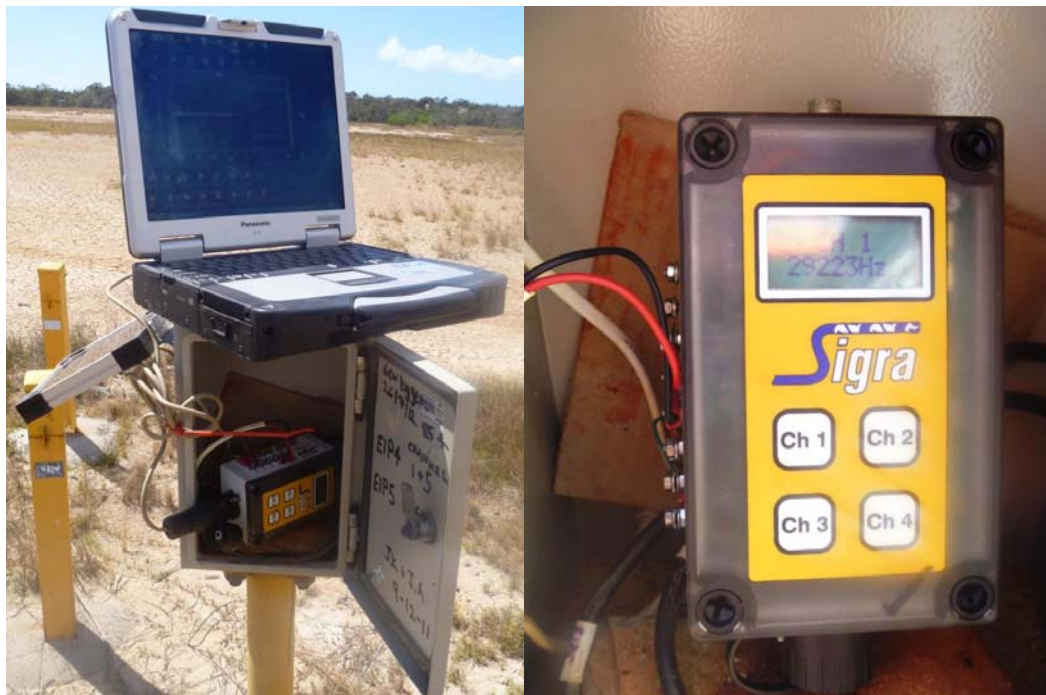
Figure 30 – Sigra logger data retrieval with a PC
