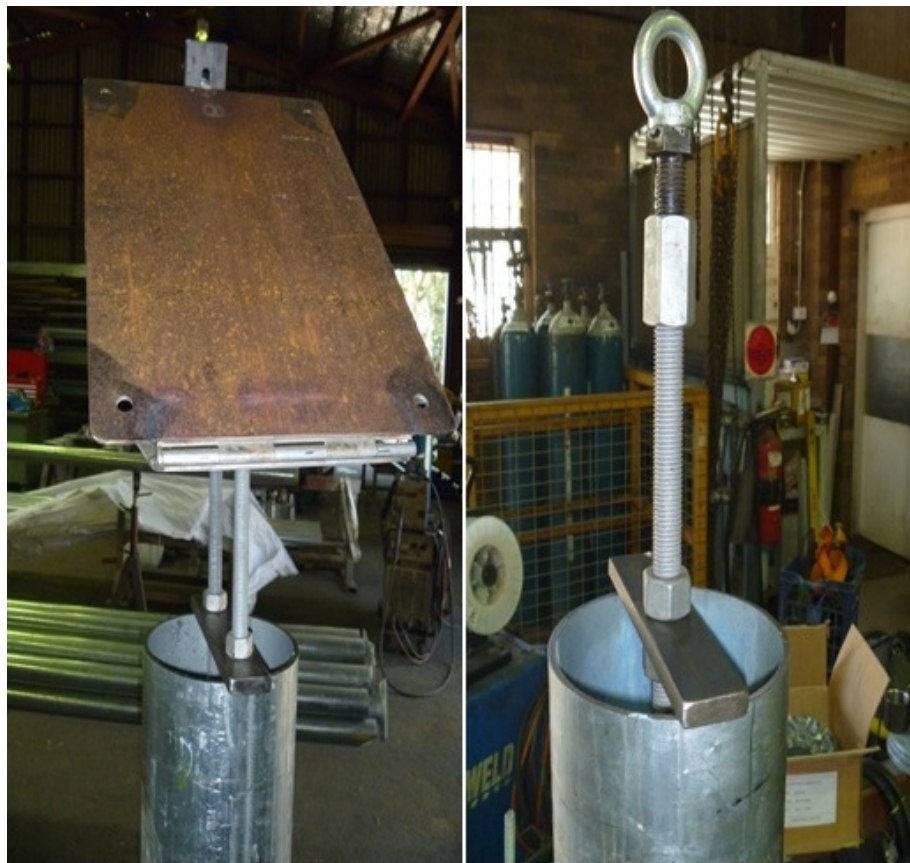
Figure 43 – Adjustable brackets: live end (left) and anchor end (right)
