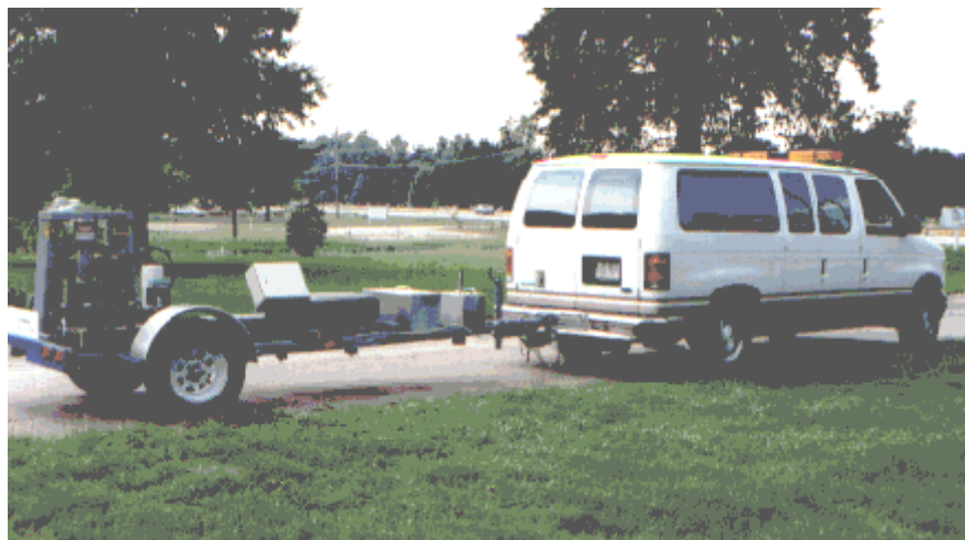
Figure 5.2 Falling Weight Deflectometer
