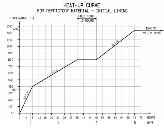
Figure 6.6: Anode furnace heat-up curve.
