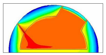
Figure 7.2: Temperature distribution for tuyere position lid-on
