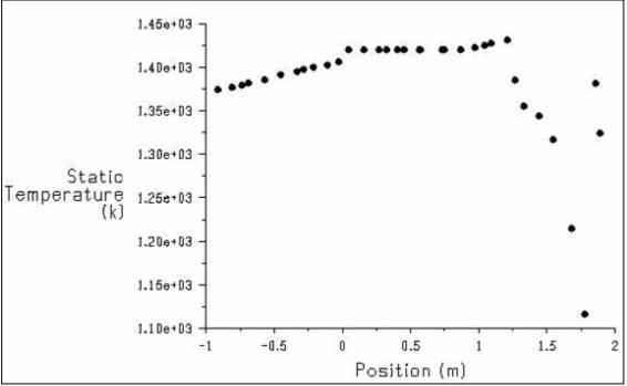
Temperature Distribution Graph for Mouth Burner. 1200°C heating results from Fluent
