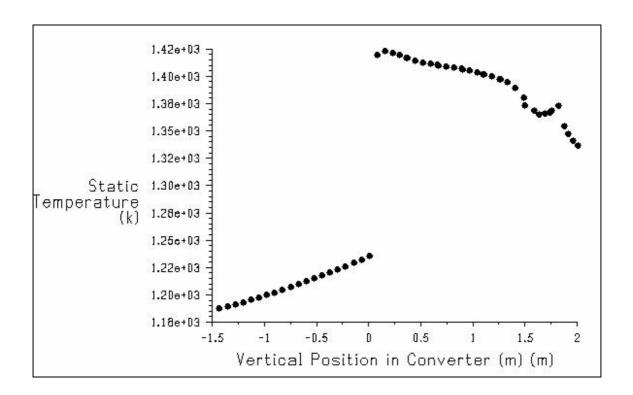
Temperature Distribution Graph for Side Wall Burner, Lid-on 1200°C heating results from Fluent
