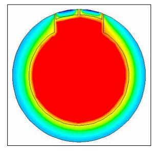
Figure 7.9: Heat distribution throughout the vessel during cold start-up
