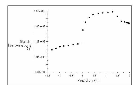
Temperature Distribution Graph for Tuyere Burner, Lid-off. 1300°C heating results from Fluent
