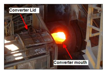
Figure 8.2: Peirce-Smith Converter at Mt Isa Copper Smelter
