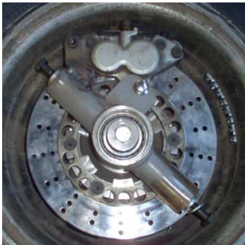
Figure 6.2: Final assembly of front brake system inside rim.
