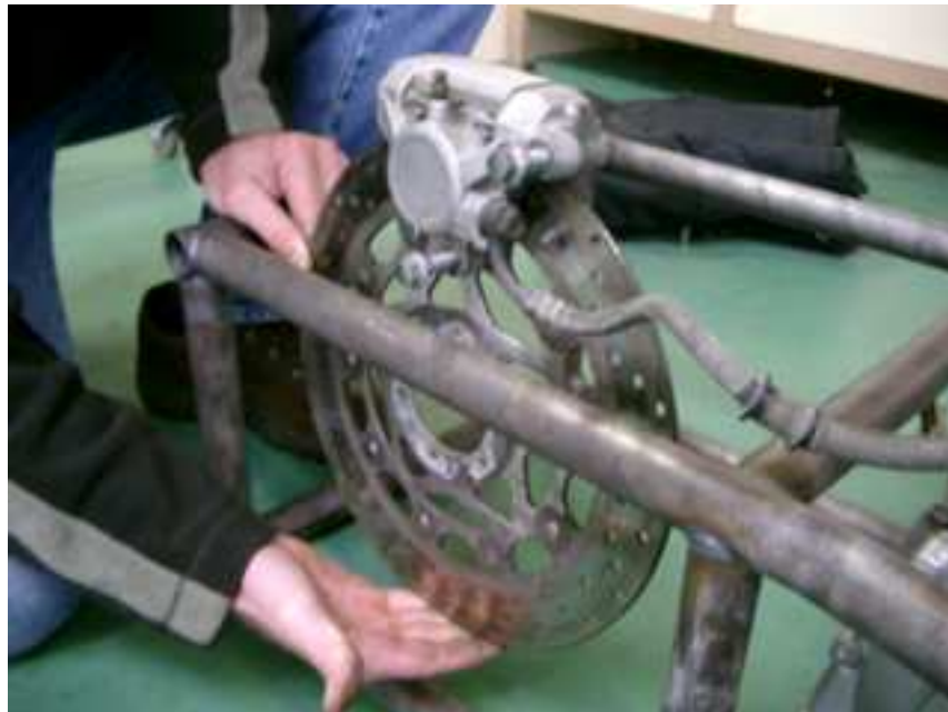
Figure 4.3: Positioning of potential rear brake assembly location.
