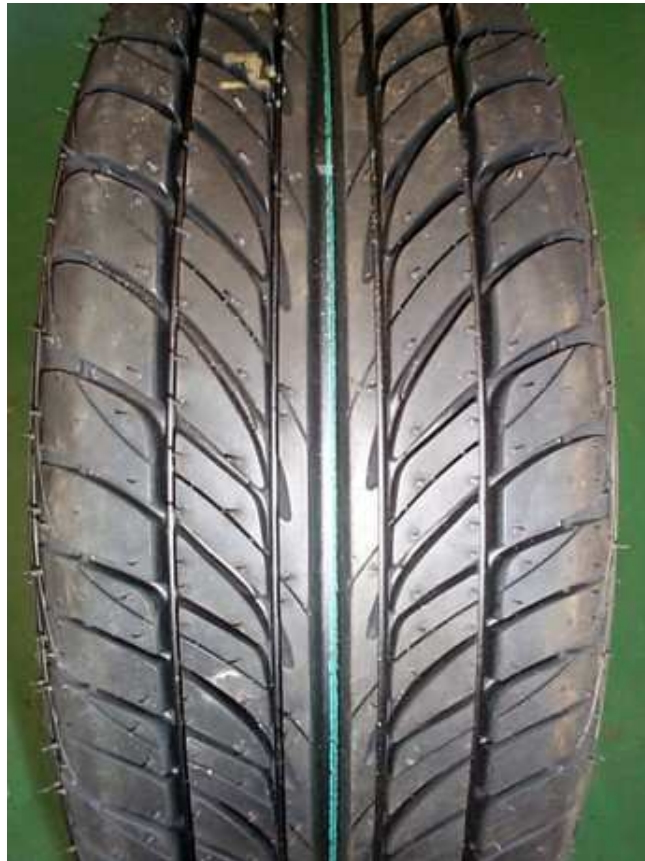
Figure 6.7: Tread pattern of the Falken ZE512 directional tyre purchased for the car.
