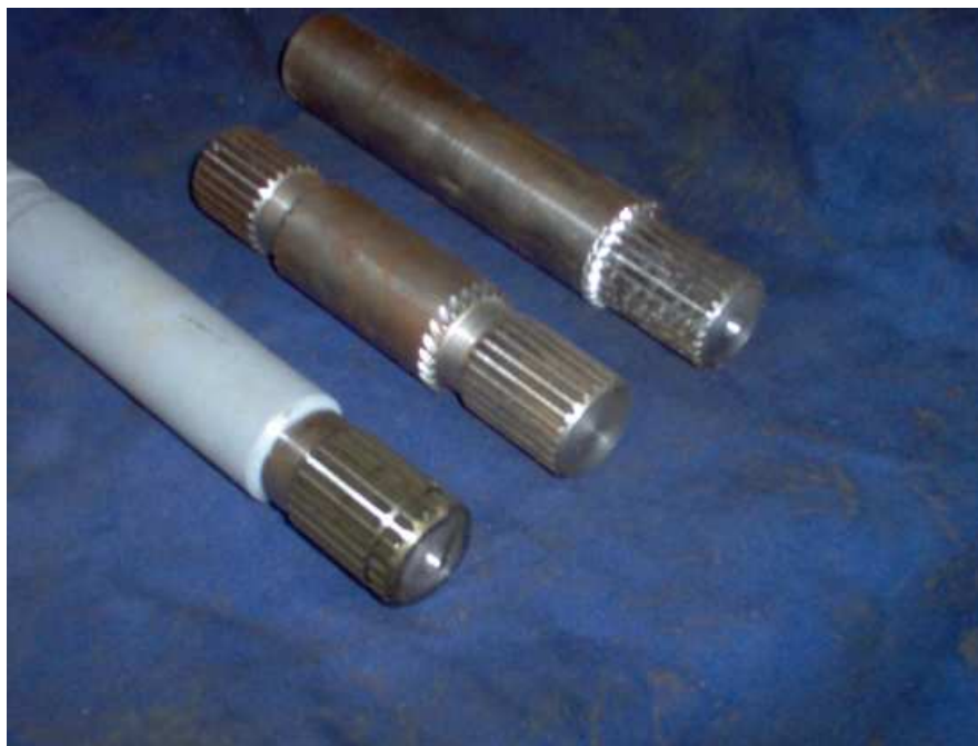
Figure 5.1: Trial splines at top with the final shorted half shaft below.
