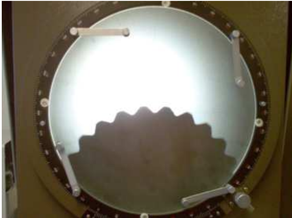
Figure 4.4: View of tooth profile under profile projector.
