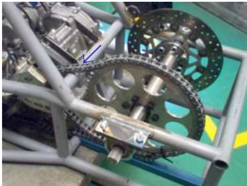
Figure 4.2: Drivetrain assembly with arrow indicating the point of chain contact with frame.
