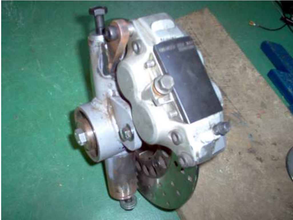
Figure 6.3: Front Caliper mounting arrangement.
