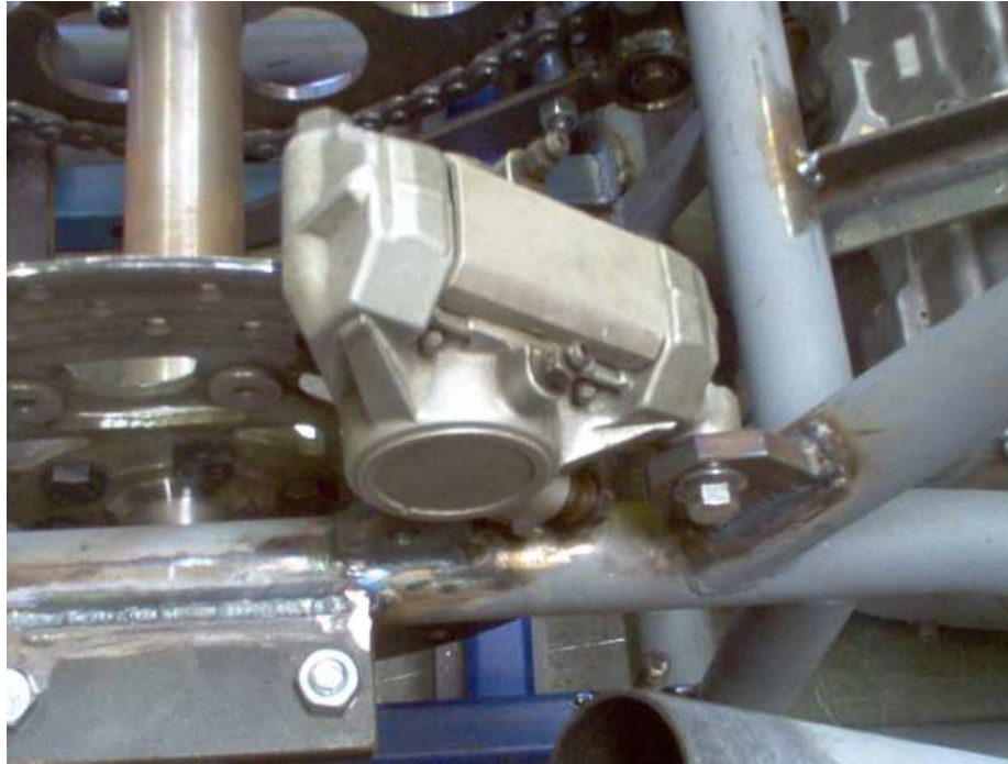
Figure 6.4: Rear Caliper mounting arrangement.
