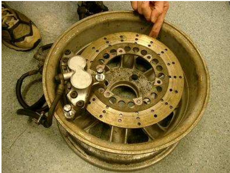
Figure 6.1: Positioning front brake assembly inside 13 inch rim.
