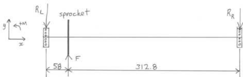
Figure 4.17: Free Body Diagram of modified centre shaft.
