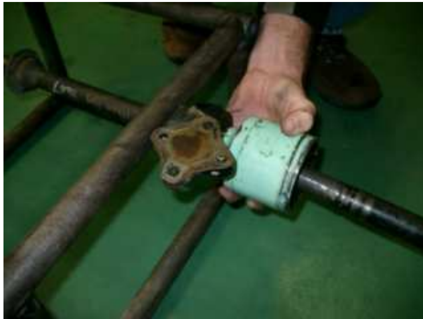
Figure 4.1: Positioning of CV joint and bearing housing in spaceframe.
