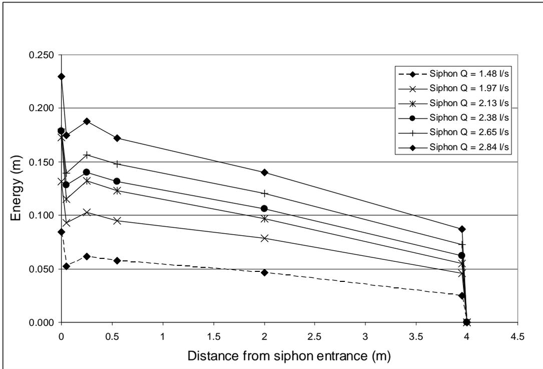
Figure 13: Energy Grade Lines (EGL) for the dynamic tests.
