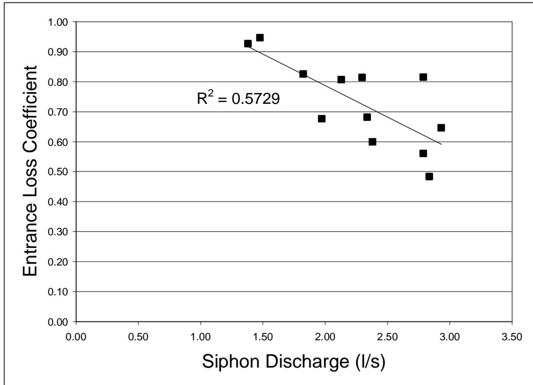
Figure 15: Entrance loss coefficient Vs siphon discharge.
