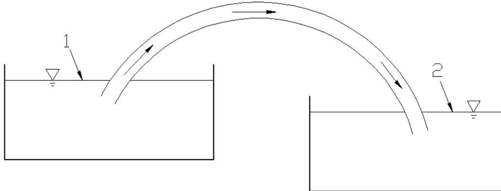
Figure 1: Simple diagram of a siphon operating with a submerged exit.
