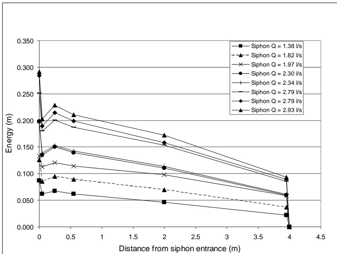
Figure 12: Energy Grade Lines (EGL) for the static tests.
