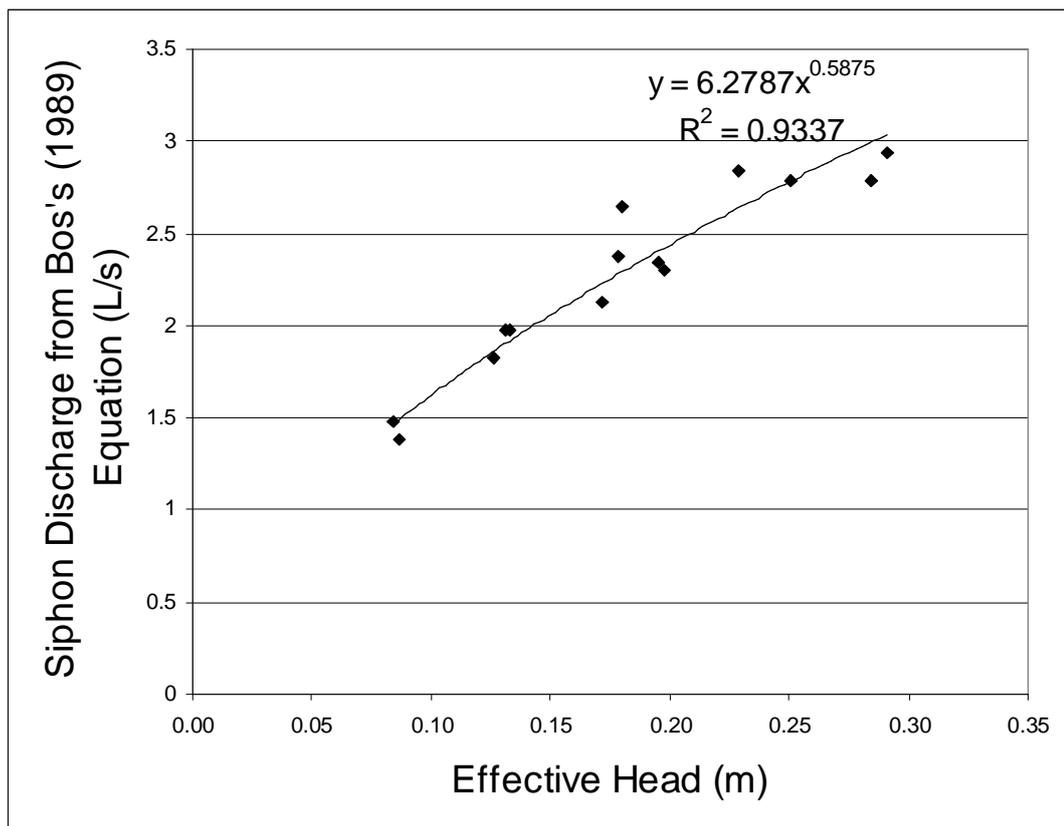
Figure 18: Using a power function to fit measured discharges with the effective head.
