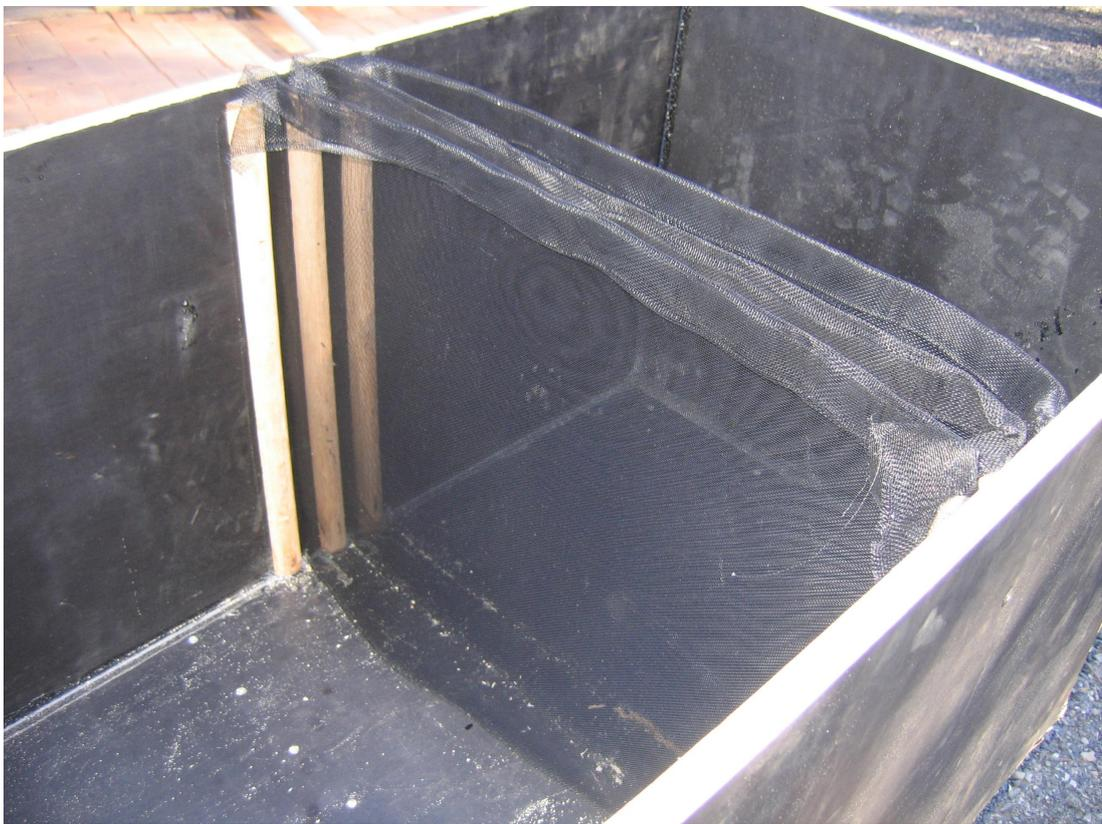
Figure 5: Metal flyscreen energy dissipators.
