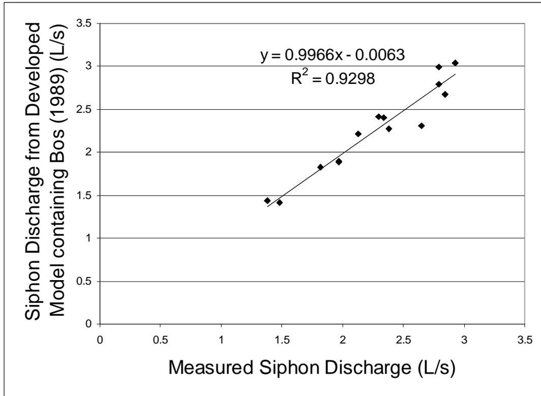
Figure 19: Developed model siphon discharge against measured siphon discharge.
