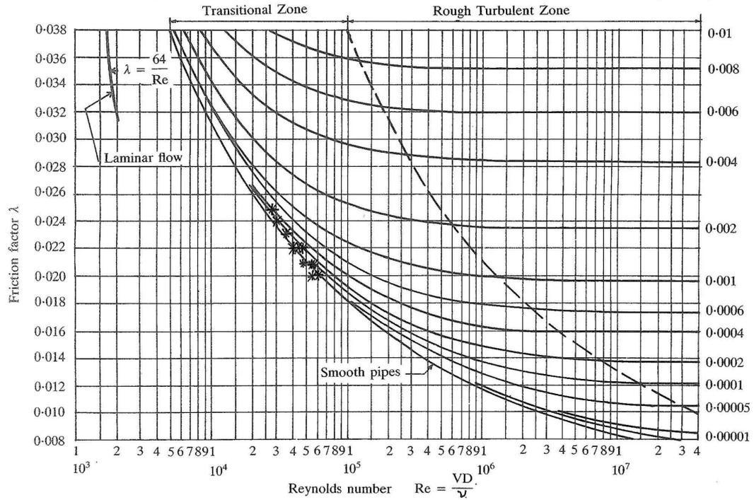
Figure 17: Moody Diagram with the Blasius friction factor plotted against Reynolds Number. (Nalluri & Featherstone 2001).
