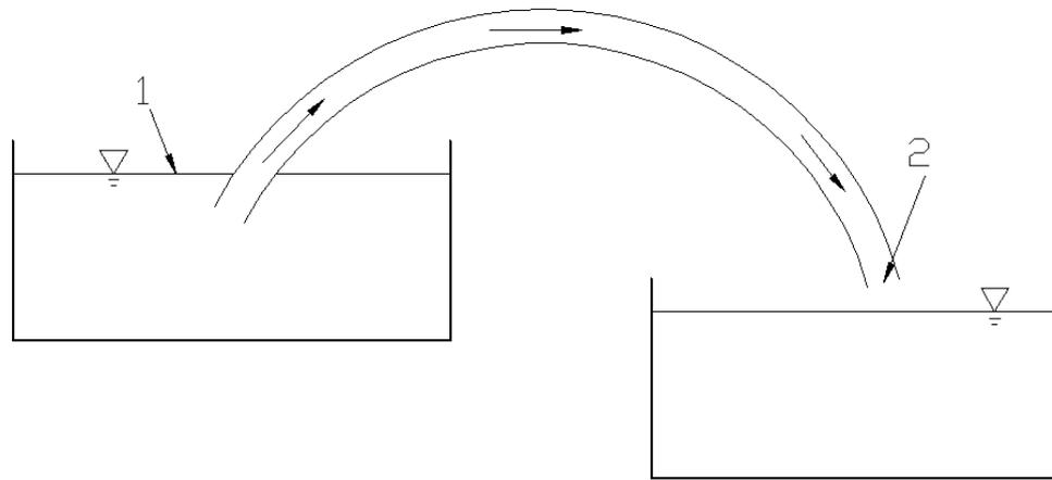
Figure 2: Simple diagram of a siphon operating with an unsubmerged exit.
