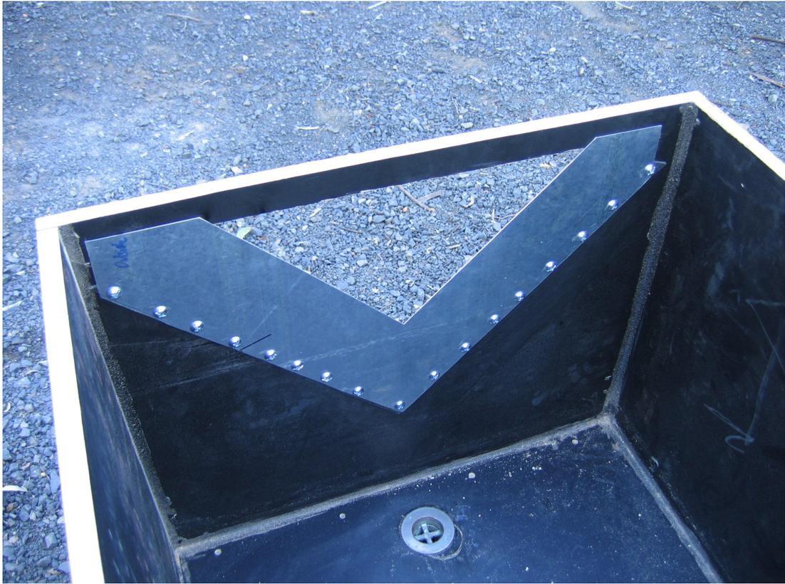
Figure 6: Small vee-notch weir and plug hole.
