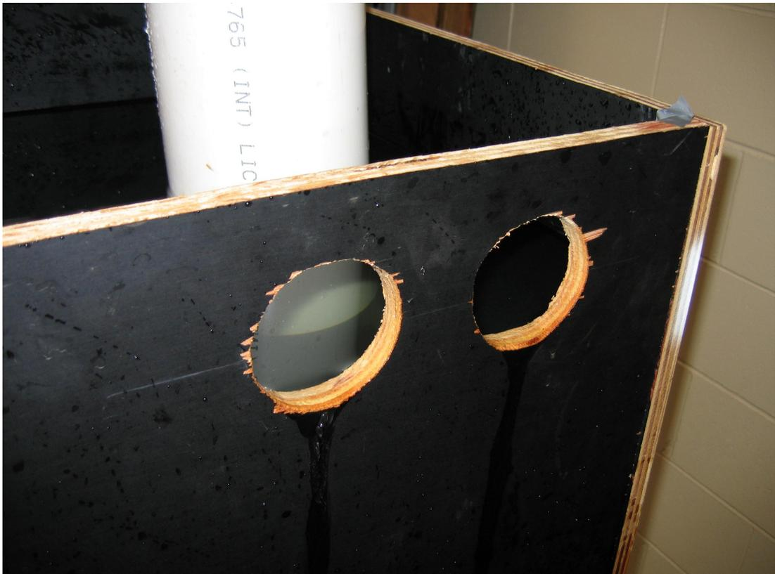
Figure 4: Holes in the side wall to maintain a constant water level in the channel while static tests were undertaken.
