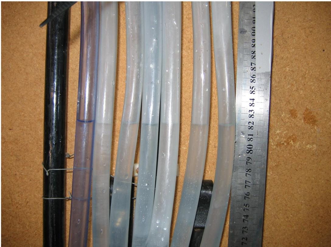
Figure 8: Manometer board with no discharge through the siphon.
