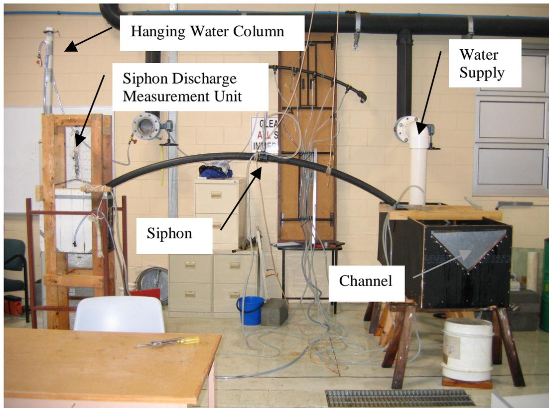
Figure 10: The experimental setup, with the siphon discharge unit on the left and the main channel on the right.
