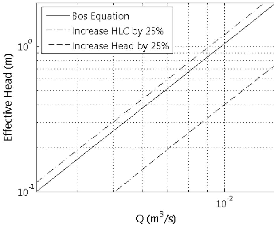
Figure 3: The effect of a 25% increase in the combined entrance and exit loss coefficient and diameter.
