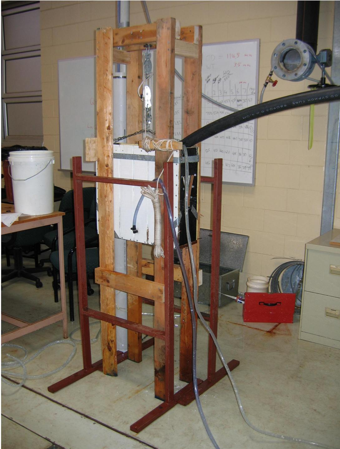
Figure 7: Siphon discharge unit and supporting structure.
