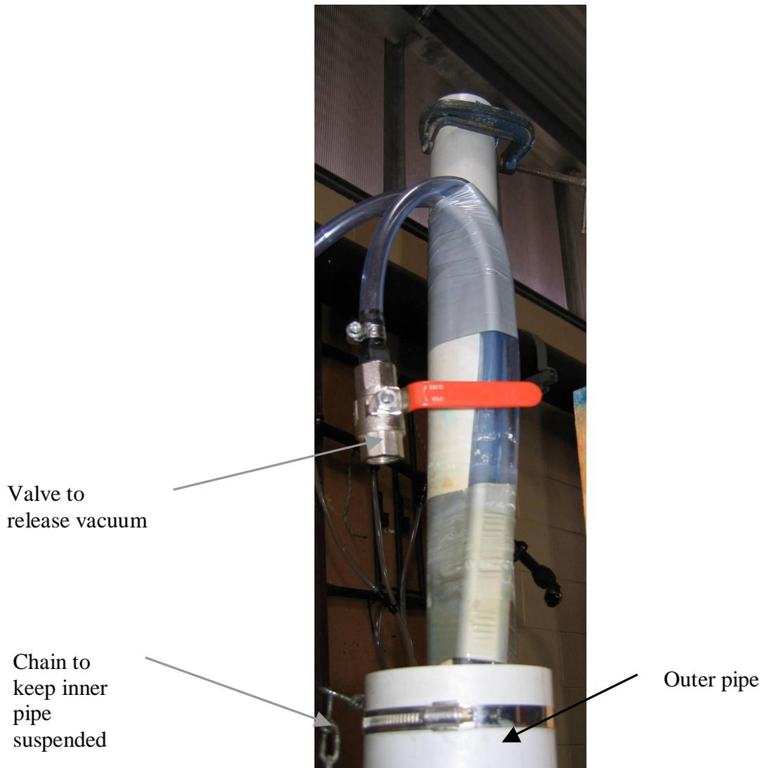
Figure 9: Top of the hanging water column.
