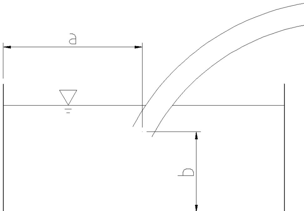
Figure 11: Diagram displaying distances of siphon entrance from channel walls.
