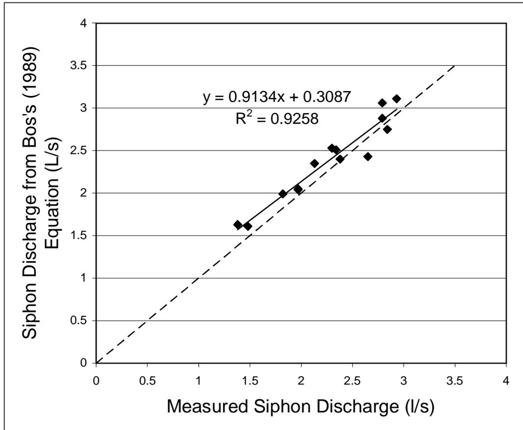
Figure 16: Comparison of measured siphon discharge to that obtained from the Bos (1989) Equation.
