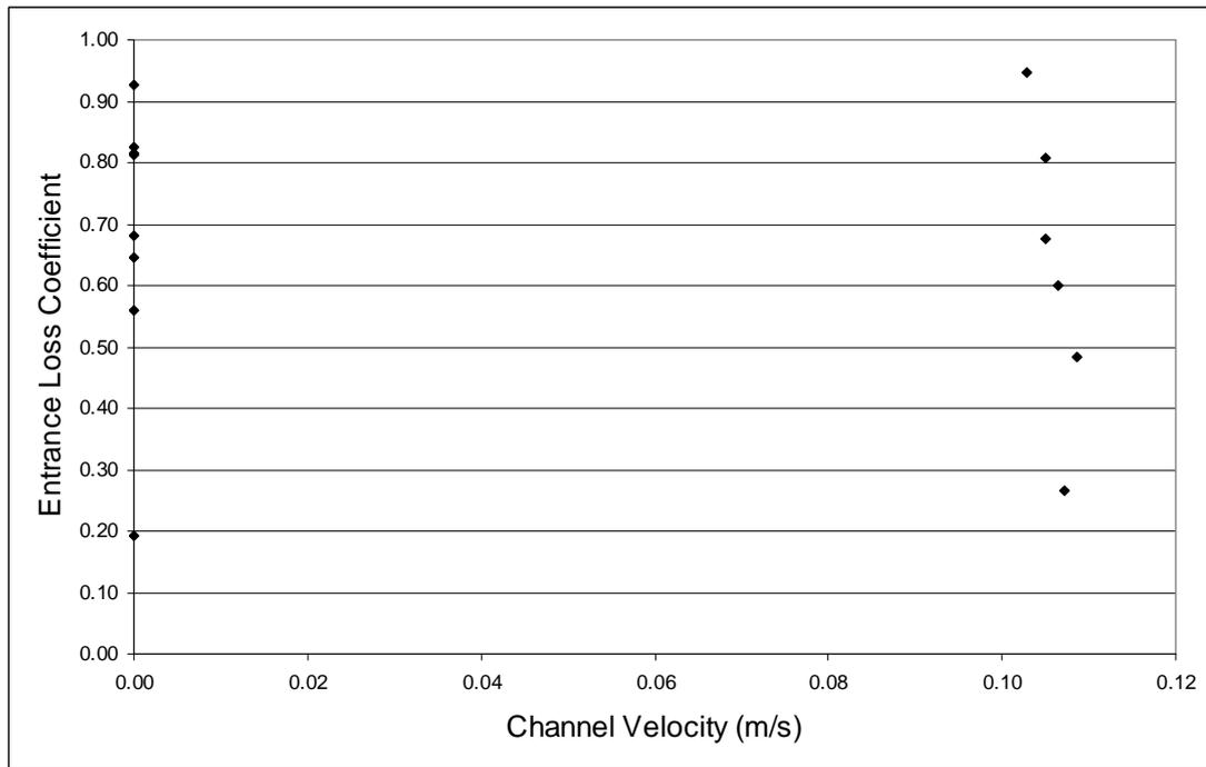
Figure 14: Entrance loss coefficient Vs channel velocity.
