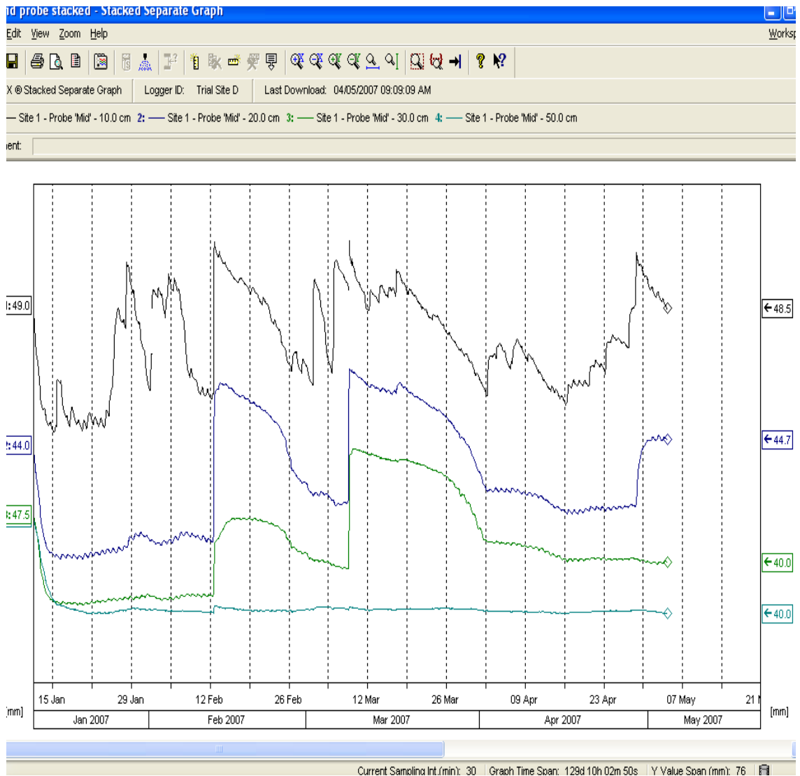
Figure 4.15 Stacked Enviroscan data from probe initially positioned in the ground with medium crop cover
