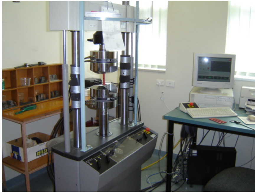
Figure 3.10 – Tensile Machine, with out puts read by the computer
