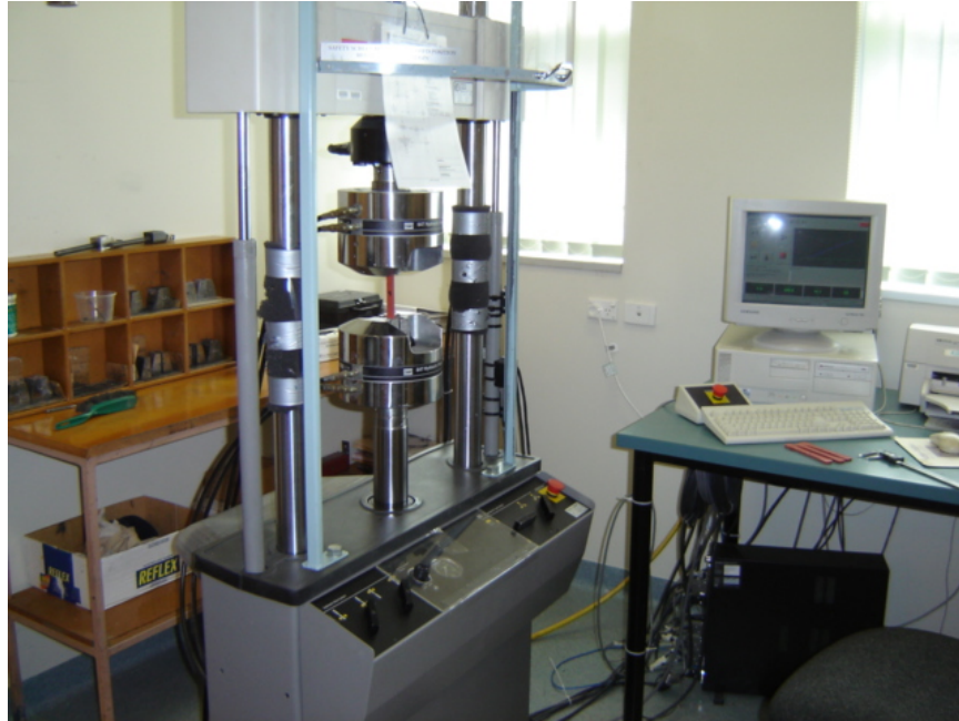
Figure 2.2 Tensile testing machine loaded with a specimen, with computer
