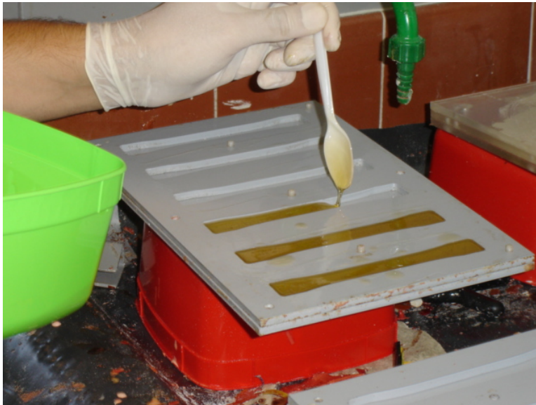
Figure 3.3 – Pouring of mixed materials into mould
