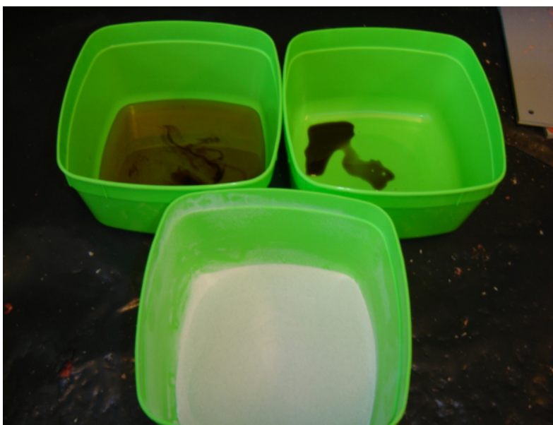
Figure 3.2 – The three materials used in study; Resin, catalyst and Filler
