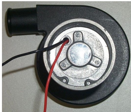
Figure 42: Motor view of a Centrifugal Blower
