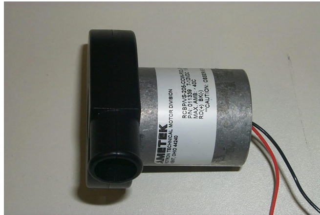
Figure 40: Side view of a centrifugal blower
