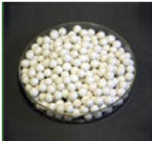
Figure 12: Activated alumina bead
