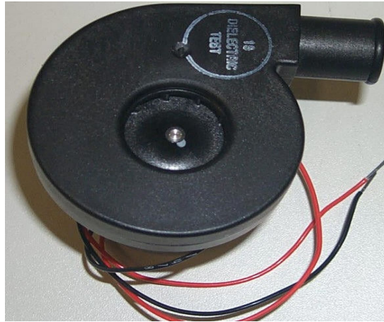
Figure 41: Inlet view of a centrifugal blower
