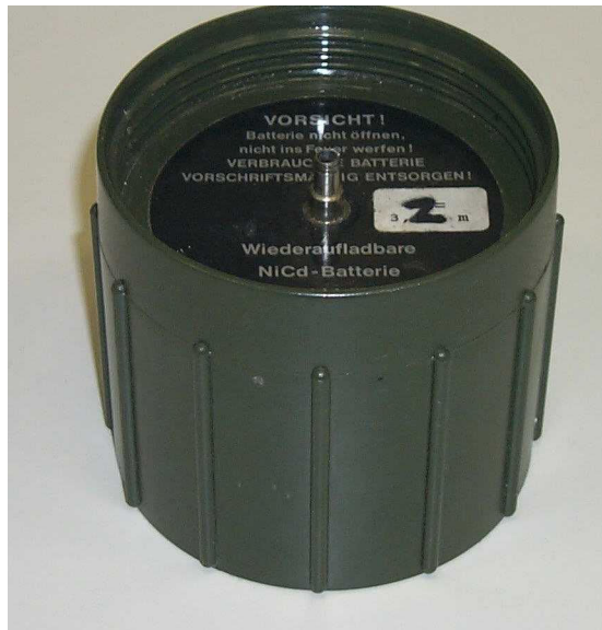
Figure 8: An existing re-charger battery
