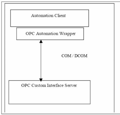
Figure 11: Interfacing to OPC servers
