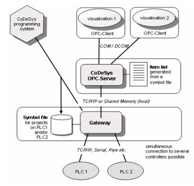
Figure 10: Architecture of the CoDeSys OPC server
