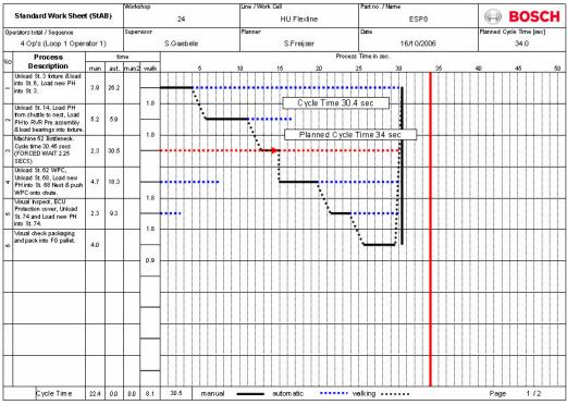
Figure 3: line balancing worksheet
