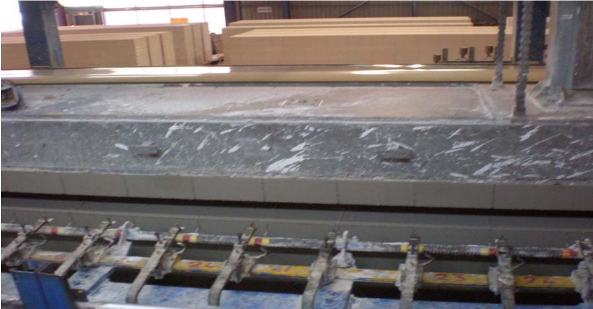
Figure 3.8: Cutting into 250 pieces of ALC blocks
