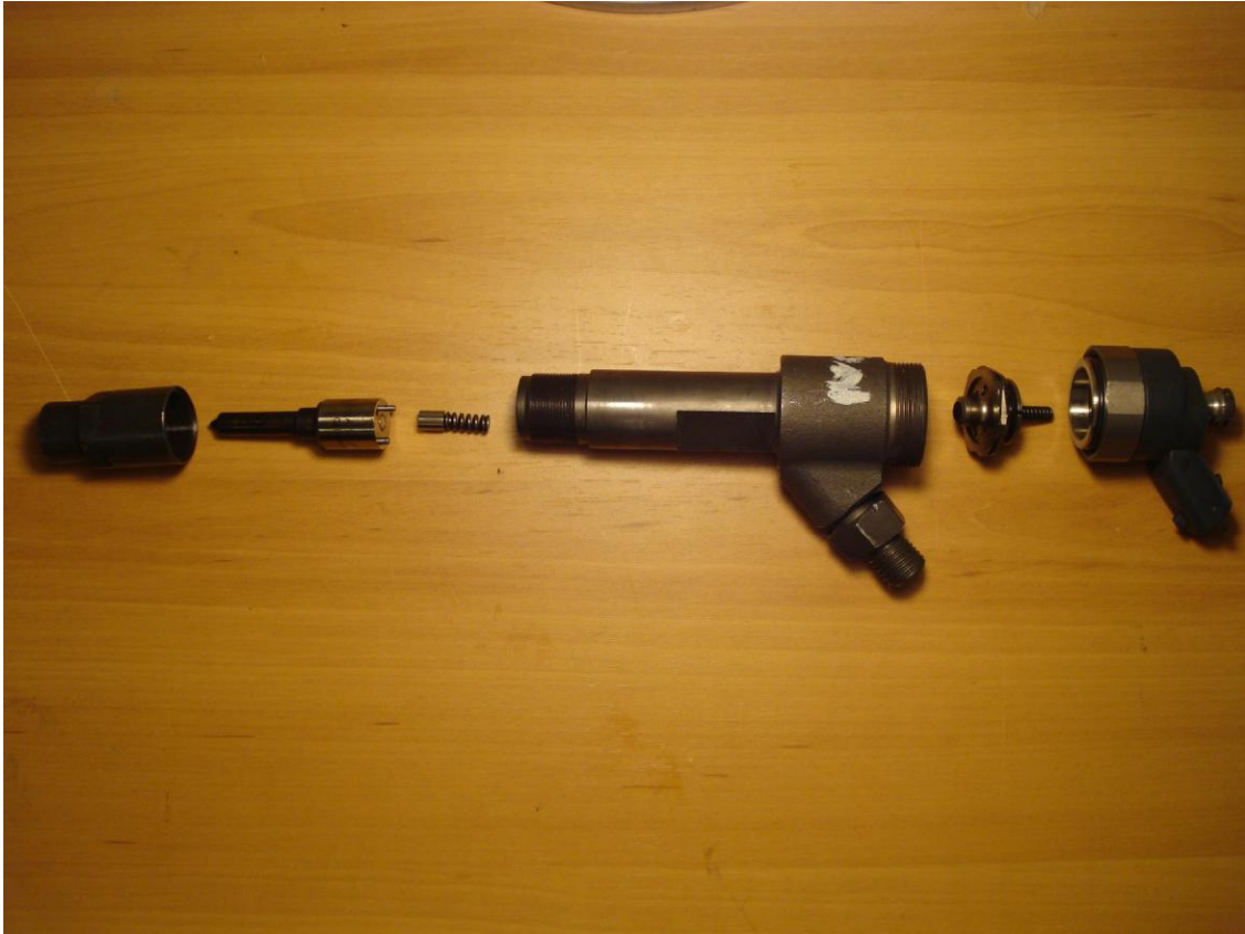
Figure 22 – Bosch Injector Exploded View
