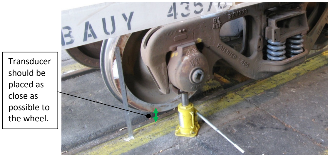
Figure 7-7 Locating the transducer
