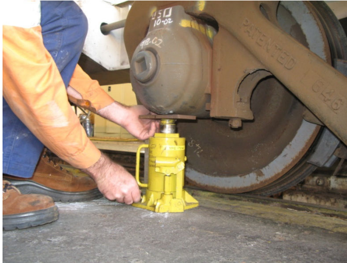
Figure 5-1 Hydraulic cylinder are viable for the twist test
