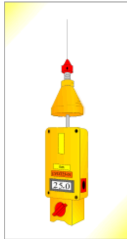
Figure 4-3 LVDT mounting used on Hydra-Capsule systems (Hydra-capsule 2007)
