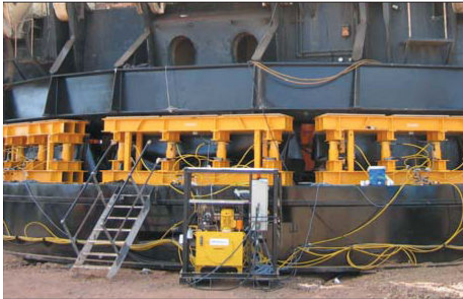
Figure 4-1 Dragline lifting with the Enerpac SLS (Enerpac catalogue)
