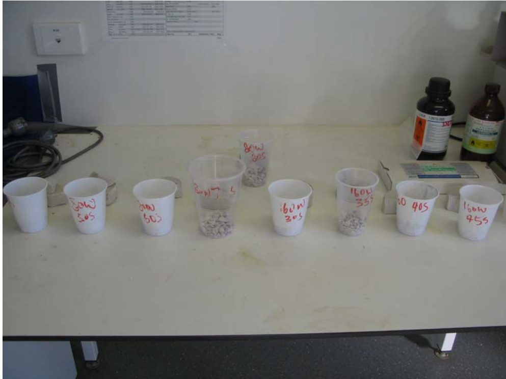
Figure 2.3: Crushed VE/FLYYASH (33%) by hammering
