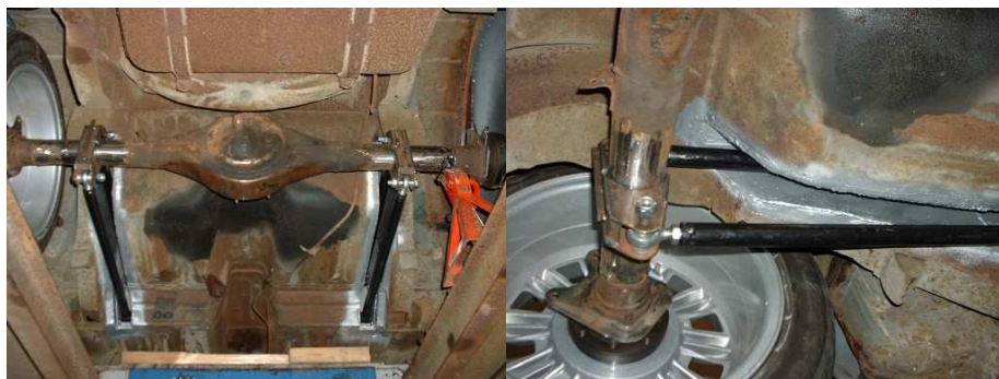
Figure 4.10: Parallel four link arrangement
