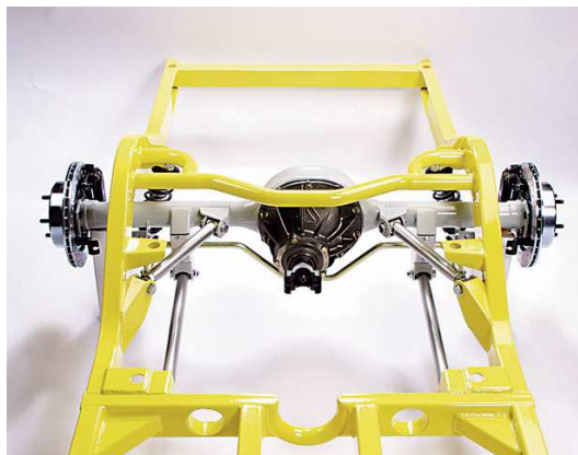
Figure 3.7: Converging four link
