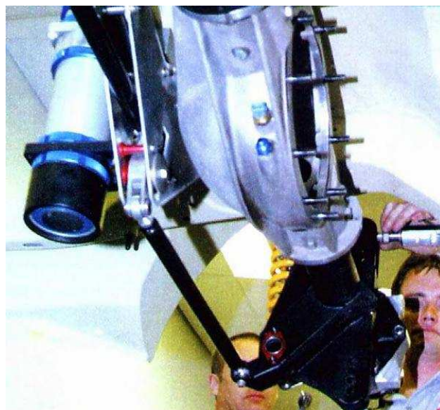
Figure 4.12: Adjustable watts linkage
