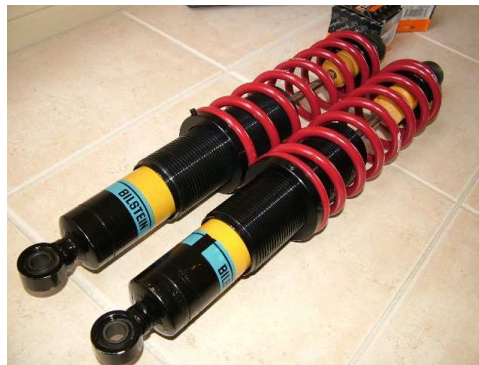
Figure 4.4: Coilover shock absorber assembly
