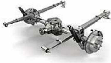
Figure 1.6: Hotchkiss rear axle
