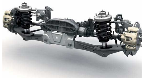
Figure 3.2: Independent rear suspension
