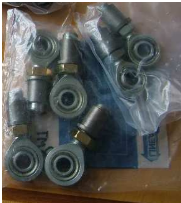
Figure C.13: Items 19 & 20; 3/8 Male Rod ends supplied with end plugs to weld into link bars and lock nuts
