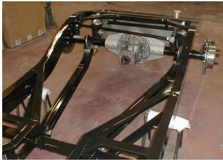
Figure 4.8: Truck arm configuration http://www.psrstreetrods.com/rear_suspension.htm
