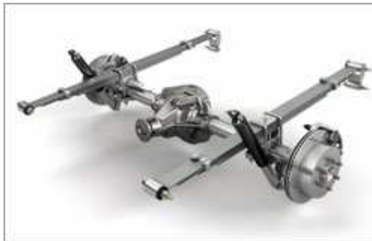
Figure 4.1: Leaf sprung Hotchkiss axle
