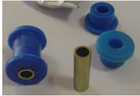
Figure C.11: Item 10; Escort lower control arm bushes
