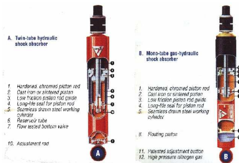
Figure 8.5: Single tube and double tube dampers
