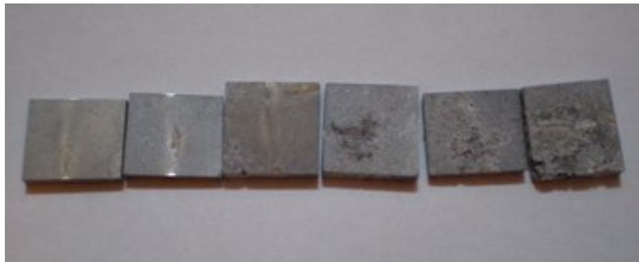
Figure 19: The static test specimens after 1, 2, 5, 10, 15, 20 days from left to right.
