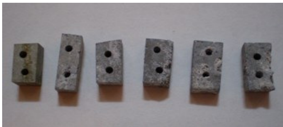
Figure 20: The dynamic test specimens after 1, 2, 5, 10, 15, 20 days from left to right.
