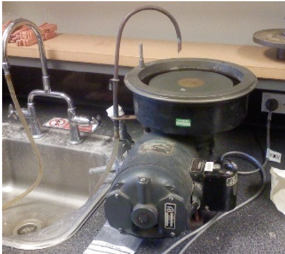
Figure 8: The grinding apparatus used for the sanding the test specimens.
