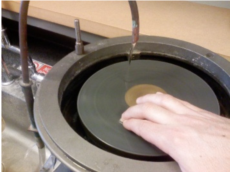
Figure 9: The grinding apparatus in use with a constant flow of water as a cleaning and cooling fluid.
