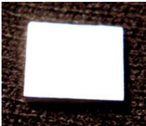
Figure 10: Fully polished static test specimen.
