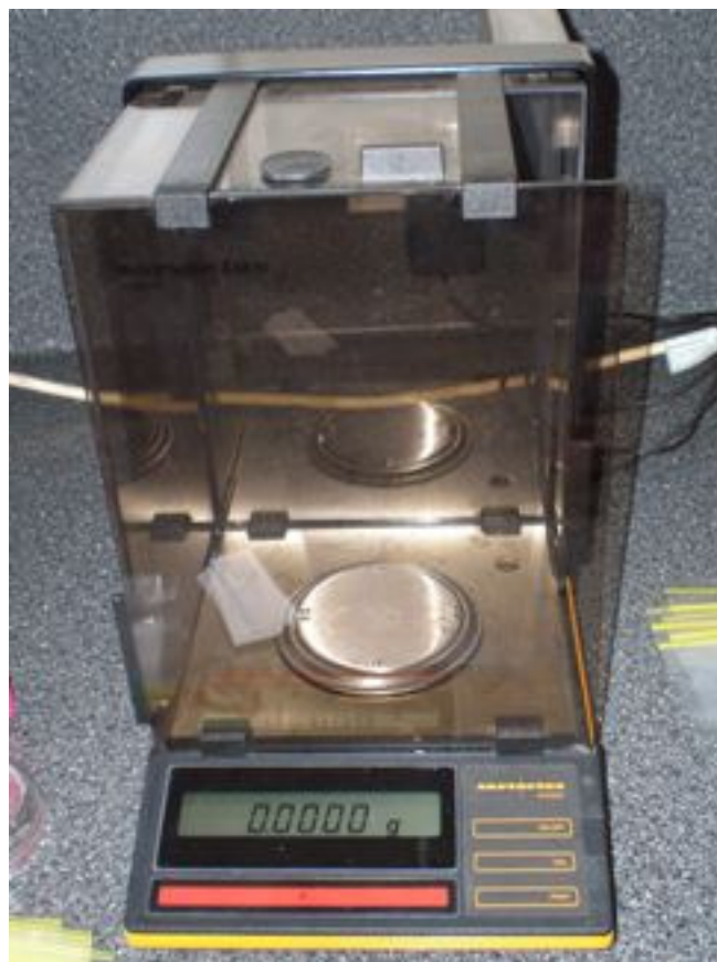
Figure 13: The highly accurate scales used for weighing each test specimen.
