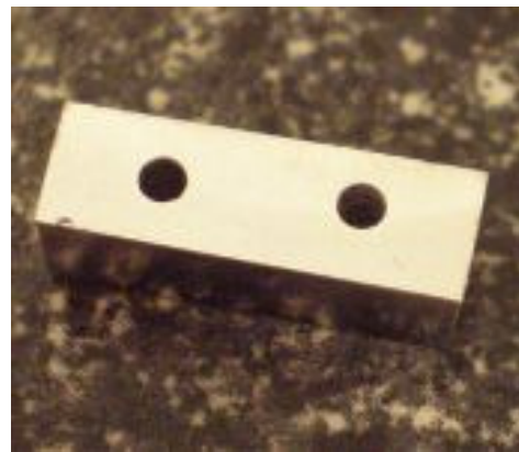
Figure 11: Fully polished dynamic test specimen.
