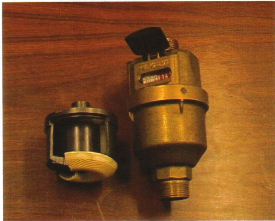
Figure 2.2 Positive Displacement Meter (Ipswich Water, 2002)
