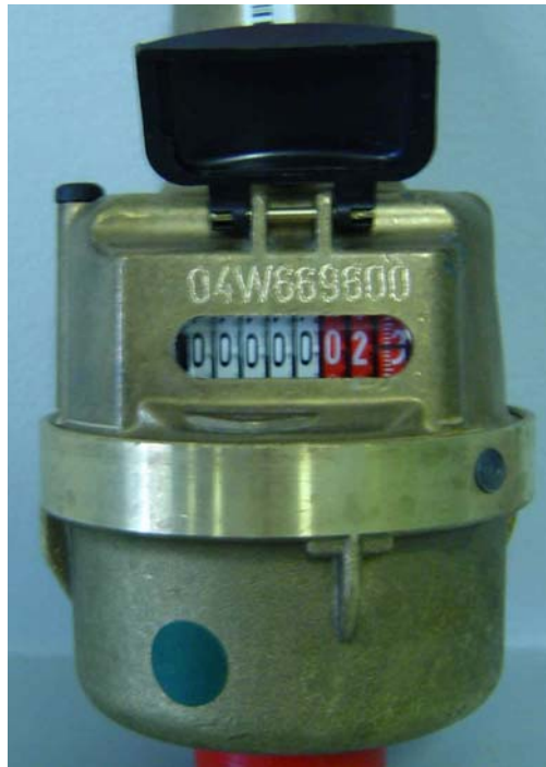
Figure 4.1 Engraving of serial number on water meter
