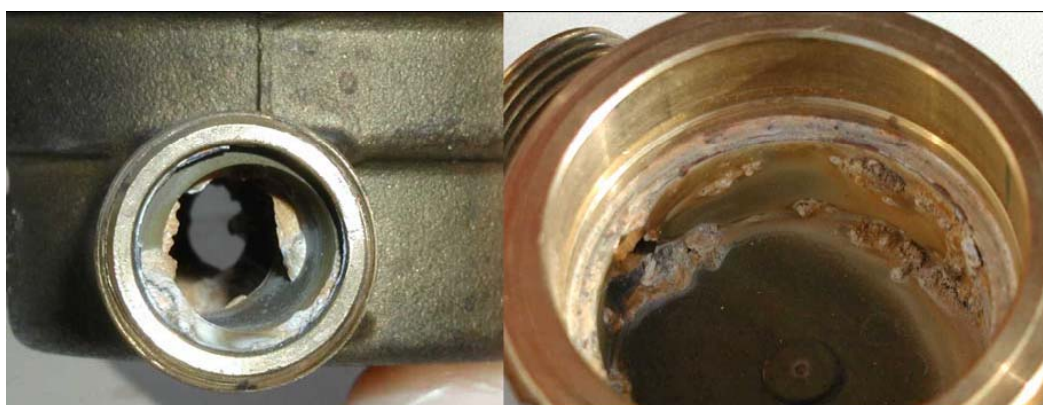
Figure 2.6 Limescale built-up in the inside of a single jet water meter housing (Arregui, 2005).
