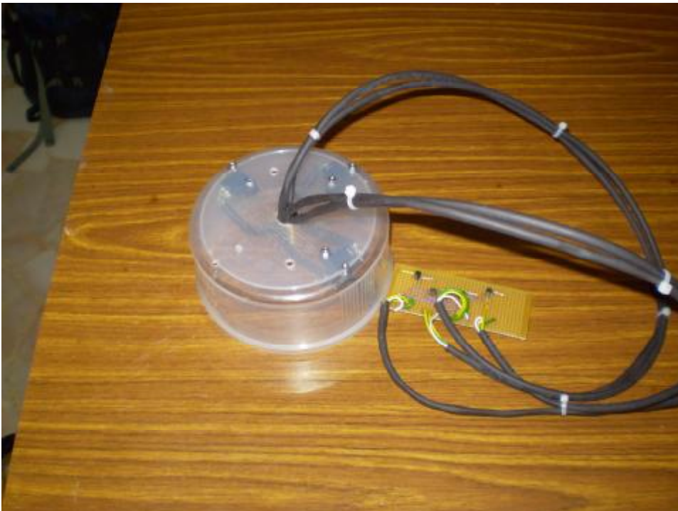
Figure 4.4: Photo of the EE-SX671 sensors and circuit
