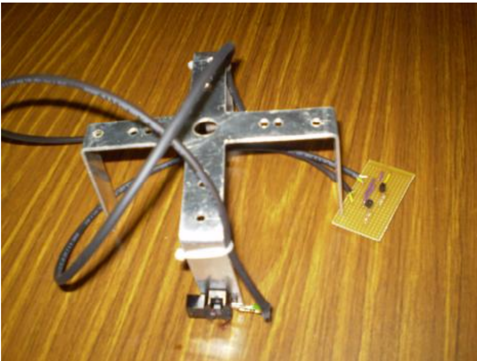
Figure 4.8: Photo of the actual PM2-LH10 sensors and the structure
